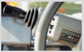
The new Powershift gearbox with electronic gear selector optimises cycle times.
