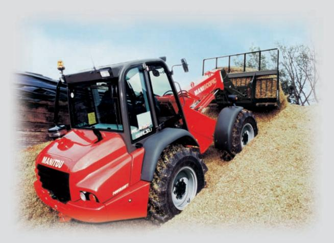
The **"kick down - kick up"** button is not only situated at the end of the forward/reverse gear change control but now in addition is placed on the hydraulic joystick and thus it is possible to engage a lower gear and come back to the initial one by simply pressing a button without taking one's hand off the steering wheel.
