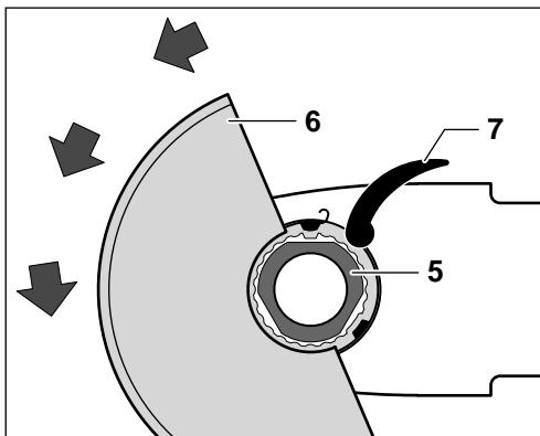
Press the protection guard onto the spindle collar until the collar of the protection guard faces against the flange of the machine and the encoding keys engage in the circular groove at the spindle collar.
