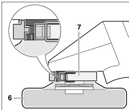
Rotate the protection guard **6** in clockwise direction to the required position (working position).
