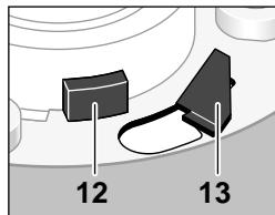
The grinding disc is clamped correctly when the 3 locking fixtures **13** and the 3 cams **12** project over the steel sheet hub of the disc. The grinding disc must be free to turn.
