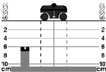
By pressing the “mode” button **8** during the measurement, the display of the measured results can be extended to 10 cm depth. This is recommended especially for concrete and other solid wall materials without air pockets (such as, for example, solid lime-sandstone blocks).
