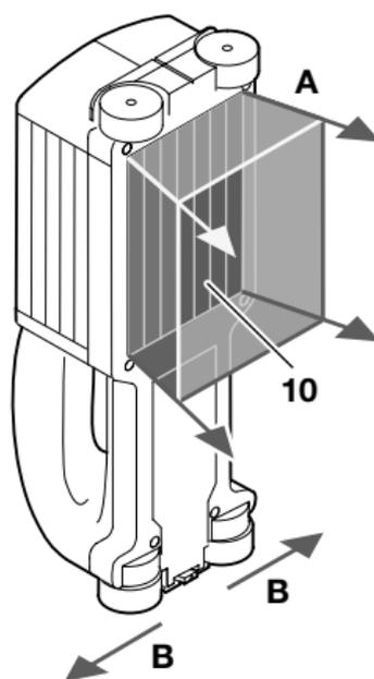
With the unit, the base material in the sensor area **10** in the measurement direction **A** is checked to the maximum measuring depth. Measurement is possible only during movement of the unit in the direction of travel **B** and for a distance of at least 8 cm.
