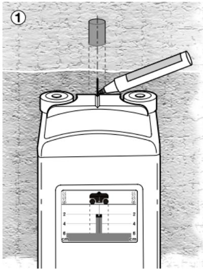
For the localisation of an object, move the unit in the direction of travel toward the object until the middle line **g** of the unit in the display is exactly over the middle line **h** of the object found. The object is then located exactly under the middle of the unit. With the help of the aligning aid **9**, the position of the object can be marked (Fig. ①).
