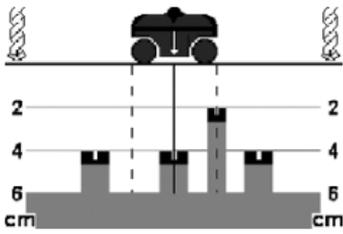
Example: In the illustration, three evenly spaced objects with an associated drilling depth of 4 cm are recognisable that, as a result of their position and depth, can be assumed to be reinforcing iron. The fourth object at 2 cm depth can be, for example, a mains cable.
