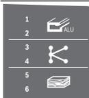
The table shows the recommended speed setting depending on the material to be worked: Aluminium, plastic, wood.
