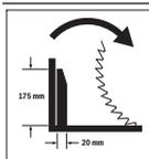
Direction of rotation of the spacer for the slide device for sawing wide mouldings.
