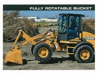
The Case quick coupler, which is standard on all compact E Series wheel loaders, allows for buckets to be completely rotated so that the top of the bucket runs parallel with the ground. This flexibility allows the operator to use the bucket to "pry" the machine out when caught up in difficult, sticky ground conditions. It's also useful for back-dragging material away from foundations, walls or other obstructions.
