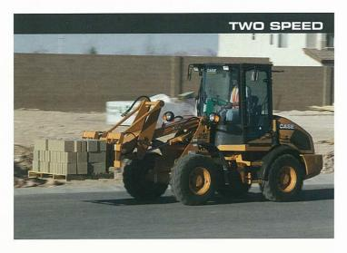
The E Series compact wheel loaders are equipped with an efficient hydrostatic transmission. This provides two speed operation up to 20 km/h on all models. A high speed option on the 121E, 221E and 321E offers a higher speed of 35 km/h.
