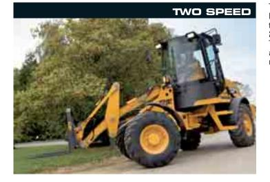
The E Series compact wheel loaders are equipped with an efficient hydrostatic transmission. This provides two speed operation up to 20 km/h on all models. A high speed option on the 121E, 221E and 321E offers a higher speed of 35 km/h. The front axle has a limited slip differential as standard equipment and the rear has limited slip as an option to ensure maximum machine traction when working in difficult ground conditions.
