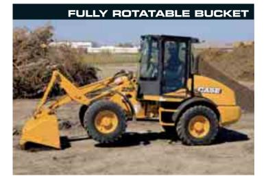
The Case quick coupler, which is standard on all compact E Series wheel loaders, allows for buckets to be completely rotated so that the top of the bucket runs parallel with the ground. This flexibility allows the operator to use the bucket to "pry" the machine out when caught up in difficult, sticky ground conditions. It's also useful for back-dragging material away from foundations, walls or other obstructions or lift front axle.
