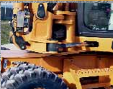
HYDRAULIC BOOM FOOT ARTICULATION FOR EASY DIGGING ALONGSIDE WALLS.
