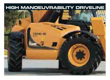
TX machines are incredibly agile, moving rapidly about the site thanks to a four-speed Powershift transmission and the easy to use three mode steering system. This combination of proven components ensures that there is no costly heat build-up in the transmission, even when travelling at high speeds on the road, where permitted.
