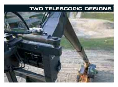
The TX range uses robust telescopic booms with inherent rigidity and strength to allow many hours of safe lifting. The TX130-30 and TX130-33 have a chain driven extension for the second boom section, while all larger machines use an internally mounted hydraulic twin cylinder to extend the boom. All models are equipped with safety valves on the lift, tilt and stabiliser cylinders, to prevent the boom dropping in the case of hose failure.
