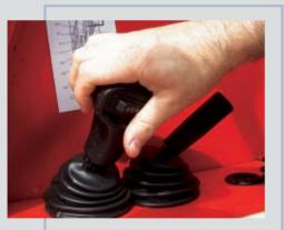
This new « boom control » joystick now integrates the « reversing shift » function : the driver can keep one hand on the steering wheel and one hand on this joystick to operate any movement. Time savings and much better driving position.
