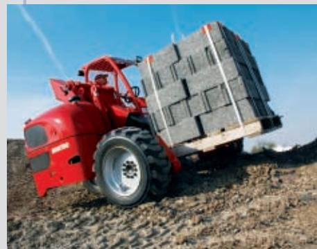
In addition to the 50 HP Perkins engine, the TMT 2520 SR XT has optimum torque: a drawbar pull 25% higher than that of the other models (2780 daN).
