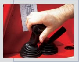
This new « boom control » joystick now integrates the « reversing shift » function : the driver can keep one hand on the steering wheel and one hand on this joystick to operate any movement. Time saving and much better driving position.
