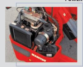
With a 50 HP Perkins engine connected to its 3 driving wheels, the TMT 2520 C has more power to be at ease on any kind of ground.
