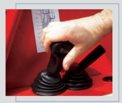
This new « boom control » joystick now integrates the « reversing shift » function : the driver can keep one hand on the steering wheel and one hand on this joystick to operate any movement. Time saving and much better driving position.
