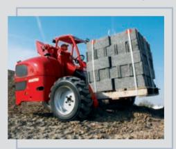
With a 50 HP Perkins engine connected to its 3 driving wheels, the TMT 2520 SR has more power to be at ease on any kind of ground.
