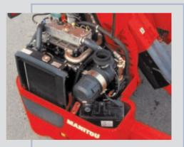
With a 50 HP Perkins engine connected to its 3 driving wheels, the TMT 2515 CR has more power to be at ease on any kind of ground.
