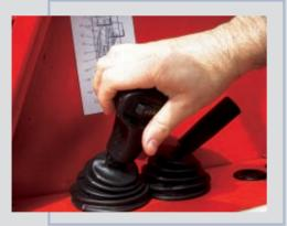
This new « boom control » joystick now integrates the « reversing shift » function : the driver can keep one hand on the steering wheel and one hand on this joystick to operate any movement. Time savings and much better driving position.
