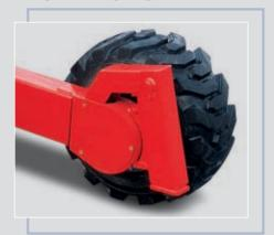
The 2 front stabilisers of the TMT 2020 S give more lifting capacity, especially when the boom is fully extended at maximum reach.
