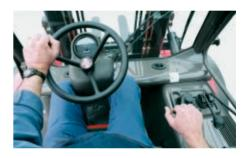
The see-through roof gives an optimum field of vision upwards.
