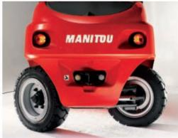
In the aisles, its compactness and very tight turning circle, thanks to a steerable axle with built-in piston, gives it incredible manoeuvrability.
