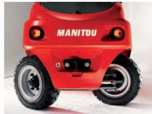
In the aisles, **its compactness and very tight turning circle,** thanks to a steerable axle with built-in piston, **gives it incredible manoeuvrability.**
