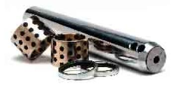
All boom pins (except the bucket pins) are extended maintenance system (EMS) chrome plated for increased hardness, with lubricated brass bushings fitted through the boom and dipper. Dust seals are double structured to prevent the ingress of dirt and dust on site.
