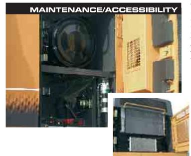
There are large, wide opening doors to both sides of the machine, making it easy for technicians to access the engine and hydraulic componentry. The CX800 is equipped with a hydraulically-driven cooling fan, which can be reversed on start-up to blow dust and debris away from the excavator's cooling pack.
