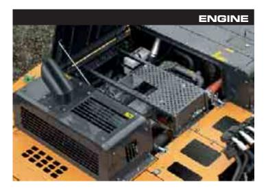
The Case CX800 is equipped with a proven Isuzu AH-6WG1X diesel engine, providing 495 hp (369 kW) of power at an unstressed 1800 rpm. With high pressure common rail fuel injection, this electronically-controlled engine meets the requirements of the EU directive 97/68/EC Tier 3A on engine emissions.
