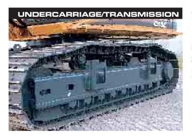
As the biggest machine in the Case range, the CX800 continues a long tradition of durable, highly productive mining and heavy earthmoving excavators. A modified X-style carbody is welded internally for added strength, and the turntable bearing hub extends down through the top plate of the carbody for additional structural integrity.
