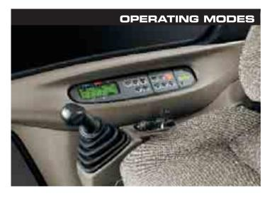
The CX800 enables the operator to have a choice on how the machine is operated. Simply choose the work mode that matches the machine output to the job application. Four operating modes are available.
