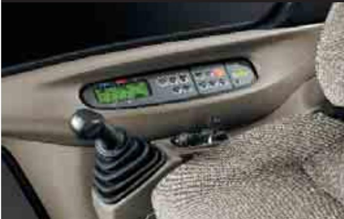
The CX800 enables the operator to have a choice on how the machine is operated. Simply choose the work mode that matches the machine output to the job application.
