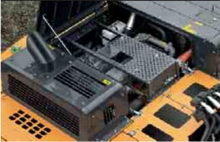
The Case CX800 is equipped with a proven Isuzu AH-6WG1X diesel engine, providing 495 hp (369 kW) of power at an unstressed 1800 rpm. With high pressure common rail fuel injection, this electronically-controlled engine meets the requirements of the EU directive 97/68/EC Tier 3A on engine emissions.
