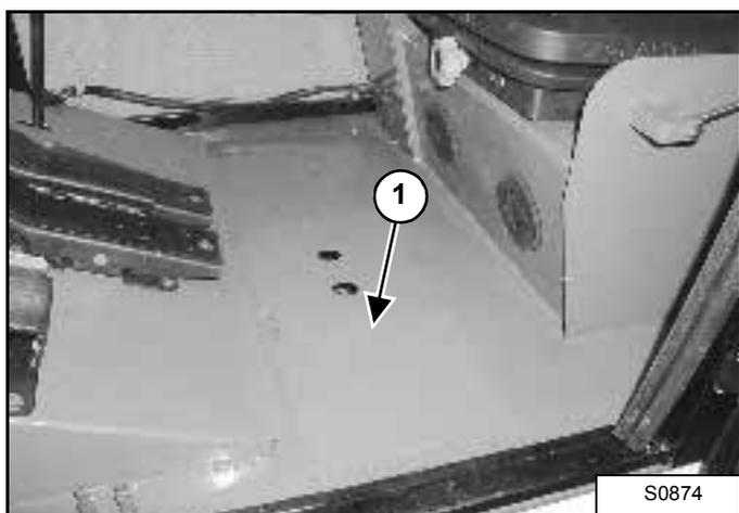
2. Remove the battery compartment cover (1).
