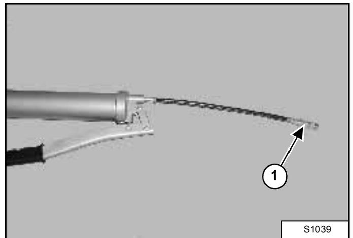
4. Remove the grease fitting adapter (1) from the end of a grease gun.
