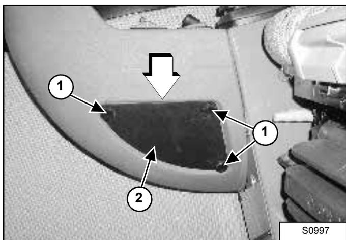
1. To check or replace the fuses in the right console, remove the three screws (1).
