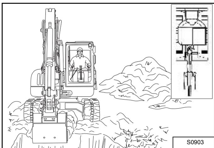
The boom offset allows the operator to dig close to buildings and other structures [Figure 89].
