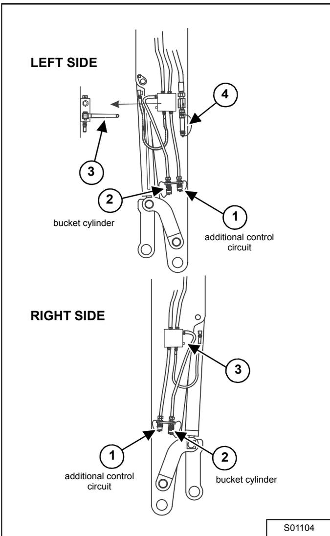
Retract the bucket cylinder piston rod completely.
