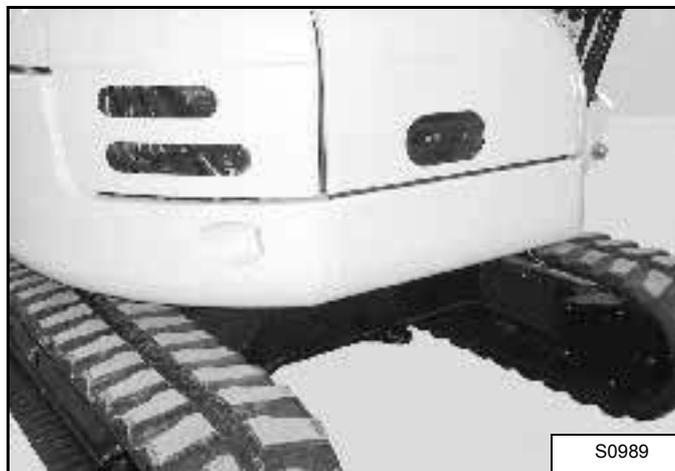
Rotate the upperstructure so the right side is positioned between the tracks [Figure 126]. Run the engine until it is at operating temperature. Stop the engine.
