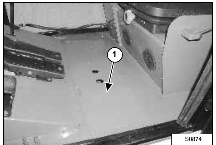
2. Remove the battery compartment cover (1).
