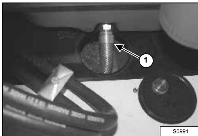
1. Install the drain hose (1) on the oil pan.
