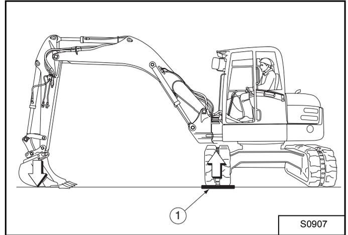
If one or both tracks have become stuck in soft or wet ground, raise one track at a time by turning the upperstructure and pushing the bucket against the ground [Figure 91].
