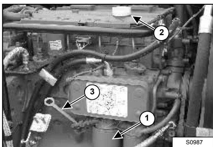
5. Remove the oil filter (1) and clean the filter housing surface.
