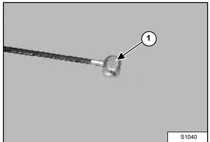
5. Install the track tensioning adapter (1) on the end of a grease gun.
