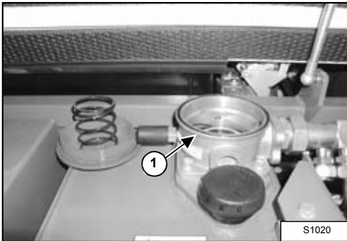
4. Inspect the O-ring (1). Replace if damaged.
