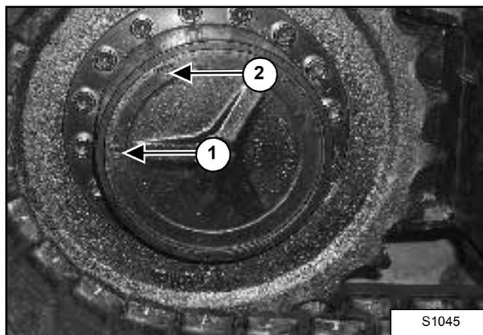
1. Put the machine on a level surface with the plugs positioned as shown (1 & 2).
