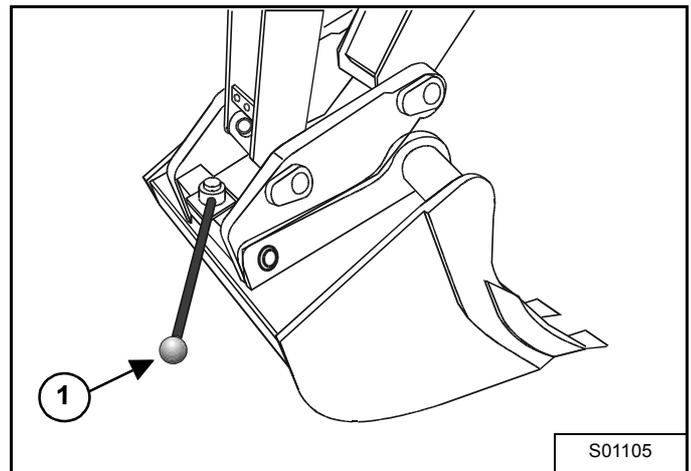
The quick-mount hitch is then opened with the control rod until the locking bolts are completely retracted.
