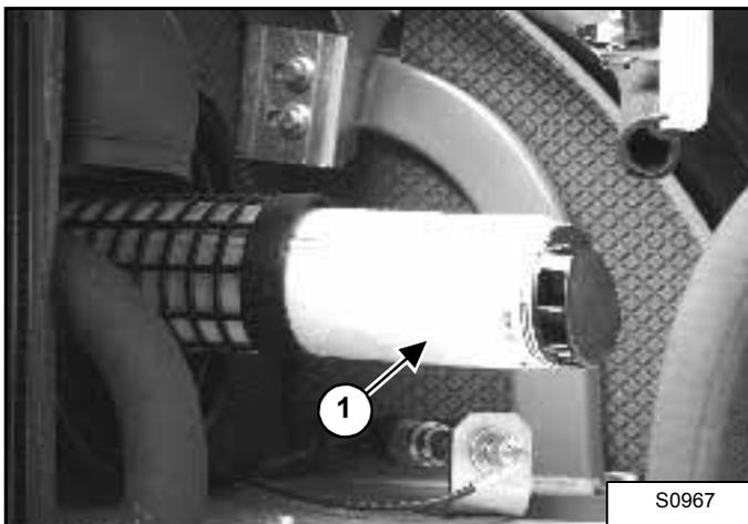
5. Install the new inner filter (1). Install the, outer filter and air cleaner cover.
