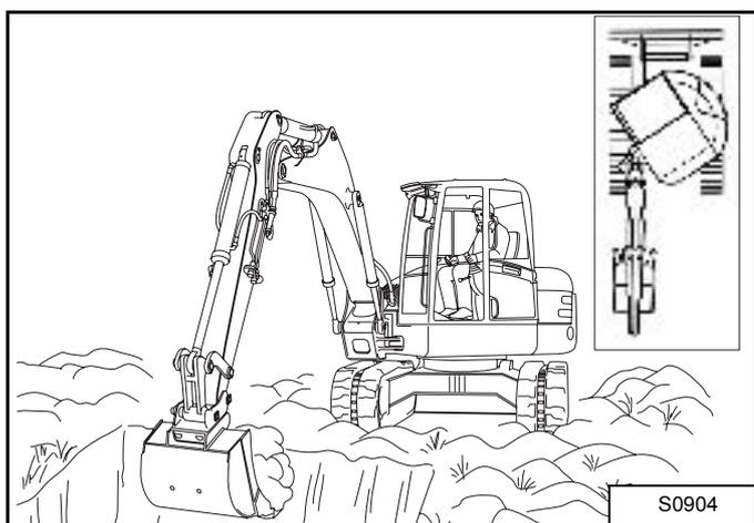
Swing the upperstructure, offset the boom to the right [Figure 86], centre [Figure 87], and left [Figure 88] to dig a square hole the width of the machine without repositioning the Excavator.
