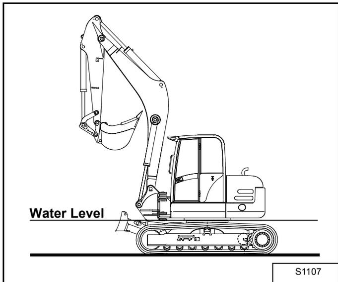
Do not operate or immerse the Excavator in water higher than the bottom of the swing circle **[Figure 98]**.
