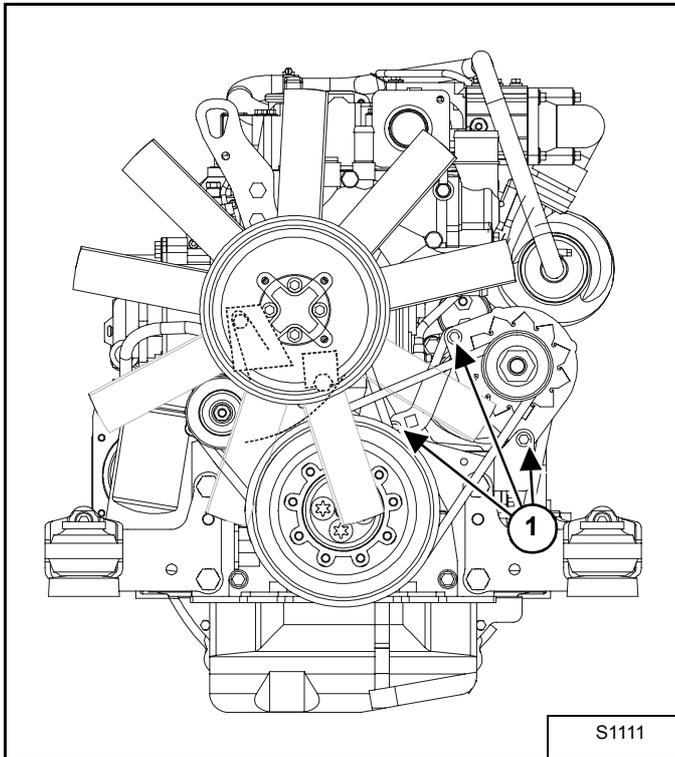
1. Loosen the three alternator bolts (1) [Figure 148] and rotate the alternator until the belt is correctly tensioned.
