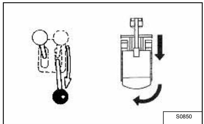
Pull the right steering lever backward to turn left while travelling backward [Figure 21].
