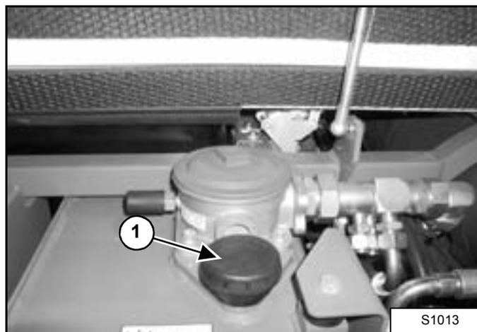
2. Clean the surface around the reservoir (breather) cap and remove the cap from the reservoir (1).
