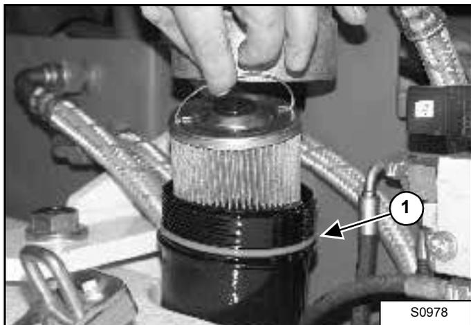
3. Install the filter in the housing [Figure 118].
