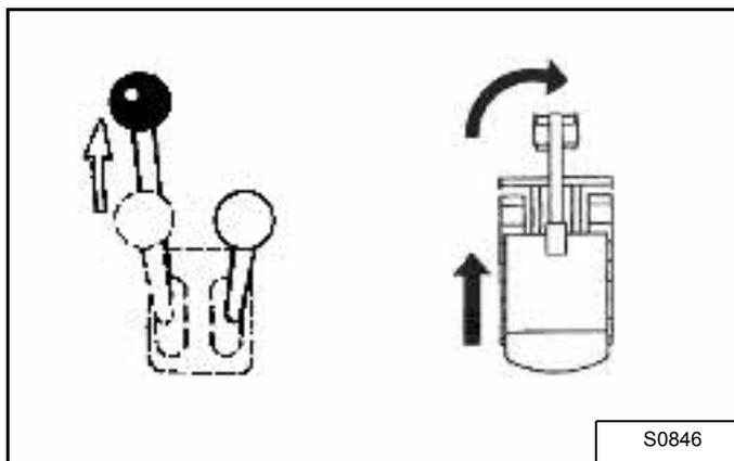
Push the left steering lever forward to turn right [Figure 17] while travelling forward.
