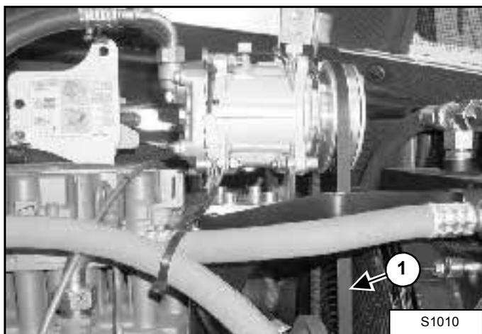
1. Check the air conditioning compressor belt deflection mid span of the belt between the crankshaft pulley and the compressor pulley (1).
