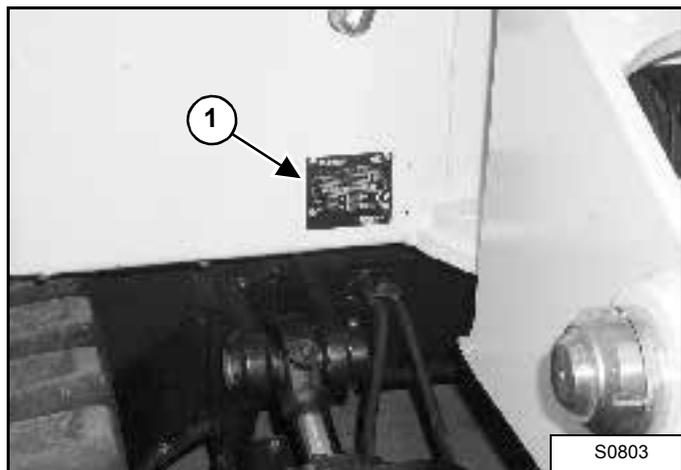
Excavator Serial Number The Excavator serial number plate (1) is located on the frame of the machine in the location shown [Figure 1].
