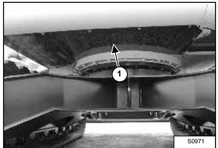
1. Remove the eleven bolts and washers of the cover plate (1) [Figure 110].
