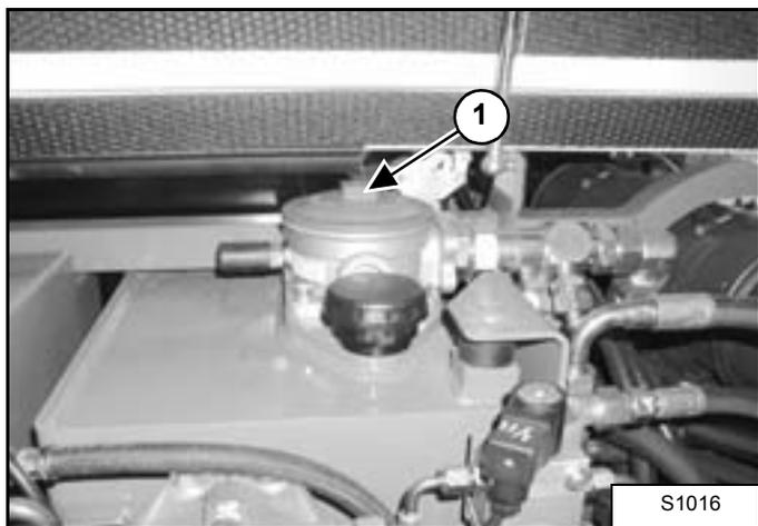
1. Remove the filter cover (1) and spring.
