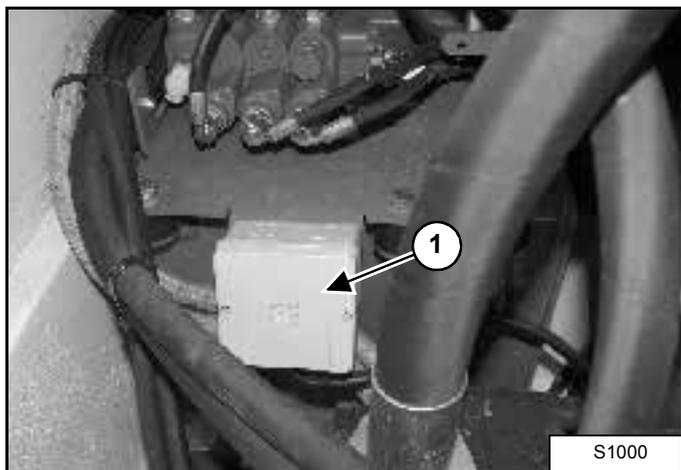
1. Remove the cover (1) for access to the fuses.
