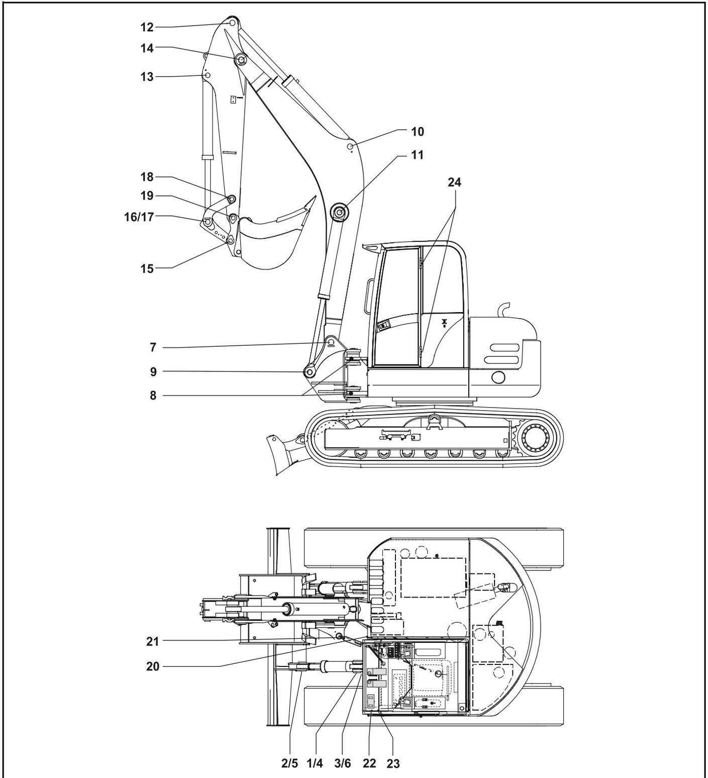
Lubricate the following locations on the Hydraulic Excavator EVERY 8-10 HOURS:
