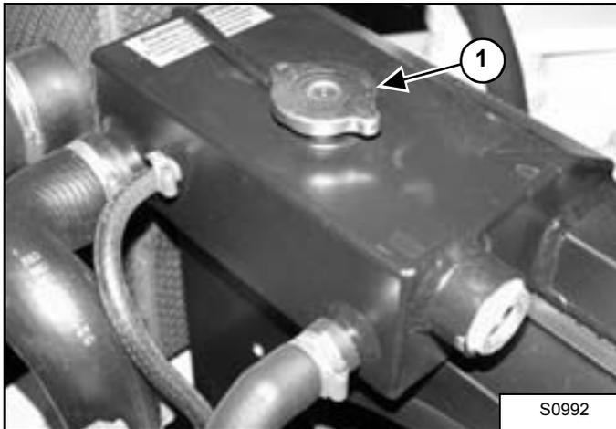
1. When the engine is cool, loosen and remove the radiator cap (1).
