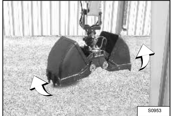
Move the right joystick to the right (2) [Figure 49] to open the clamshell [Figure 51].
