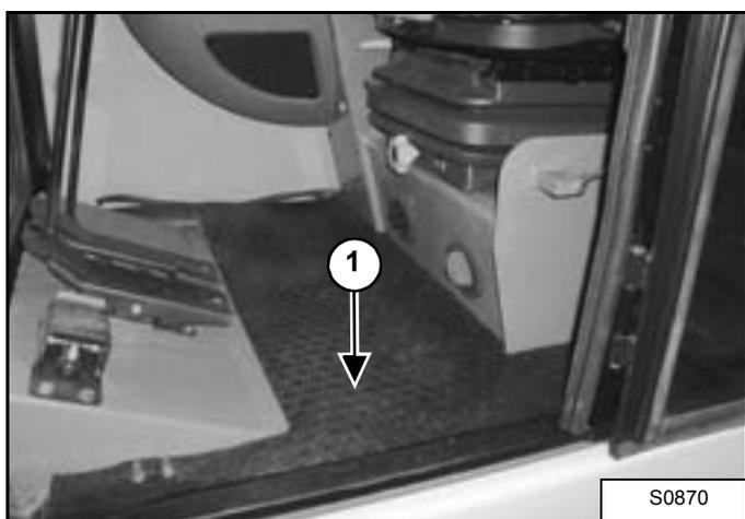
1. Pull up on and remove the floormat (1).
