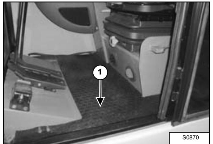
1. To check or replace fuses beside the battery, pull up on and remove the floor mat (1).
