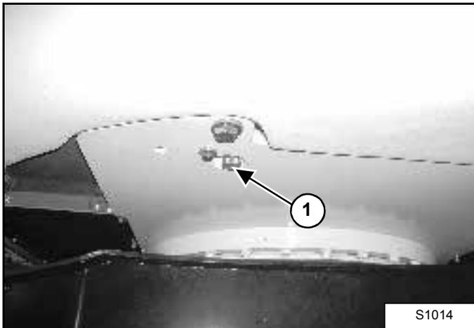
1. Remove the cap (1) from the hydraulic reservoir drain.
