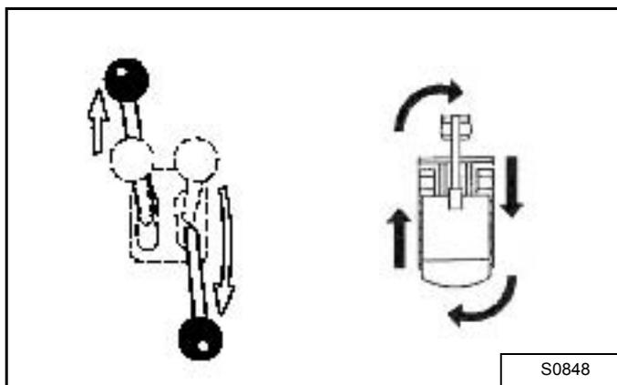
Push the left steering lever forward and pull the right steering lever backward [Figure 19].
