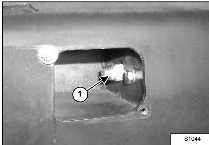
8. To release track tension, loosen the tensioner (1). Do not remove the tensioner.
