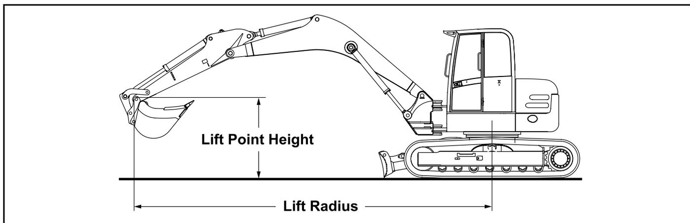
**Note:** Lift point is bucket hinge pin with standard bucket attached and bucket cylinder fully extended. Rated lift capacity over blade, blade down.
