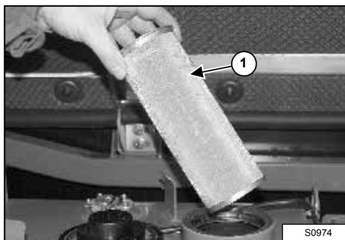
2. Check the condition of the fill strainer screen (1). Clean or replace as necessary.
