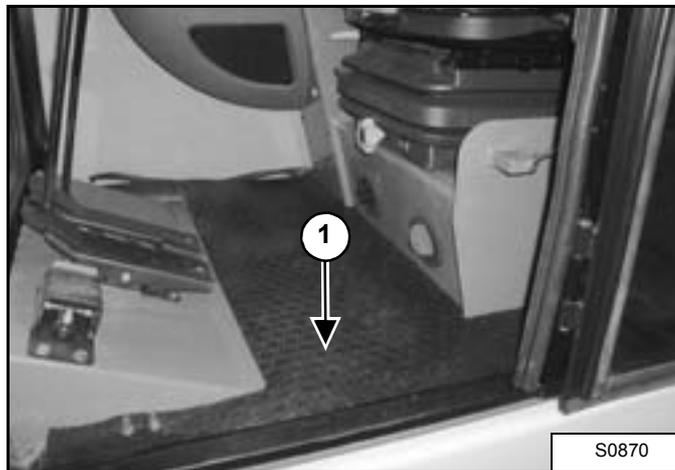
2. Pull up on and remove the floor mat (1).
