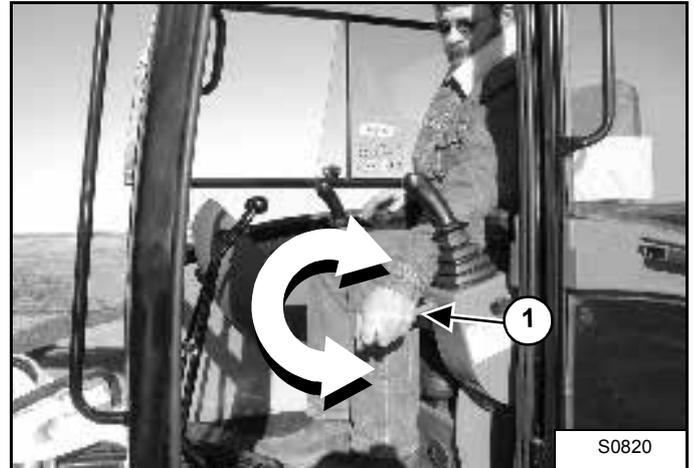
Raise the console before exiting the cab. Pull up on the handle [Figure 27]. The lift spring will assist in raising the console.
