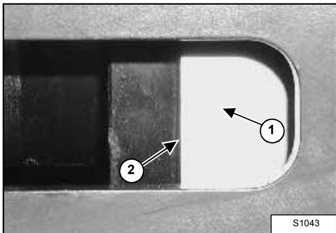
7. Add grease to the track tensioner until the track tension indicator (1) is flush with the cylinder edge (2) [Figure 176] & [Figure 177].
