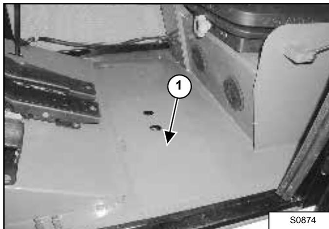
3. Remove the battery compartment cover (1).
