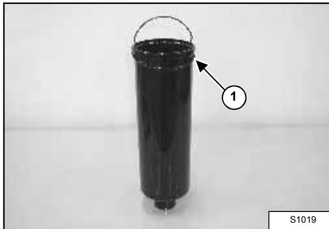
1. Inspect the O-rings (1) on the outside and inside bottom of the filter bowl. Replace the O-rings if damaged.
