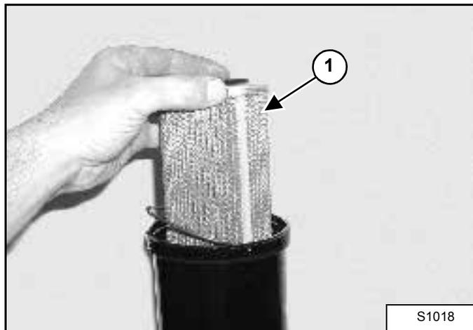
2. Install a new filter (1) in the filter bowl.
