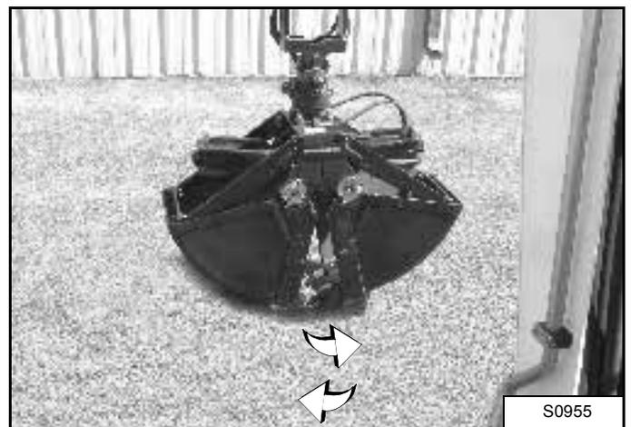
Push and hold the switch (1) [Figure 52] to rotate the bucket in the counter clockwise direction [Figure 53].
