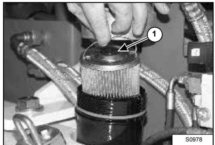
3. Remove the filter (1) from the filter housing.
