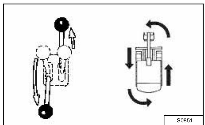
Push the right steering lever forward and pull the left steering lever backward [Figure 22].
