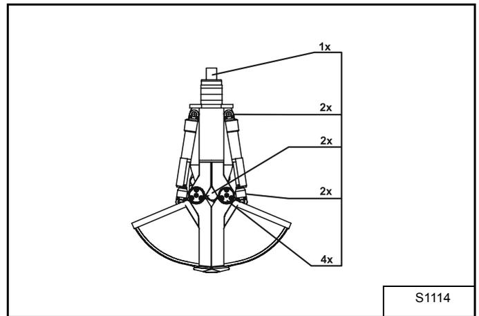
Always use a good quality Lithium based multipurpose grease when lubricating the attachment. Apply the lubricant until extra grease shows.
