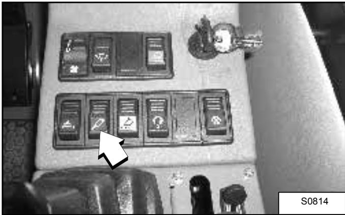
When the grab is operated, the change-over switch must be in position "Rock breaker OFF" (see [Figure 25])
