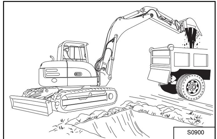
Extend the arm and uncurl the bucket to dump the material into a pile or truck [Figure 84].
