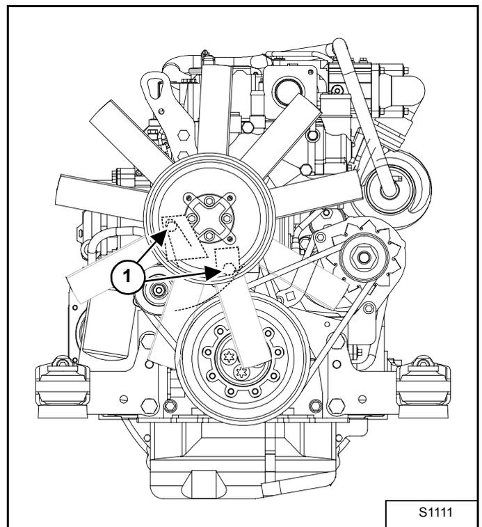
3. Loosen the two bolts (1) on the fuel pump mount. Rotate the fuel pump until the belt is correctly tensioned.
