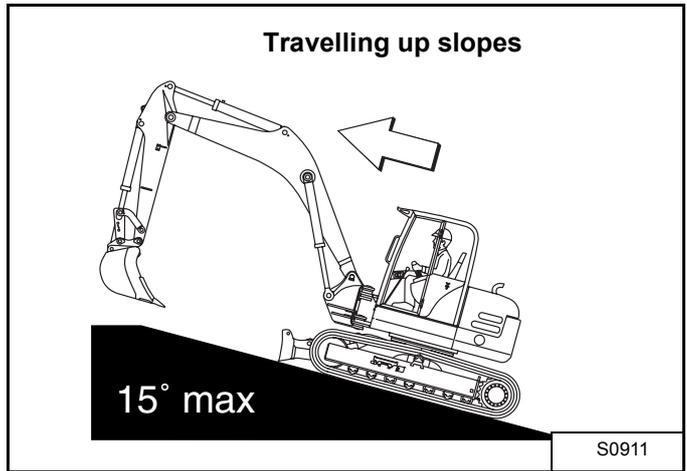
When travelling up slopes or on side slopes that are 15 degrees or less, position the machine as shown and run the engine slow [Figure 94] & [Figure 95].
