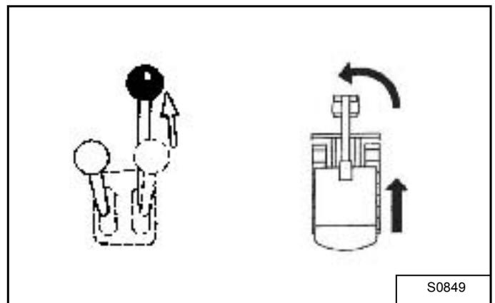
Push the right steering lever forward to turn left while travelling forward [Figure 20].
