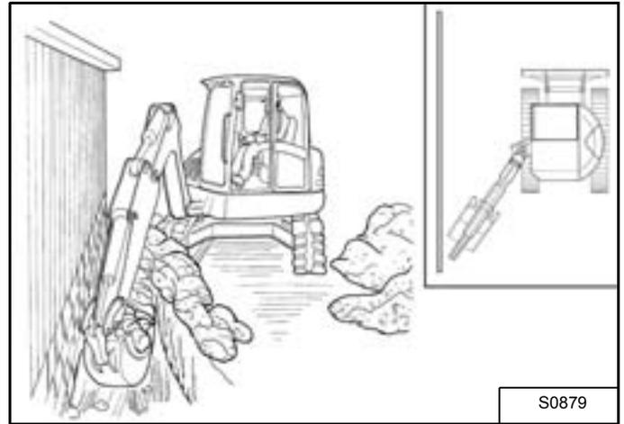
Note: The purpose of the boom swing pedal is to offset the boom with respect to the upperstructure for digging close to a structure [Figure 25].
