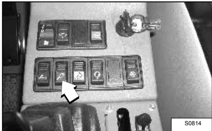
Set the change-over switch (see figure [Figure 55]) to "Rock breaker operation".
