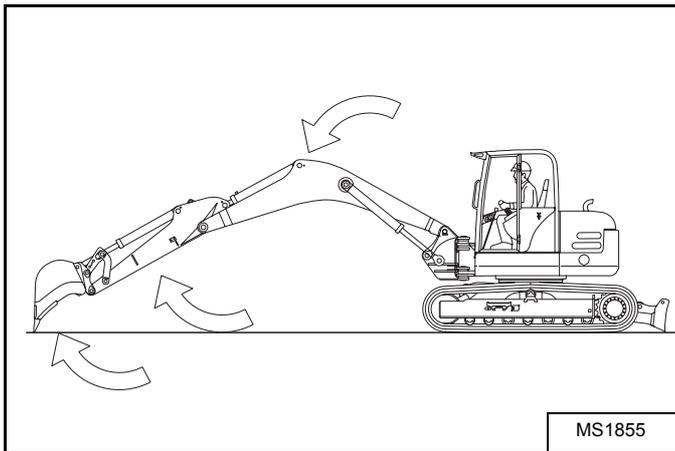
Extend the arm, lower the boom and open the bucket [Figure 81].
