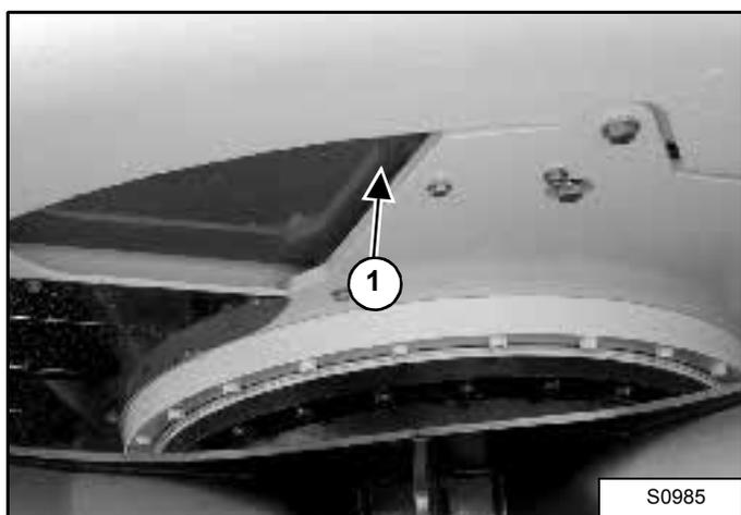
1. Remove the cap (1) from the drain.
