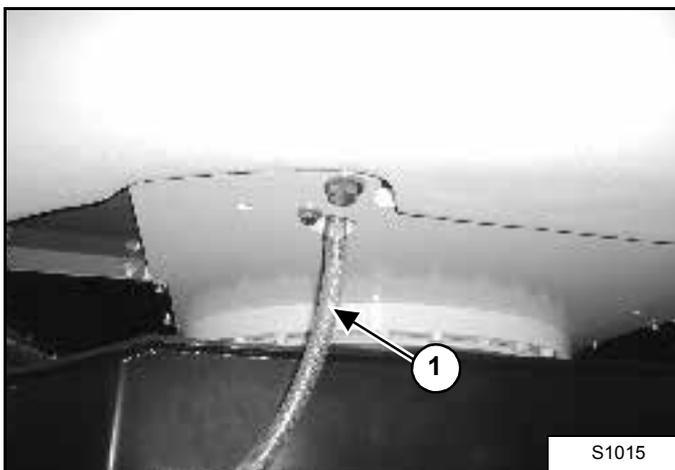
2. Install the drain hose (1) on the hydraulic reservoir. Tighten the hose until oil starts to drain from the reservoir.
