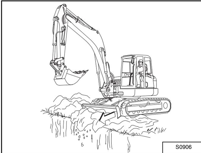
Use the blade to backfill the trench or hole after excavating [Figure 90].
