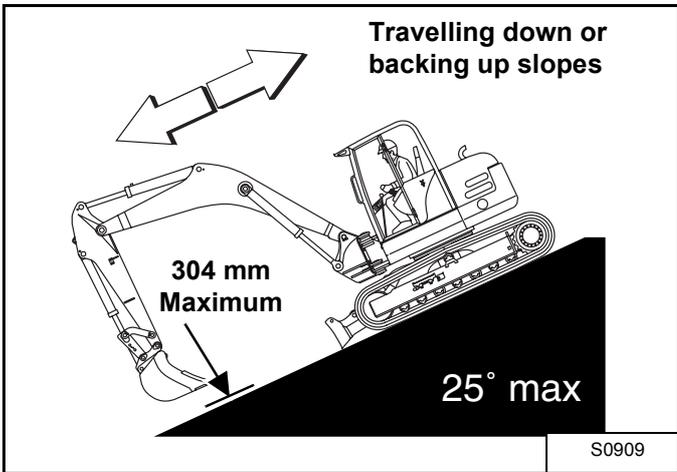
When going down grades that exceed 15 degrees, put the machine in the position shown, and run the engine slowly [Figure 93].
