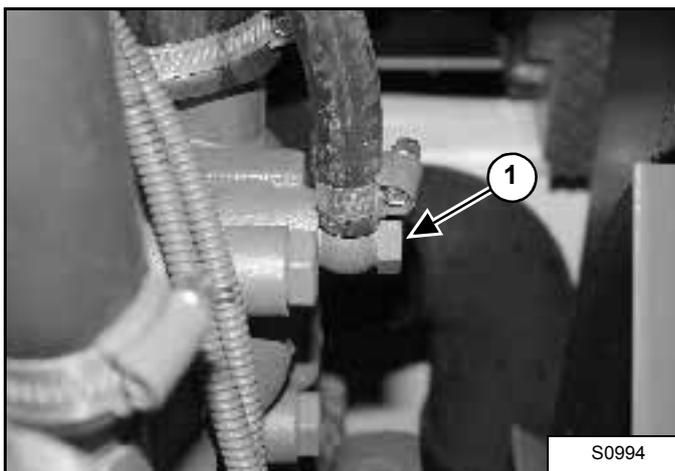
2. Remove the plug (1) from the back side of the engine block.
