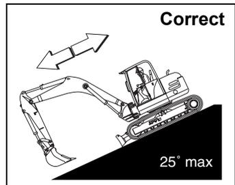
⚠ Never exceed 25° when going down or backing up a slope.
