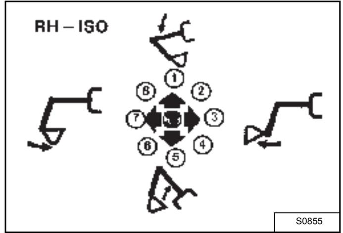
The right lever is used to operate the boom and bucket.
