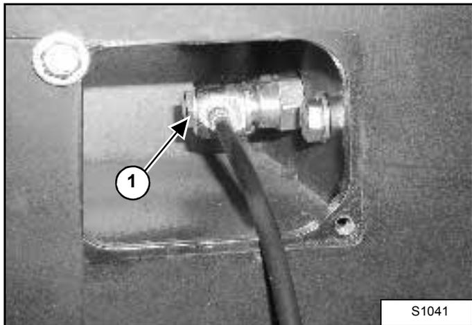
6. Install the adapter (1) on the track tensioner.
