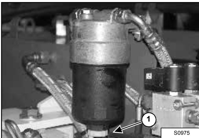
1. Loosen the drain (1) at the bottom of the filter housing and drain the fuel out of the housing.
