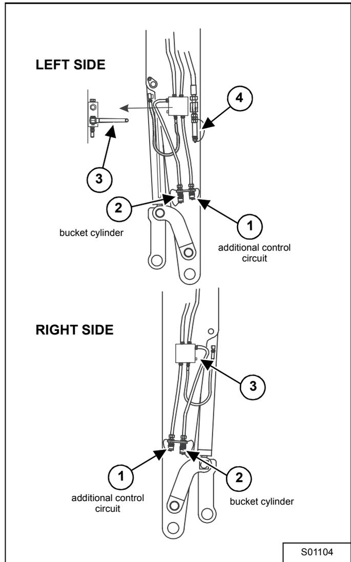
The hydraulic rock breaker is mechanically attached in the same manner as a bucket attachment.
