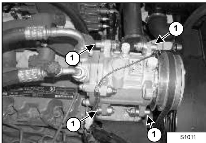
3. Loosen the bolts (1) and rotate the compressor until the belt is correctly tensioned.
