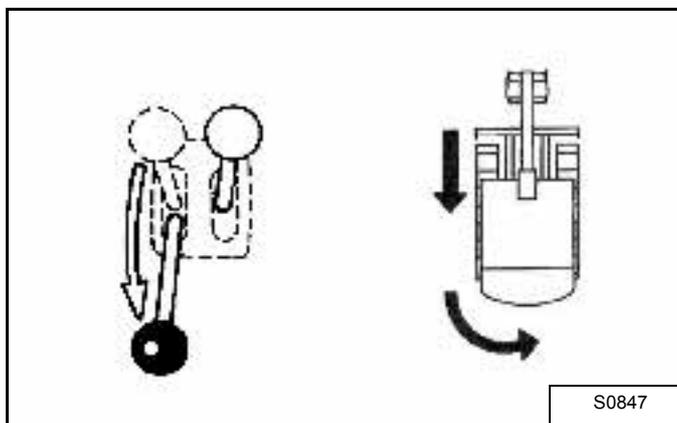
Pull the left steering lever backward to turn right [Figure 18] while travelling backward.
