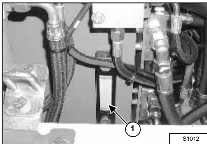
1. Check the hydraulic fluid level, it must be visible in the sight gauge (1).
