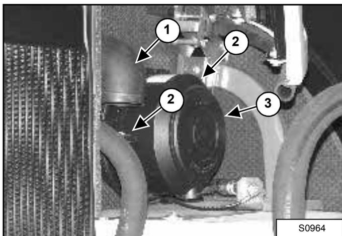
1. Open the right side cover to inspect the air intake (1) for damage or restrictions.
