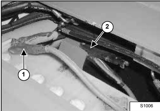
1. Connect one end of the first cable to the positive (+) terminal of the booster battery. Connect the other end of the same cable to the positive (+) terminal (1) of the Excavator battery.
