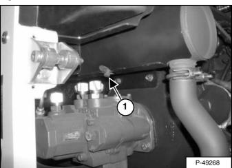
Remove the plug (Item 1) [Figure PM-39] from the bottom of the silencer.
