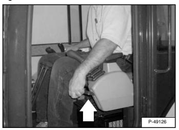
Pull up on the release handle **[Figure OI-6]**. The lifting spring will assist in raising the console.
