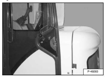
Push the door all the way open until the latch engages to hold the door in the open position.
