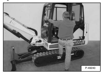
Use the grab handles, tracks and safety treads to enter the canopy/cab [Figure OI-45].
