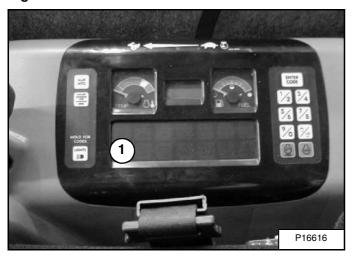
When High Range is engaged, the two speed travel icon (Item 1) [Figure OI-8] will illuminate.
