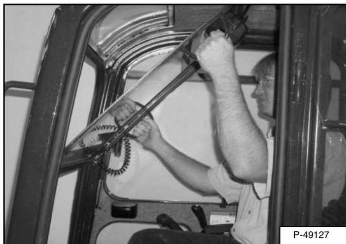
Use both window grab handles to pull the top of the window in **[Figure OI-19]**.
