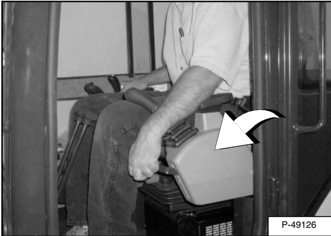
Lower the control console [Figure OI-48].
