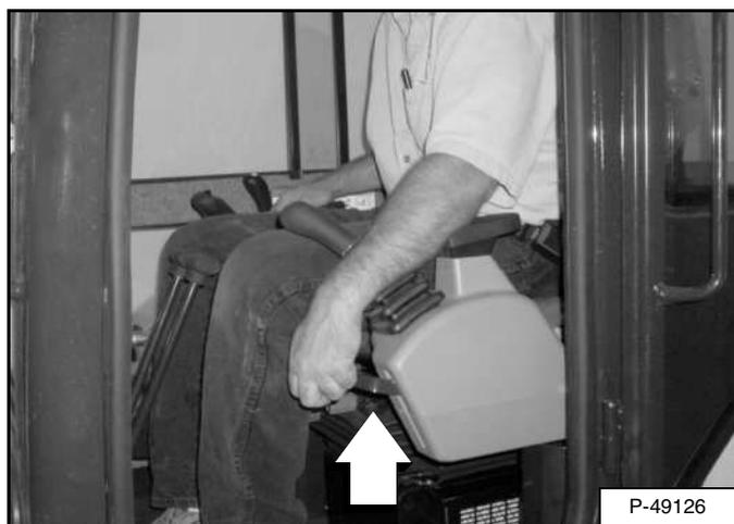
Pull up on the release handle [Figure OI-6]. The lifting spring will assist in raising the console.
