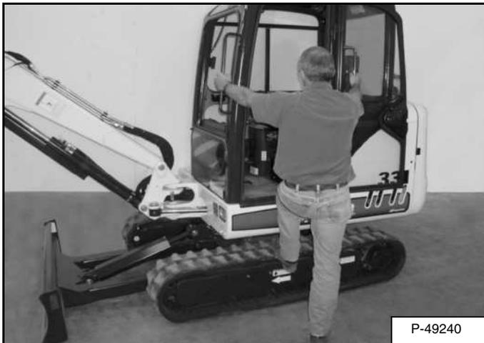
Use the grab handles, tracks and safety treads to enter the canopy/cab [Figure OI-45].
