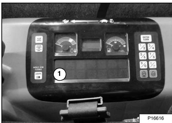
When High Range is engaged, the two speed travel icon (Item 1) [Figure OI-8] will illuminate.
