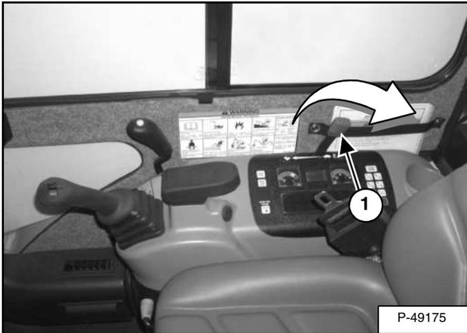
Move the engine speed control (Item 1) [Figure OI-52] to low idle.
