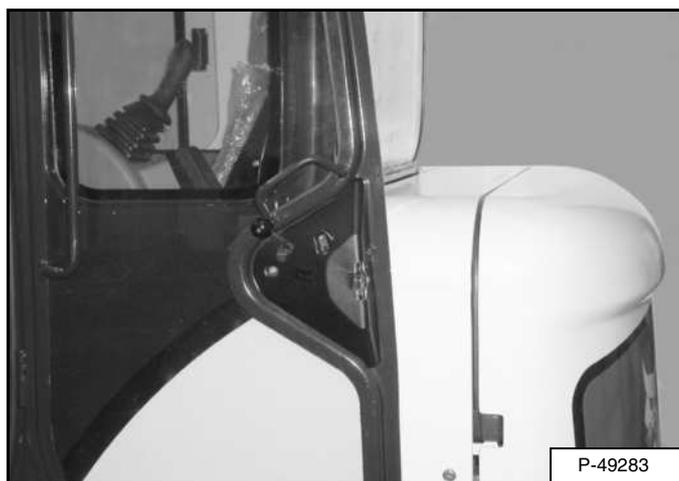
Push the door all the way open until the latch engages to hold the door in the open position.
