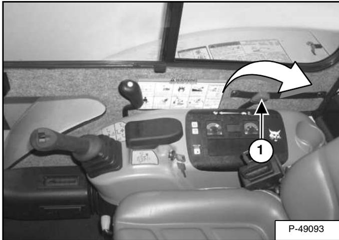
Move the engine speed control (Item 1) [Figure OI-50] to low idle.
