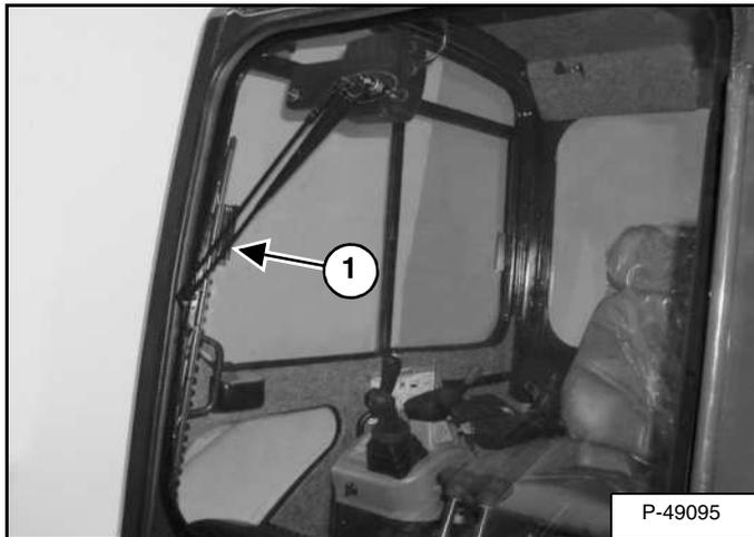
The front window is equipped with a wiper (Item 1) [Figure OI-16] and washer.
