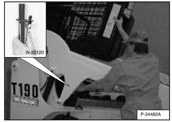
Pull down on the bottom of the operator cab until it stops at the latching mechanism [Figure 133].
