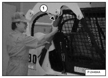
Have a second person install the lift arm support device (1) **[Figure 128]** over the rod of one of the lift cylinders.
