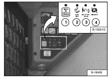
There are display lights (1, 2, 3, and 4) **[Figure 15]** located on the left instrument panel that must be ON to operate the machine.
