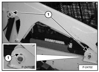
All lift arm and cylinder pivots have a large pin held in position with a retainer bolt and lock nut (1) **[Figure 191]**.
