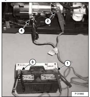
Connect the end of the first cable (1) [Figure 160] to the positive (+) terminal of the booster battery. Connect the other end of the same cable (2) [Figure 160] to the positive terminal on the loader starter.
