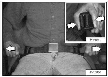
Squeeze both seat belt adjusters to release and lengthen each half of the seat belt **[Figure 55]**.
