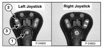
Press the button (1) **[Figure 28]** on the left joystick once to engage Speed Management.
