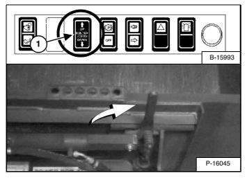
Push and hold the BOB-TACH "WEDGES UP" Switch (Front Accessory Panel) (1) [Figure 88] until the wedges are fully raised.
