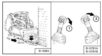
Lower the lift arms (1) **[Figure 112]** and put the cutting edge of the bucket on the ground (2) **[Figure 112]**. Drive forward to the edge of the hole to push the material into the hole.
