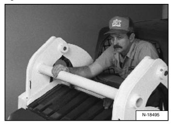
Exit through the rear of the operator cab [Figure 74].
