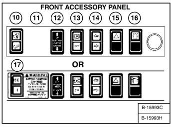
NOTE: Parking Brake (13) [Figure 12] is Standard on all loaders.
