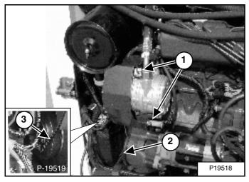
Loosen the mounting and adjustment bolts (1) [Figure 180].
