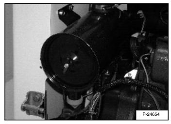
Remove the wing nut and remove the dust cover [Figure 144].
