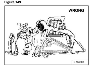
Use a clean, approved safety container to add fuel of the correct specifications. Add fuel only in an area that has free movement of air and no open flames or sparks. NO SMOKING [Figure 149]!
