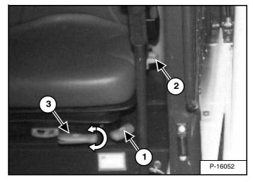
*Suspension Seat* - (Option & Field Accessory) Release the lever (1) **[Figure 54]** to adjust the seat distance from the levers and footrests.
