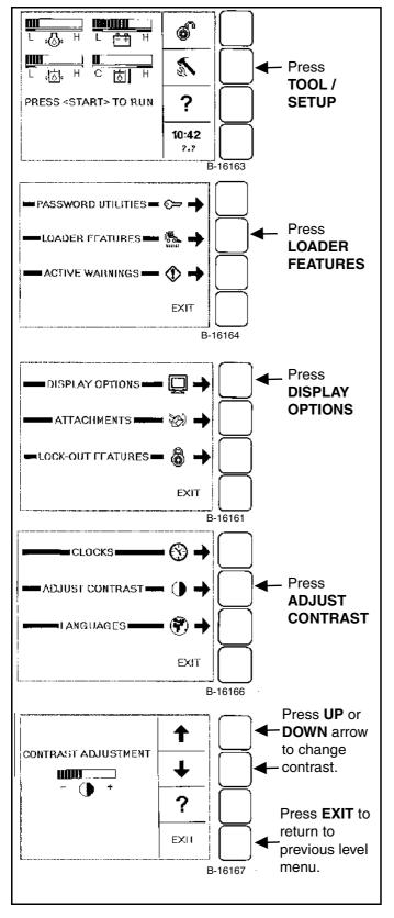
All new machines with Keyless Instrumentation arrive at Bobcat dealerships with the panel in locked mode. This means that a password must be used to start the engine [Figure 201].
