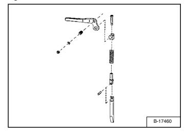
Inspect the mounting frame on the attachment and the Bob-Tach, linkages and wedges for excessive wear or damage **[Figure 197]**. Replace any parts that are damaged, bent, or missing. Keep all fasteners tight.
