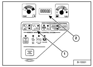
Press and hold the BUCKET POSITIONING Button (1) [Figure 203] for two seconds. If the SHUTDOWN feature is installed, Shtdn will appear in the HOURMETER / CODE DISPLAY (2) [Figure 203]. If it is not installed, BASE will appear.
