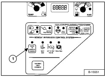
Press the PRESS TO OPERATE LOADER Button (1) [Figure 61] to activate the BICS system and to perform hydraulic and loader functions. (See Cold Temperature Starting on Page 33.)
