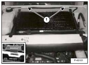
Lift and pull the rear grill and remove it from the loader **[Figure 139]**.
