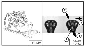
Press and hold the float button (1) **[Figure 116]** while the joystick is in neutral. While lowering the lift arms (2) **[Figure 116]**, release the float button.
