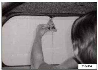
Pull on the tag on the top of the rear window to remove the rubber cord **[Figure 73]**.
