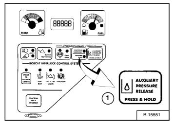
Press the AUXILIARY PRESSURE RELEASE Button (1) [Figure 44]. Hold it for two seconds after the engine comes to a complete stop. The pressure will be released.
