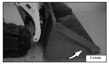
Tilt the Bob-Tach backward until the cutting edge of the bucket (or other attachment) is slightly off the ground **[Figure 87]**.
