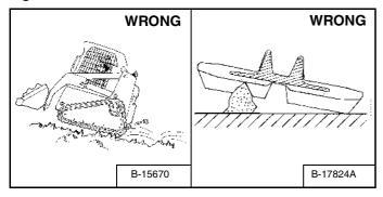
Avoid operating or turning on sharp objects such as jagged rocks, broken concrete, quarry materials or scrap applications. This can cause cuts on the lug surface of the tracks [Figure 94].
