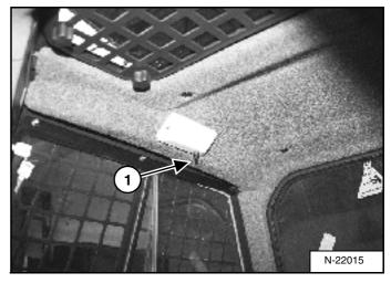
Push the button (1) **[Figure 10]** to turn the light ON. Push the button again to turn OFF.
