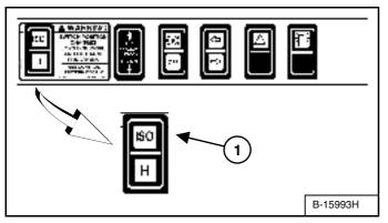
Select the 'ISO' control pattern by pressing the top of the switch (1) [Figure 25].
