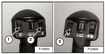
You can use additional switches (1, 2 and 3) [Figure 47] on the right and left control handles for functions which control some attachments.
