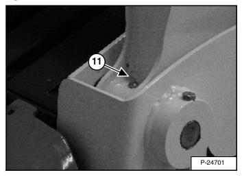
11. Lift Arm Link Pivot Pin (Both Sides) [Figure 189].
