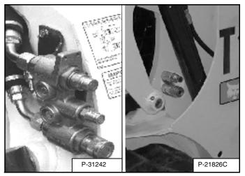
*To Connect:* Remove dirt or debris from the surface of both the male and female couplers, and from the outside diameter of the male coupler. Visually check the couplers for corroding, cracking, damage or excessive wear. If any of these conditions exist, the coupler(s) **[Figure 43]** must be replaced.
