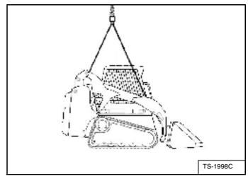
Attach cables or chains to lift eyes [Figure 121].
