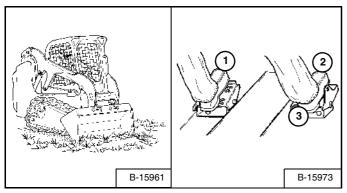
Lower the lift arms all the way (1) **[Figure 103]**. Put the cutting edge of the bucket on the ground (2) **[Figure 103]**.
