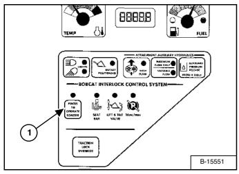
Press the PRESS TO OPERATE LOADER Button (1) **[Figure 65]** to activate the BICS system and to perform hydraulic and loader functions.
