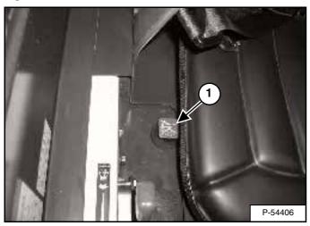
The lift arm by-pass control (1) **[Figure 16]** is used to lower the lift arms if the lift arms cannot be lowered during normal operations.
