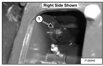
NOTE: There are stop blocks (1) [Figure 175] that keep the cylinders from turning. If the cylinders turn, the fittings will not be accessible. Check the stop block bolts to be sure they are tight.
