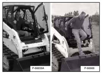
Stop the Bobcat Loader on level ground.
