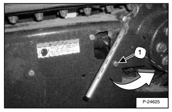
Install the bleed tool (MEL-1560) on the *bleed fitting* (1) **[Figure 176]** (upper fitting on left side, lower fitting on right side).
