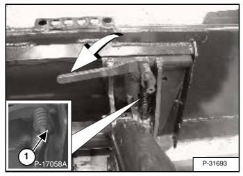
Push down on the Bob-Tach levers until they are fully engaged in the locked position (1) **[Figure 81]** (wedges fully extended).
