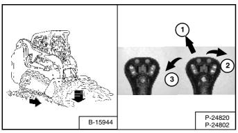
Lower the lift arms all the way (1) **[Figure 117]**. Put the cutting edge of the bucket on the ground (2) **[Figure 117]**.
