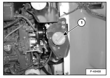
Remove the fuel fill cap (1) [Figure 148].
