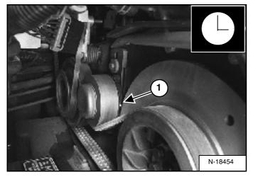
Push the idler pulley against the belt, using a pry bar **[Figure 182]**. The pointer will be at the 3 o'clock position (1) **[Figure 182]** when the idler pulley is against the stop (maximum movement).
