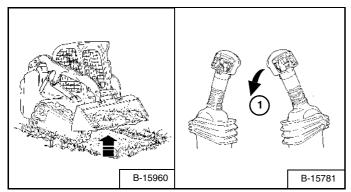
Tilt the bucket backward (1) [Figure 111] as far as it will go when the bucket is full.
