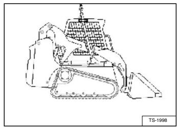
Install the kit as explained in the Instructions with the kit and attach lift as shown [Figure 120].
