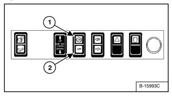
Press the top of the switch (1) **[Figure 19]** to engage the parking brake. The traction drive system will be locked.
