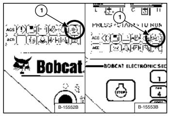
It is important to change the air filter element only when the Air Cleaner Icon in the right panel is ON (1) [Figure 142] and you hear three beeps from the alarm.
