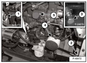
Park the machine on level ground. Open the rear door and remove the dipstick (1) [Figure 152].
