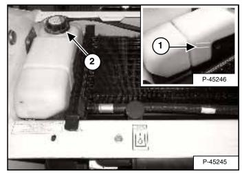
Check the coolant level on the side of the recovery tank (1) **[Figure 154]**. The level must be between the MIN and MAX marks.
