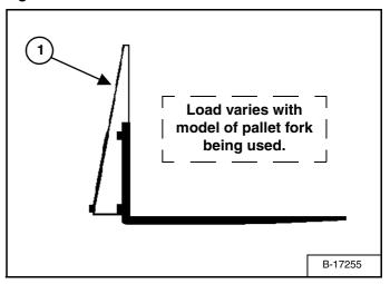
The maximum load to be carried when using a pallet fork is shown on a decal located on the pallet fork frame (1) **[Figure 78]**.
