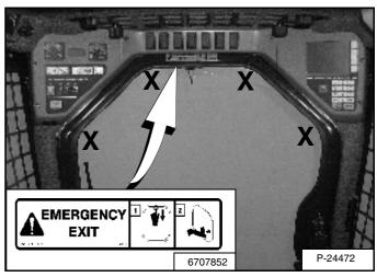
Push the window out with your foot **[Figure 76]** at any corner of the window.
