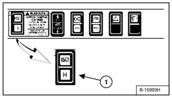
Select the 'H' control pattern by pressing the bottom of the switch (1) [Figure 22].
