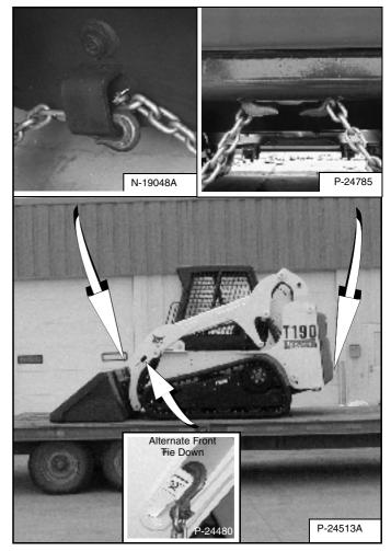
Use the following procedure to fasten the Bobcat Loader to the transport vehicle to prevent the loader from moving during sudden stops or when going up or down slopes **[Figure 123]**.
