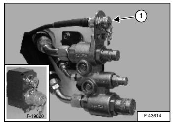
You will need the Dual-Connector (7-pin / 14-pin) kit (1) **[Figure 48]** to operate early model attachments. See your Bobcat Loader dealer.
