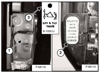
The cab door has a sensor (1) **[Figure 135]** installed which deactivates the lift and tilt valves when the door is open.
