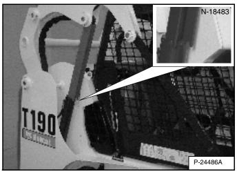
Lower the lift arms slowly until the lift arm support device is held between the lift arms and the lift cylinder [Figure 129]. The tabs of the lift arm support device must go under the cylinder (Inset) [Figure 129].
