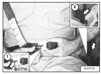
*3-Point Restraint - (Option)* Connect the shoulder belt to the lap belt (1) **[Figure 56]**. Pull the lap belt across to the left side of the seat (2) **[Figure 56]** and fasten.
