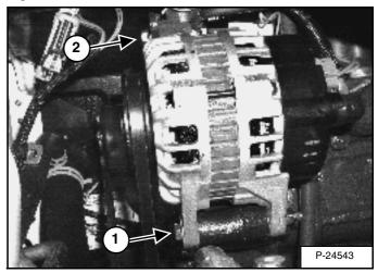
Loosen the alternator mounting bolt (1) and adjustment bolt (2) [Figure 179].
