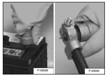
Always clean the battery terminals and cable ends when installing a new or used battery [Figure 162].
