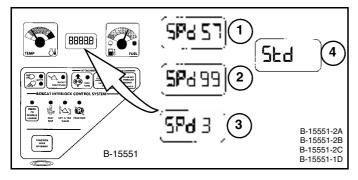
When Speed Management is engaged, the machine will travel at 57% of Standard travel speed and the percentage **[SPd 57]** will appear in the display (1) **[Figure 29]**.
