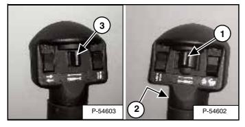
*VARIABLE FLOW* allows for slow-to-fast movement of auxiliary functions. If you move the auxiliary switch (1) **[Figure 40]** half-way, the auxiliary functions move at approximately one-half speed.
