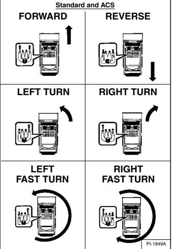
The steering levers control forward and reverse travel and turning the loader [Figure 21].
