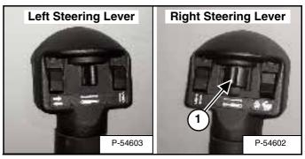
Push switch (1) **[Figure 50]** to the right or left to change fluid flow direction. (EXAMPLE: Side shift on the Planer.)
