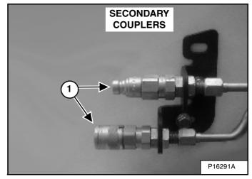
The secondary front auxiliary quick couplers (1) **[Figure 49]** are available a Field Installed Accessory. These are used when there is a need for additional auxiliary hydraulics (EXAMPLE: Planer side shift).
