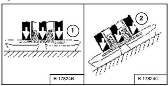
The track carriage components will wear faster when operated on a slope. When the machine is operated on a level surface, the weight of the machine is distributed throughout the entire surface of the rollers to the tracks (1) [Figure 92]. When operated on a slope, the weight is directed to the edge of the rollers and against the lugs of the track (2) [Figure 92] which causes increased wear.
