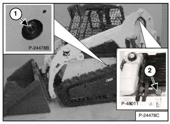
Check the fluid level in the sight gauge (1) [Figure 163].
