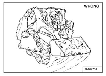
*Turning:* Use a gradual turn (one lever farther forward than the other) instead of a fast turn (one lever forward and one lever backward) on asphalt or concrete surfaces to prevent reduced track life or derailing of tracks **[Figure 90]**.
