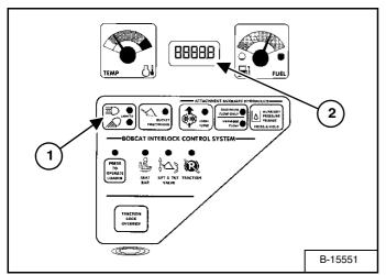
Press and hold the LIGHT Button (1) [Figure 143] for two seconds.
