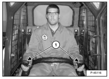
Both joysticks control drive and steering and are located on the right and left side in front of the seat (1) [Figure 23].
