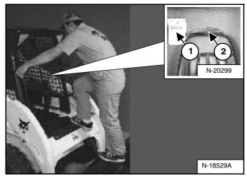
Use the bucket or attachment steps, grab handles and safety treads (on top of the loader lift arms and frame) to get on and off the loader **[Figure 52]**. Do not jump.
