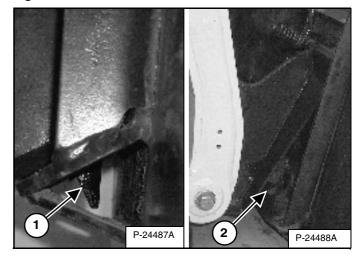
The wedges (1) **[Figure 82]** must extend through the holes (2) **[Figure 82]** in the mounting frame of the bucket (or attachment), securely fastening the bucket to the Bob-Tach.
