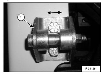
The door latch (1) **[Figure 138]** can be adjusted side to side for alignment with the door latch mechanism.
