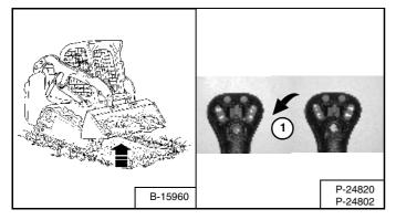
Tilt the bucket backward (1) **[Figure 118]** as far as it will go when the bucket is full.
