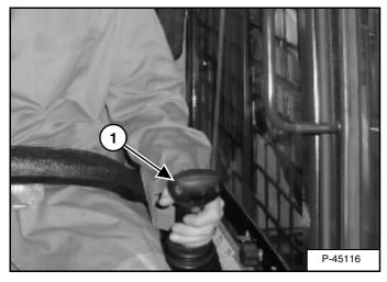
The joystick which controls drive and steering is on the left side in front of the seat (1) **[Figure 26]**.
