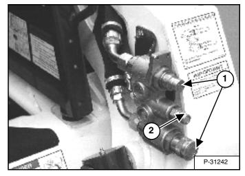
The High-Flow function provides additional flow to the system to operate an attachment which requires more hydraulic flow (EXAMPLE: Planer).
