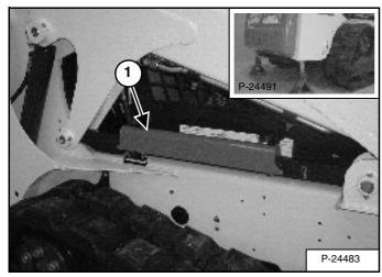
Put jackstands under the rear corners of the loader frame (Inset) [Figure 132].
