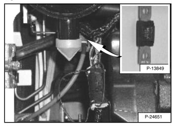
The loader has a 12 volt, negative ground alternator charging system. The electrical system is protected by fuses located in the cab on the steering control panel and a 100 amp. master fuse [Figure 156] in the engine compartment on the left side of the engine, under the air cleaner. The fuses will protect the electrical system when there is an electrical overload. The reason for the overload must be found before starting the engine again.
