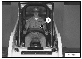
The seat bar restraint system has a pivoting seat bar with arm rests (1) [Figure 13].
