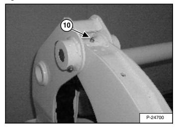
10. Lift Arm Pivot Pin (Both Sides) [Figure 188].
