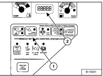
Press BUCKET POSITIONING button (1) [Figure 38] to engage the bucket position function. (The light will be on.) Press again to disengage.
