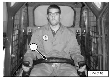
The Bobcat Interlock Control System (BICS) has a pivoting seat bar with arm rests (1) [Figure 14].
