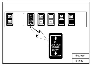
Push and hold the BOB-TACH "WEDGES UP" switch [Figure 196] until wedges are fully raised. Push and hold the BOB-TACH "WEDGES DOWN" switch [Figure 196] until the wedges are fully down.
