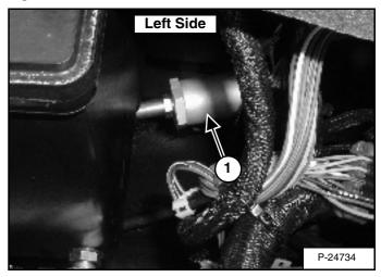
Remove the case drain filters (1) [Figure 167] and [Figure 168]. Disassemble the filter housings, thoroughly clean and install new filters. Reassemble and install the case drain filters. (See Lowering on Page 75.)
