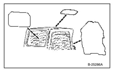
Available for special applications to restrict material from entering cab openings. Kit includes 12 mm Lexan<sup>™</sup> front door, top and rear windows.
