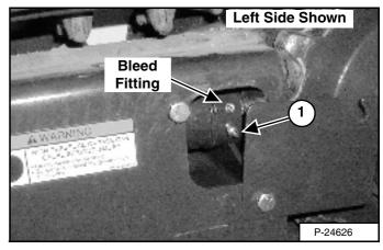
Loosen the cover bolts and turn the cover down [Figure 174].
