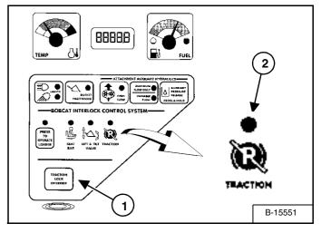
(Functions Only When The Seat Bar Is Raised And The Engine Is Running) There is a TRACTION LOCK OVERRIDE Button (1) [Figure 17] on the left instrument panel which will allow you to use the steering levers to move the loader forward & backward when using the backhoe attachment or for loader service.
