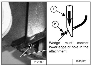
The wedges (1) [Figure 193] must extend through the holes in the attachment mounting frame (2) [Figure 193].
