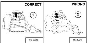
**Digging And Leveling:** Keep the full length of the tracks in contact with the ground (1) **[Figure 91]** for best traction. Raising the front end of the tracks off the ground (2) **[Figure 91]** will reduce traction and cause increased track wear.
