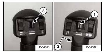
Press the auxiliary hydraulics button for VARIABLE FLOW.
