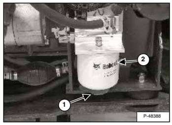
Loosen the drain (1) **[Figure 150]** at the bottom of the filter element to remove water from the filter.
