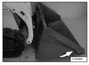
Tilt the Bob-Tach backward until the cutting edge of the bucket (or other attachment) is slightly off the ground **[Figure 80]**.
