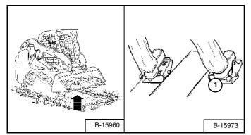
Tilt the bucket backward (1) [Figure 104] as far as it will go when the bucket is full.
