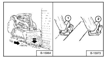
Lower the lift arms (1) **[Figure 105]** and put the cutting edge of the bucket on the ground (2) **[Figure 105]**. Drive forward to the edge of the hole to push the material into the hole.
