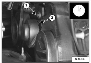
Loosen the bolt (1) [Figure 181] on the spring loaded drive idler.
