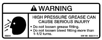
Turn the tool 1/4 turn counterclockwise and let the grease flow into a container. Turn the tool one additional turn to continue to release pressure.
