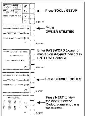
The Display Panel will list the Code Number, (CODE) hourmeter reading when the error occurred (HOUR), and the User (USER) who was logged in to operate the machine when the error occurred.
