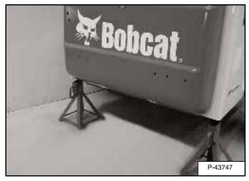
Install jackstands under the rear of the loader frame [Figure 130].
