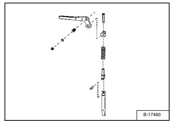
Inspect the mounting frame on the attachment and Bob-Tach, linkages and wedges for excessive wear or damage **[Figure 194]**. Replace any parts that are damaged, bent or missing. Keep all fasteners tight.
