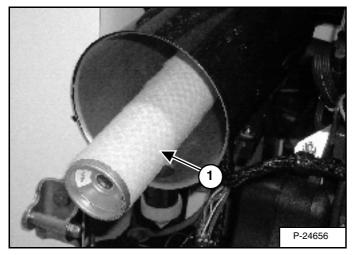
Remove the inner filter element (1) [Figure 146].
