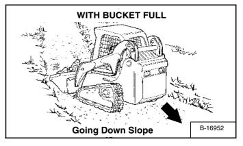
With a full bucket, go up or down the slope with the heavy end toward the top of the slope [Figure 95] and [Figure 96].
