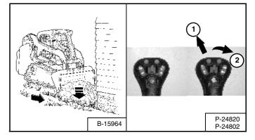
Lower the lift arms (1) **[Figure 119]** and put the cutting edge of the bucket on the ground (2) **[Figure 119]**. Drive forward to the edge of the hole to push the material into the hole.
