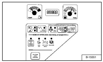
Frequently monitor the temperature and fuel gauges and BICS lights (all must be ON to operate loader) [Figure 67].
