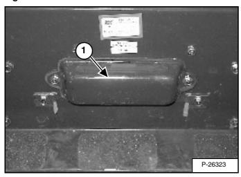
The electrical system is protected from overload by fuses and relays under the fuse panel cover (1) **[Figure 157]**. A decal is inside the cover to show location and amp ratings.
