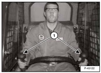
The control levers (1) **[Figure 20]** are on the left and right side in front of the seat.
