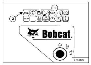
Turn the key switch to RUN [Figure 59]. The indicator lights on the right instrument panel [Figure 59] will come ON briefly and the Instrument Panel / monitoring system will do a self test.
