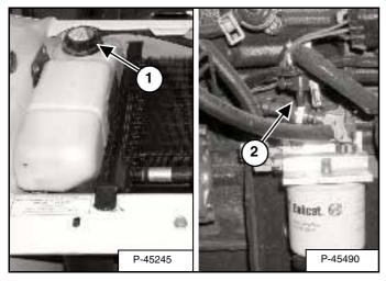
Remove the coolant fill cap (1) [Figure 155].
