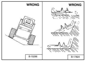
**Operating Conditions:** Avoid operating the loader with one track on a slope and the other on flat ground or with the end of the track turned up against a curb or mound **[Figure 93]**. This can cause the tracks to derail, cracks in the edge of the tracks or cracks at the edges of the embedded metal.
