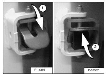
Move the door stop into the engaged position (1) **[Figure 137]** to hold the door open. Move to disengaged position (2) **[Figure 137]** allow the door to close.
