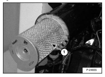
Remove the wing nut and remove the outer filter element (1) [Figure 145].
