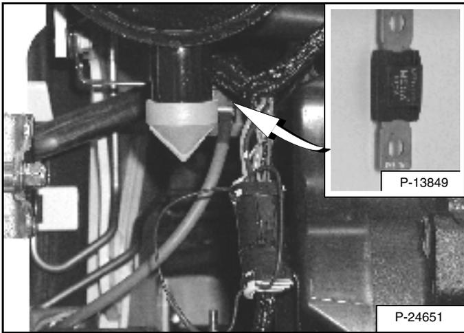
The loader has a 12 volt, negative ground alternator charging system. The electrical system is protected by fuses located in the cab on the steering control panel and a 100 amp. master fuse [Figure 156] in the engine compartment on the left side of the engine, under the air cleaner. The fuses will protect the electrical system when there is an electrical overload. The reason for the overload must be found before starting the engine again.
