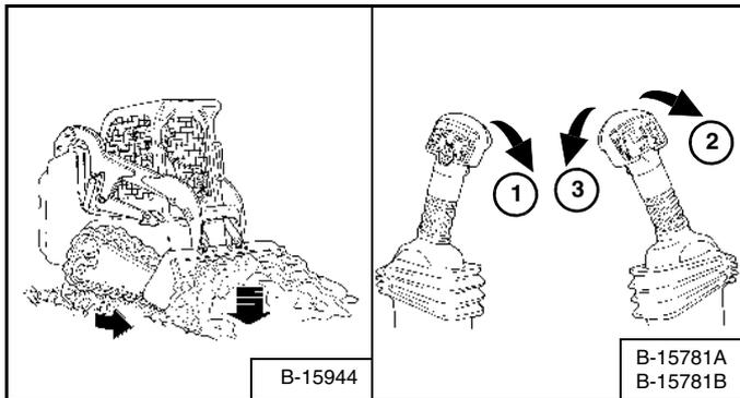
Lower the lift arms all the way (1) [Figure 110]. Tilt the bucket forward (2) [Figure 110] until the cutting edge of the bucket is on the ground.
