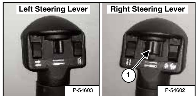
Push switch (1) [Figure 50] to the right or left to change fluid flow direction. (EXAMPLE: Side shift on the Planer.)
