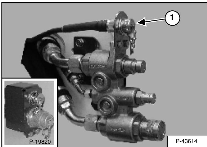
You will need the Dual-Connector (7-pin / 14-pin) kit (1) [Figure 48] to operate early model attachments. See your Bobcat Loader dealer.
