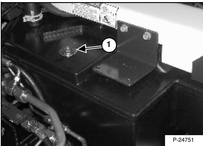
Raise the cab (See Raising on Page 74). Remove the plug from the top of the reservoir (1) [Figure 166] then pump the fluid out of the reservoir and into a container.
