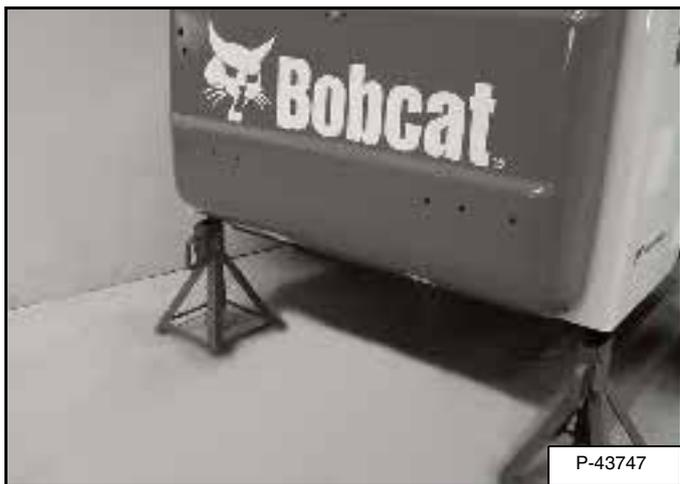
Install jackstands under the rear of the loader frame [Figure 130].
