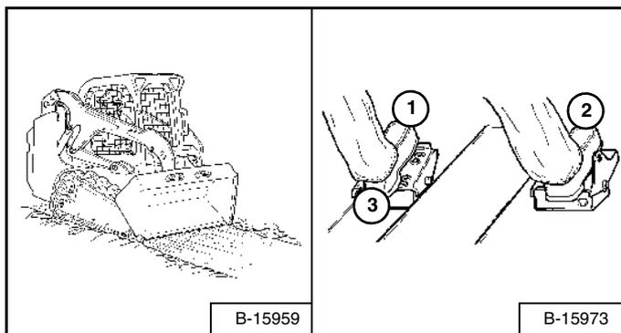
Put the lift arms in *float* position by pushing the pedal all the way forward (1) [Figure 102] until the pedal is locked in the forward position.
