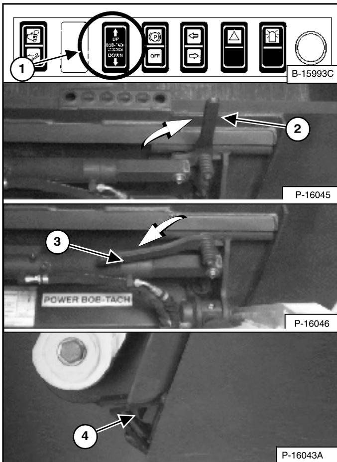
Push and hold BOB-TACH "WEDGES UP" switch (1) [Figure 85] (Front Accessory Panel) until levers (2) are in unlocked position (wedges fully raised).
