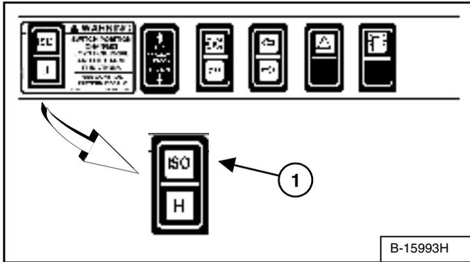
Select the 'ISO' control pattern by pressing the top of the switch (1) [Figure 25].
