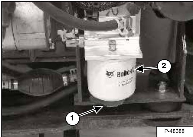
Loosen the drain (1) [Figure 150] at the bottom of the filter element to remove water from the filter.
