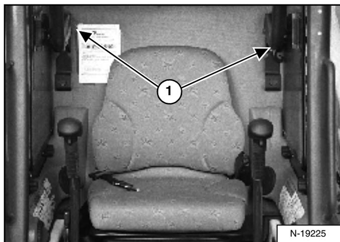
Use compressed air to clean any debris or dirt from the pivot parts (1) [Figure 125]. Do not lubricate. Inspect all mounting hardware. The correct bolt torque is 35 Nm.
