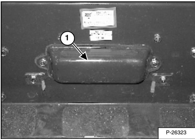
The electrical system is protected from overload by fuses and relays under the fuse panel cover (1) [Figure 157]. A decal is inside the cover to show location and amp ratings.
