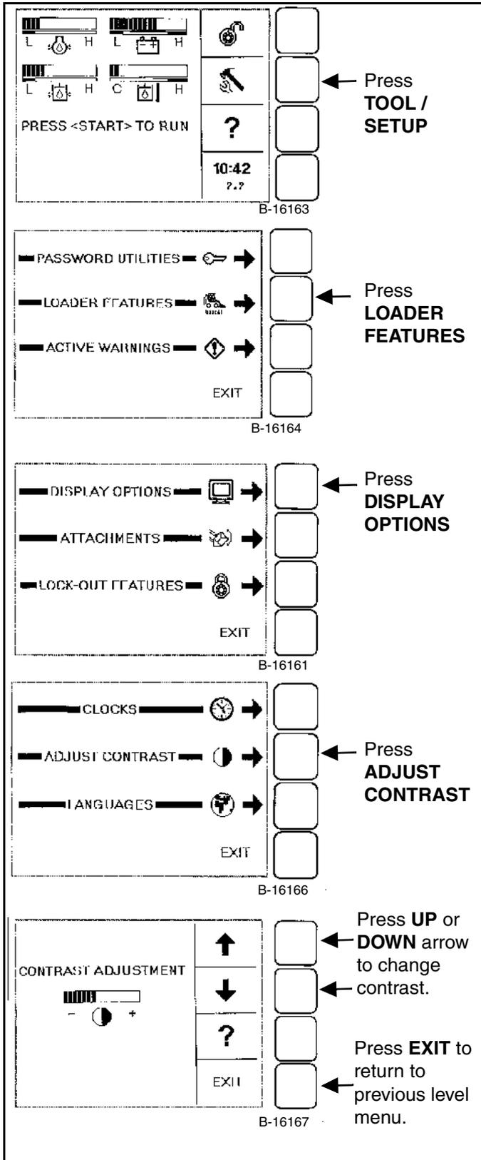
All new machines with Keyless Instrumentation arrive at Bobcat dealerships with the panel in locked mode. This means that a password must be used to start the engine [Figure 201].
