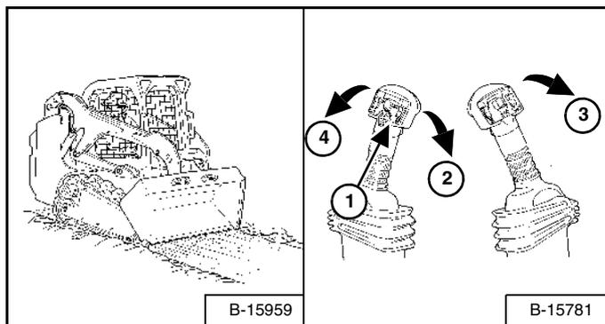
Press and hold the float button (1) [Figure 109] while the lever is in neutral. While lowering the lift arms (2) [Figure 109], release the float button.
