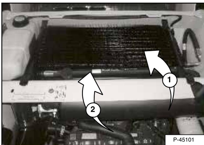
Use low air pressure or water pressure to clean the top of the oil cooler (1) [Figure 153].
