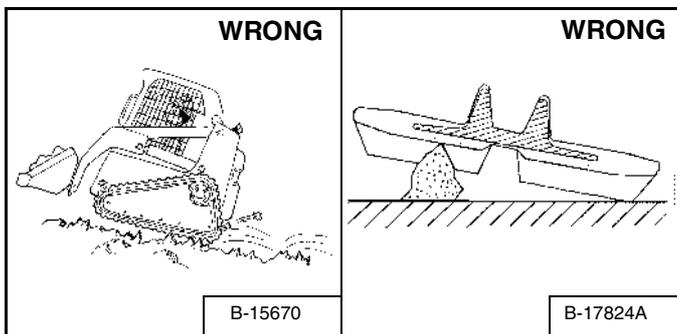
Avoid operating or turning on sharp objects such as jagged rocks, broken concrete, quarry materials or scrap applications. This can cause cuts on the lug surface of the tracks [Figure 94].
