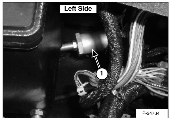
Remove the case drain filters (1) [Figure 167] and [Figure 168]. Disassemble the filter housings, thoroughly clean and install new filters. Reassemble and install the case drain filters. (See Lowering on Page 75.)
