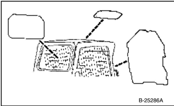
Available for special applications to restrict material from entering cab openings. Kit includes 12 mm Lexan™ front door, top and rear windows.
