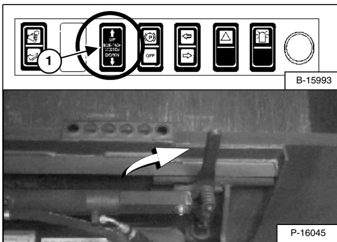
Push and hold the BOB-TACH "WEDGES UP" Switch (Front Accessory Panel) (1) [Figure 88] until the wedges are fully raised.
