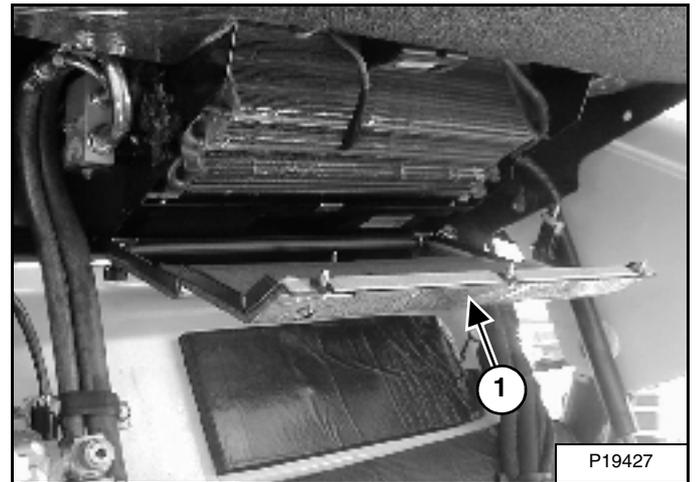
Raise the cab and remove the evaporator cover (1) [Figure 141].
