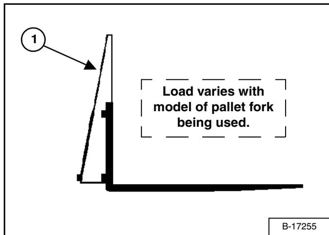
The maximum load to be carried when using a pallet fork is shown on a decal located on the pallet fork frame (1) [Figure 78].
