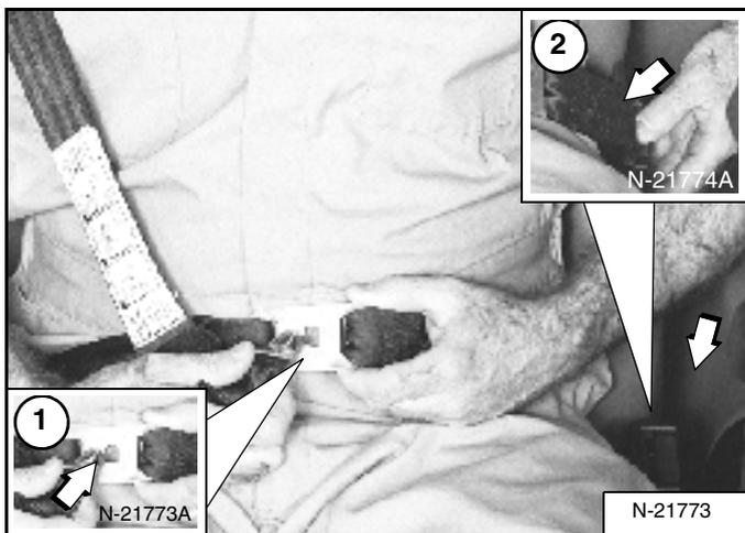
**3-Point Restraint - (Option)** Connect the shoulder belt to the lap belt (1) [Figure 56]. Pull the lap belt across to the left side of the seat (2) [Figure 56] and fasten.
