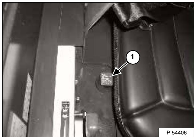
The lift arm by-pass control (1) [Figure 16] is used to lower the lift arms if the lift arms cannot be lowered during normal operations.
