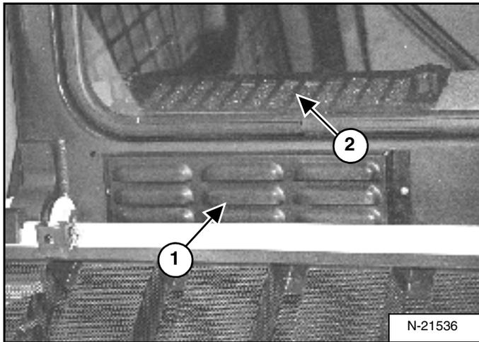
The *Fresh Air Filter* is located below the rear window of the cab (1) [Figure 140].
