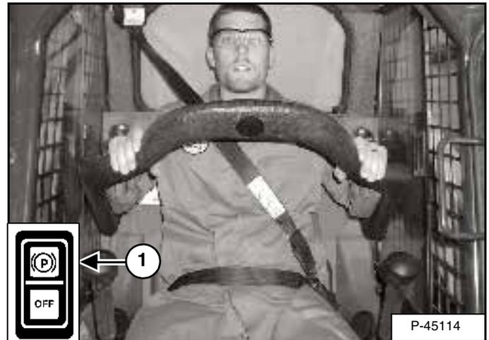
Lower the seat bar and engage the parking brake (1) [Figure 57].
