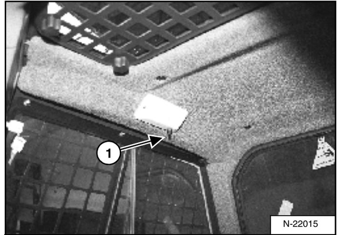
Push the button (1) [Figure 10] to turn the light ON. Push the button again to turn OFF.
