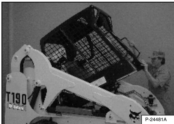
Lift on the grab handles and bottom of the operator cab [Figure 132] slowly until the cab is all the way up and the latching mechanism engages.
