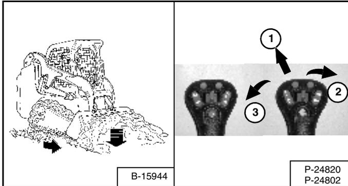
Lower the lift arms all the way (1) [Figure 117]. Put the cutting edge of the bucket on the ground (2) [Figure 117].
