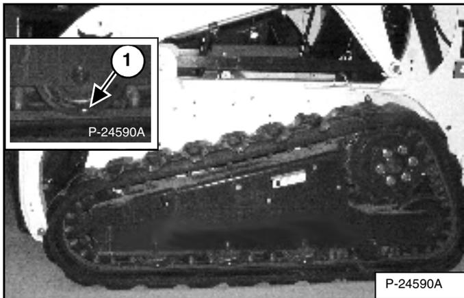
Raise one side of the loader and put jackstands at the front and rear of the loader frame so that the track is about 76 mm off the ground [Figure 172]. Lower the loader to the jackstands. Be sure the jackstands do not touch the tracks.
