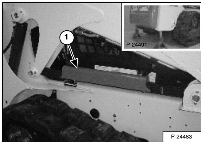
Put jackstands under the rear corners of the loader frame (Inset) [Figure 132].
