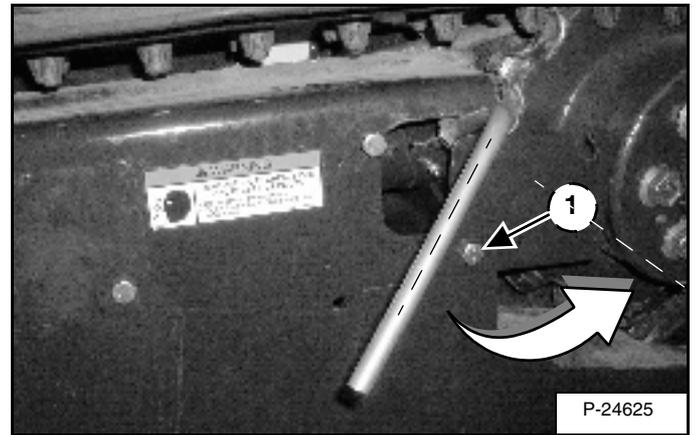
Install the bleed tool (MEL-1560) on the *bleed fitting* (1) [Figure 176] (upper fitting on left side, lower fitting on right side).
