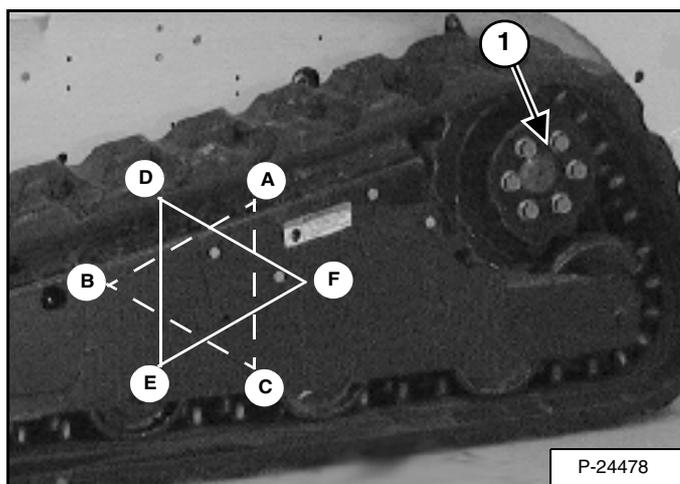
Check the torque of the six (6) track sprocket bolts (1) [Figure 178] for the correct service interval. Use a cross-pattern tightening sequence (A-B-C, D-E-F) [Figure 178] and then repeat to tighten the bolts to 407 Nm torque.
