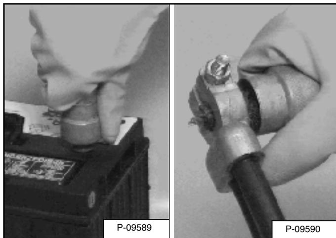
The battery cables must be clean and tight **[Figure 159]**. Check electrolyte level in the battery. Add distilled water as needed. Remove acid or corrosion from battery and cables with sodium bicarbonate (baking soda) and water solution.
