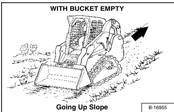
With empty bucket, go down or up the slope with the heavy end toward the top of the slope [Figure 97] and [Figure 98].
