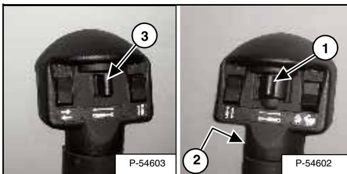
*VARIABLE FLOW* allows for slow-to-fast movement of auxiliary functions. If you move the auxiliary switch (1) [Figure 40] half-way, the auxiliary functions move at approximately one-half speed.
