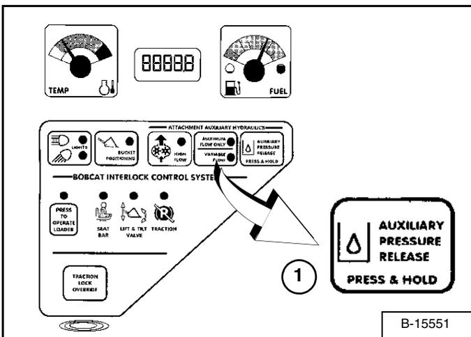
Press the AUXILIARY PRESSURE RELEASE Button (1) [Figure 44]. Hold it for two seconds after the engine comes to a complete stop. The pressure will be released.
