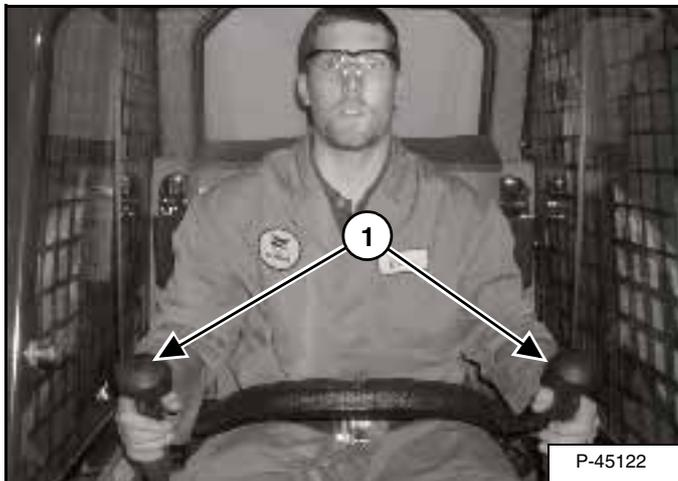
The control levers (1) [Figure 20] are on the left and right side in front of the seat.
