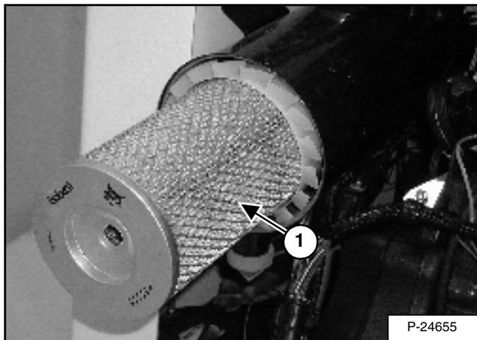
Remove the wing nut and remove the outer filter element (1) [Figure 145].
