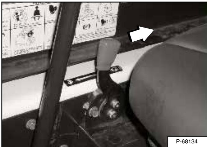
Pull the engine speed control fully backward [Figure 71] to decrease the engine speed.
