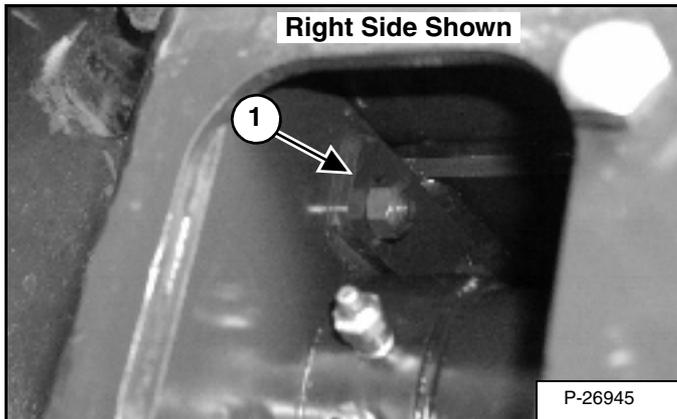
**NOTE:** There are stop blocks (1) [Figure 175] that keep the cylinders from turning. If the cylinders turn, the fittings will not be accessible. Check the stop block bolts to be sure they are tight.
