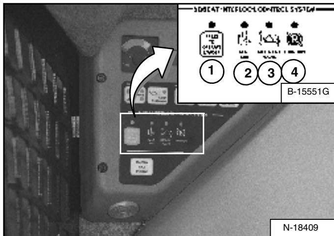
1. Sit in operator's seat. Turn key ON (*Key Switch Panel*), press RUN / ENTER Button (*Keyless Panel*), lower seat bar and disengage parking brake. Press the PRESS TO OPERATE LOADER Button. Three BICS lights (1, 2 and 3) [PRESS TO OPERATE LOADER, SEAT BAR, and LIFT & TILT VALVE] on left instrument panel should be ON [Figure 124].
