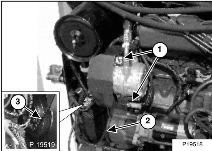
Loosen the mounting and adjustment bolts (1) [Figure 180].
