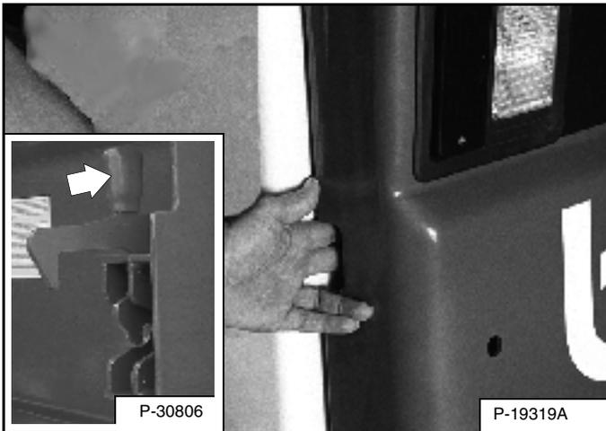
Reach into the slot in the rear door and pull the latch handle [Figure 136].
