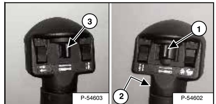
Press the auxiliary hydraulics button for *VARIABLE FLOW*.
