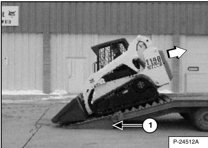
A loader with an empty bucket or no attachment must be loaded backward onto the transport vehicle [Figure 122].
