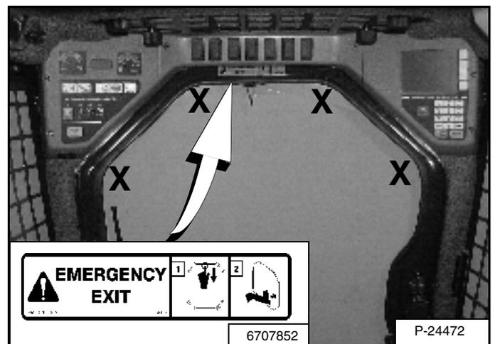
Push the window out with your foot [Figure 76] at any corner of the window.
