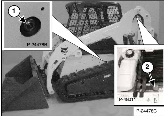
Check the fluid level in the sight gauge (1) [Figure 163].
