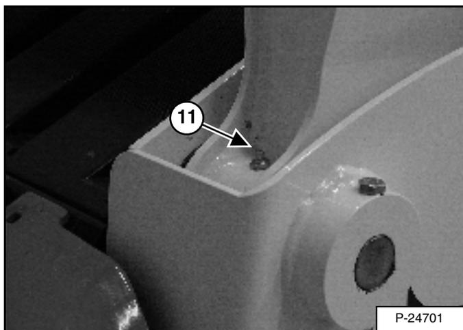
11. Lift Arm Link Pivot Pin (Both Sides) [Figure 189].
