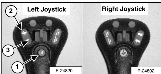
Press the button (1) [Figure 28] on the left joystick once to engage Speed Management.
