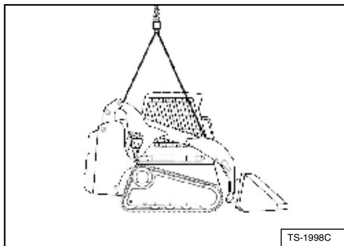
Attach cables or chains to lift eyes [Figure 121].
