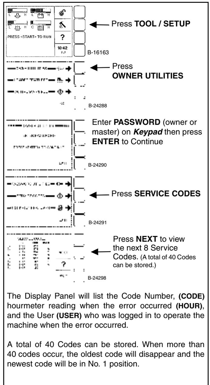
The Display Panel will list the Code Number, (CODE) hourmeter reading when the error occurred (HOUR), and the User (USER) who was logged in to operate the machine when the error occurred.
