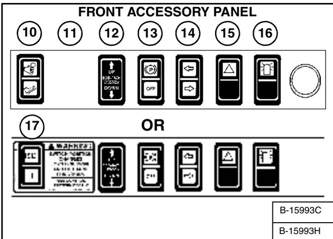
**NOTE:** Parking Brake (13) [Figure 12] is Standard on all loaders.
