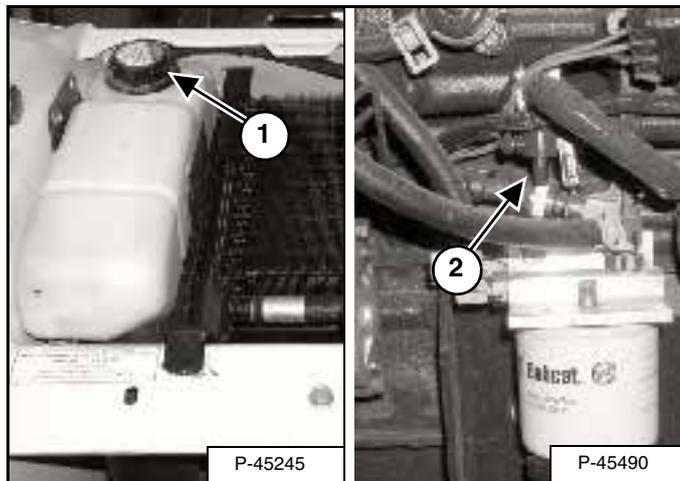
Remove the coolant fill cap (1) [Figure 155].
