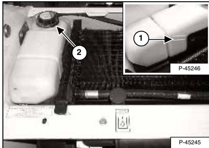
Check the coolant level on the side of the recovery tank (1) [Figure 154]. The level must be between the MIN and MAX marks.
