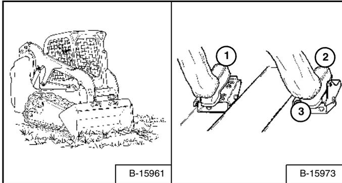
Lower the lift arms all the way (1) [Figure 103]. Put the cutting edge of the bucket on the ground (2) [Figure 103].
