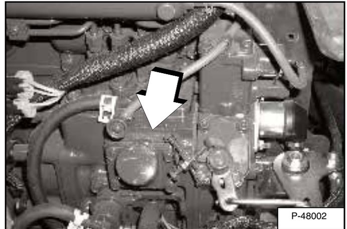
The engine serial number is located on the side of the engine [Figure 2] above the oil filter.
