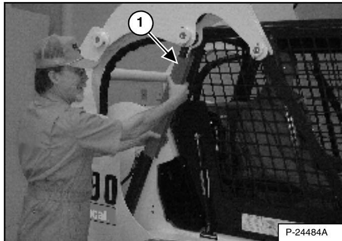
Have a second person install the lift arm support device (1) [Figure 128] over the rod of one of the lift cylinders.
