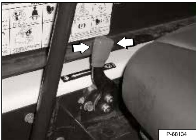
Set the engine speed control to the 1/2 speed position [Figure 58].
