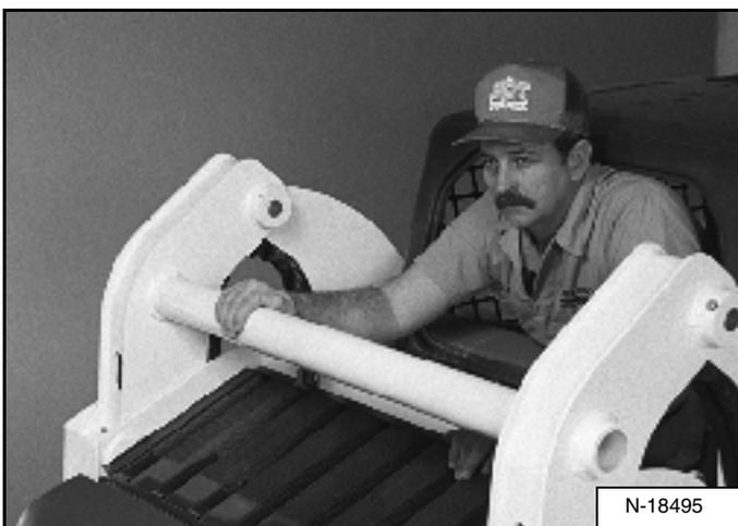
Exit through the rear of the operator cab [Figure 74].
