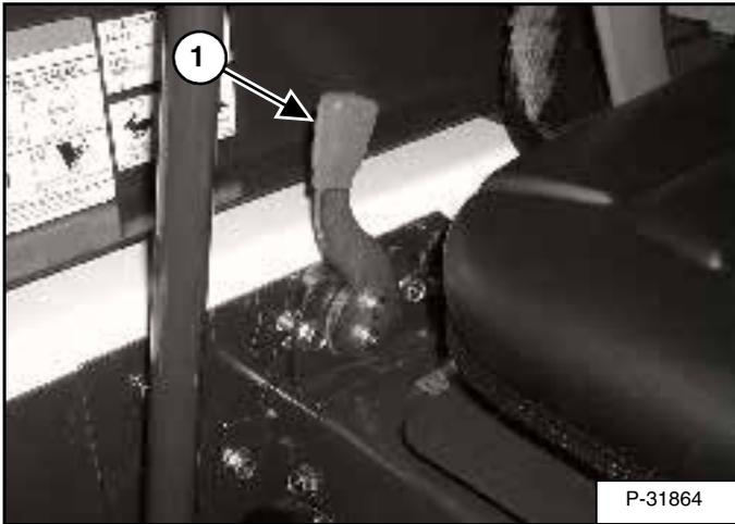
The speed control lever is at the right side of the operator's seat (1) [Figure 18].
