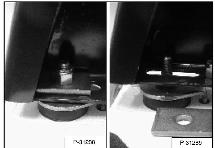
Install the plates and nuts [Figure 134] (both sides).
