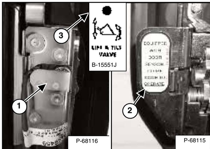
The cab door has a sensor (1) [Figure 135] installed which deactivates the lift and tilt valves when the door is open.
