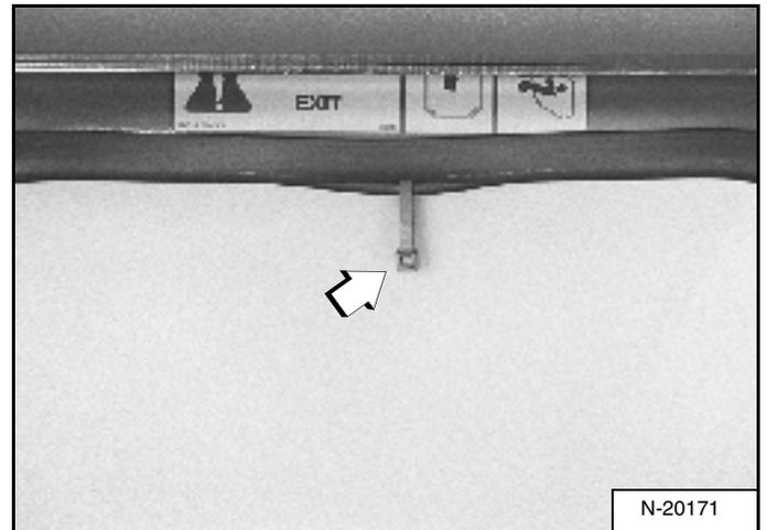
Pull the plastic loop at the top of the window in the front door to remove the rubber cord [Figure 75].
