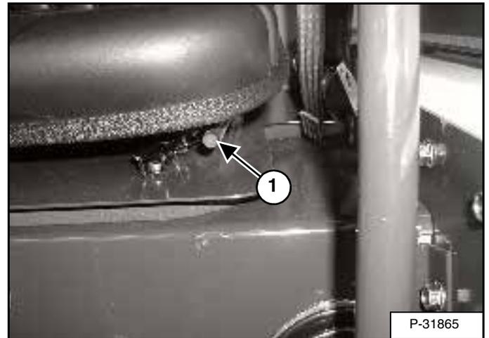
Release the seat lever (1) [Figure 53] and adjust the seat position for comfortable operation of the loader controls.
