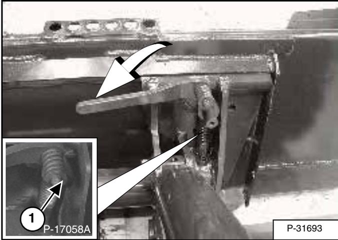
Push down on the Bob-Tach levers until they are fully engaged in the locked position (1) [Figure 81] (wedges fully extended).
