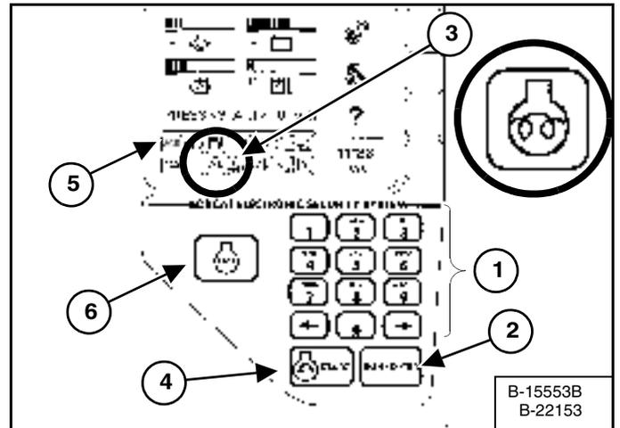
Use the numeric keypad (1) [Figure 63] to enter the password, then press the RUN/ENTER Button (2) [Figure 63].
