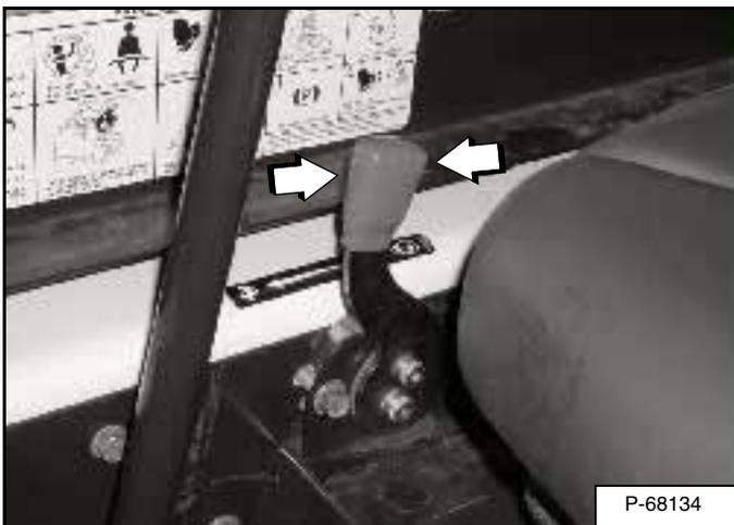
Set the engine speed control at the 1/2 speed position [Figure 58].
