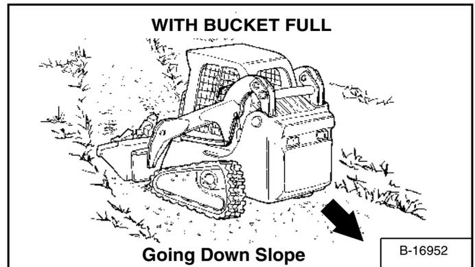
With a full bucket, go up or down the slope with the heavy end toward the top of the slope [Figure 95] and [Figure 96].
