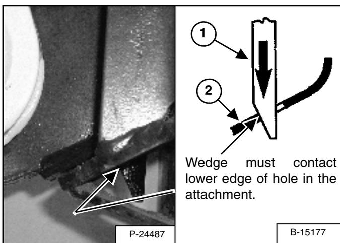
The wedges (1) must extend through the holes in the attachment mounting frame (2) [Figure 196].
