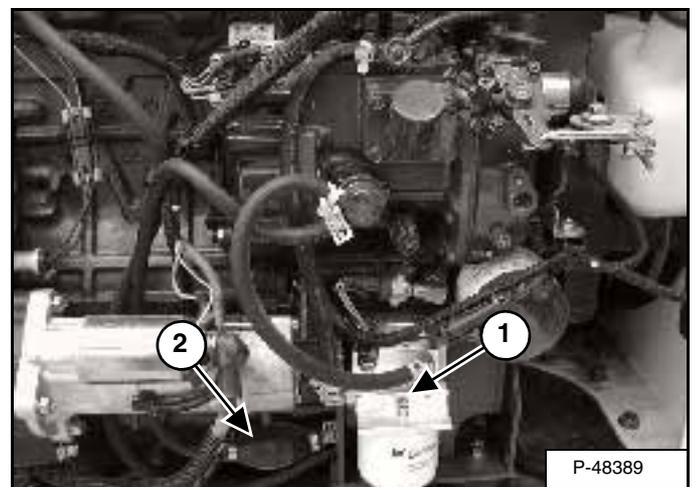
Open the vent (1) [Figure 151] on the fuel filter housing.
