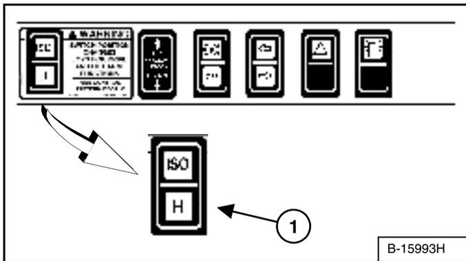
Select the 'H' control pattern by pressing the bottom of the switch (1) [Figure 22].
