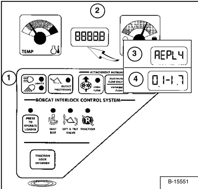
Press and hold the LIGHTS Button (1) [Figure 198] for two seconds to view SERVICE CODES in the HOURMETER / CODE DISPLAY (2). If more than one SERVICE CODE is present, the codes will scroll on the HOURMETER / CODE DISPLAY.
