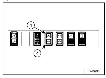
Press the top of the switch (Item 1) [Figure OI-41] to engage the parking brake. The traction drive system will be locked.
