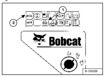
Turn the key switch to RUN [Figure OI-49]. The indicator lights on the right instrument panel [Figure OI-49] will come ON briefly and the Instrument Panel / monitoring system will do a self test.
