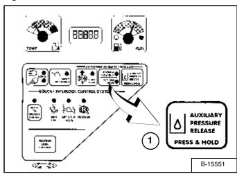
Press the AUXILIARY PRESSURE RELEASE Button (Item 1) [Figure OI-31]. Hold it for two seconds after the engine comes to a complete stop. The pressure will be released.
