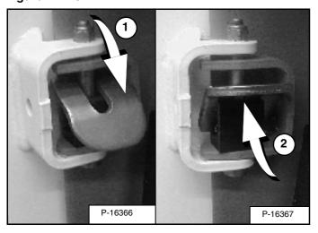
Move the door stop into the engaged position (Item 1) **[Figure PM-18]** to disengage the door stop and allow the door to close.
