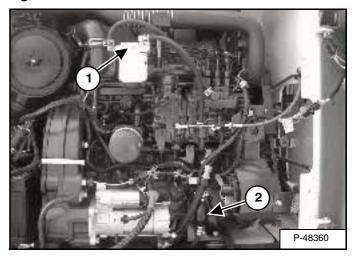
Open the vent (Item 1) [Figure PM-29] on the fuel filter housing.
