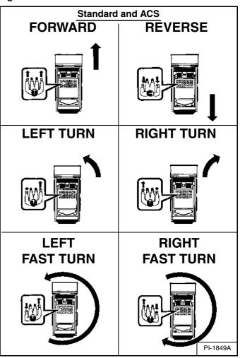
The steering levers control forward and reverse travel and turning the loader [Figure OI-15].
