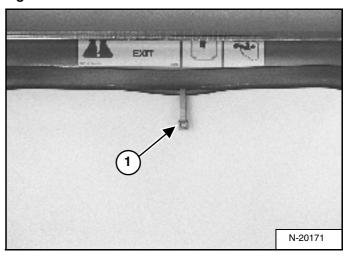
NOTE: When an Operator Cab Enclosure Kit is installed, the window of the front door can be used as an emergency exit [Figure PM-13].
