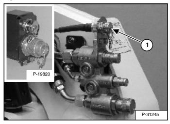
You will need the Dual-Connector (7-pin / 14-pin) kit (Inset) **[Figure Ol-39]** to operate early model attachments. The 7 pin connector is shown (Item 1) **[Figure Ol-39]**. See your Bobcat loader dealer.
