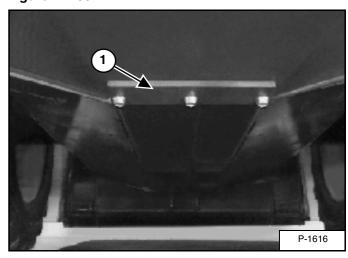
Remove the cover (Item 1) [Figure PM-55] which is installed over the drain plug at the bottom rear of the chaincase.
