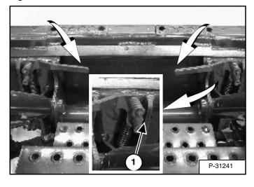
Push down on the Bob-Tach levers until they are fully engaged in the locked position (Item 1) [Figure OI-65] (wedges fully extended).
