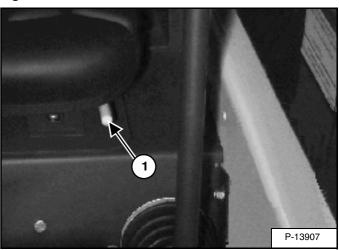
Release the seat lever (Item 1) [Figure OI-43] and adjust the seat position for comfortable operation of the loader controls.
