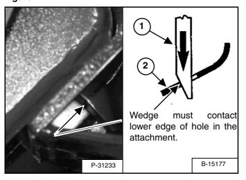
The wedges must extend through the holes in the attachment mounting frame (Item 1) [Figure PM-77].
