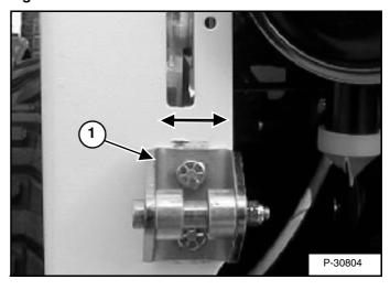
The door latch (Item 1) [Figure PM-19] can be adjusted side to side for alignment with the door latch mechanism.
