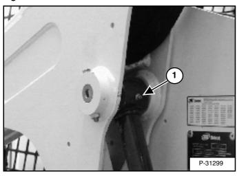
1. Rod End Lift Cylinder (Both Sides) [Figure PM-62].
