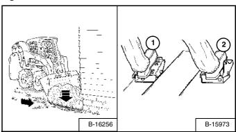
Lower the lift arms (Item 1) [Figure OI-83] and put the cutting edge of the bucket on the ground (Item 2) [Figure OI-83]. Drive forward to the edge of the hole to push the material into the hole.
