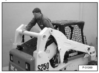
Exit through the rear of the operator cab [Figure PM-11].
