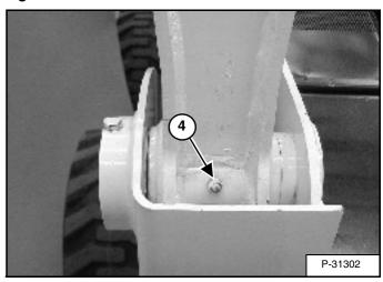
4. Lift Arm Link Pivot (Both Sides) [Figure PM-65].
