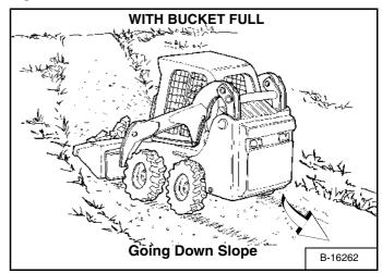
With a full bucket, go up or down the slope with the heavy end toward the top of the slope [Figure OI-74] and [Figure OI-75].
