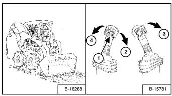
Press and hold the float button (Item 1) [Figure OI-87] while the lever is in neutral. While lowering the lift arms (Item 2) [Figure OI-87], release the float button.
