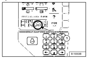
If the Fluid Pressure Icon (Item 1) [Figure OI-56] (Standard Panel) or [Figure OI-57] (Deluxe Panel) comes ON when operating the loader (cold), more warm up time is needed.
