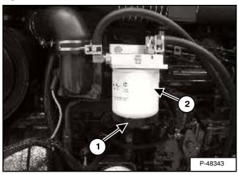
Loosen the drain (Item 1) [Figure PM-28] at the bottom of the filter element to remove water from the filter.
