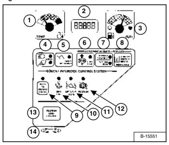
The left instrument panel is the same for both the Standard and Deluxe Instrument Panels [Figure OI-1].
