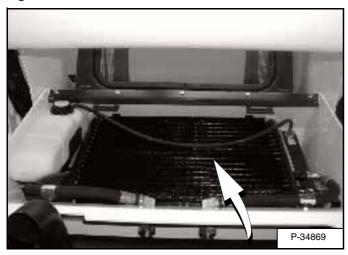
Use air pressure or water pressure to clean the top of the oil cooler [Figure PM-33].
