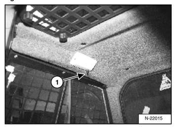
Push the button (Item 1) [Figure OI-8] to turn the light ON. Push the button again to turn OFF.
