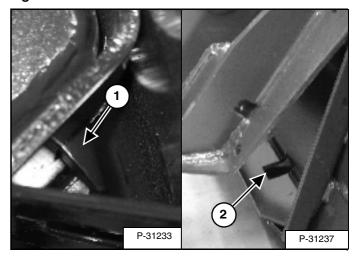
The wedges (Item 1) [Figure OI-66] must extend through the holes (Item 2) [Figure OI-66] in the mounting frame of the bucket (or other attachment), securely fastening the bucket to the Bob-Tach.
