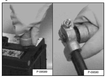
Always clean the battery terminals and cable ends when installing a new or used battery [Figure PM-42].
