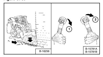
Lower the lift arms (Item 1) [Figure OI-89] and put the cutting edge of the bucket on the ground (Item 2) [Figure OI-89]. Drive forward to the edge of the hole to push the material into the hole.
