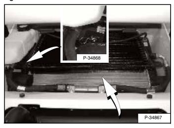
Raise the overflow tank slightly and remove the two fasteners (Inset) [Figure PM-34].
