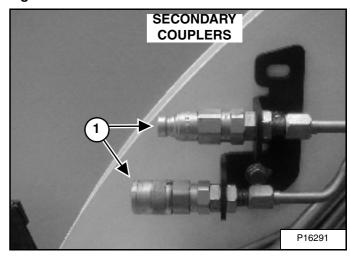
The secondary front auxiliary quick couplers (Item 1) [Figure OI-35] are available a Field Installed Accessory. These are used when there is a need for additional auxiliary hydraulics (EXAMPLE: Planer side shift).
