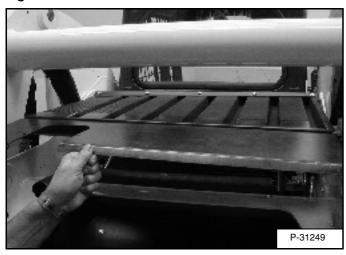
Lift and pull the rear grill and remove it from the loader [Figure PM-20].
