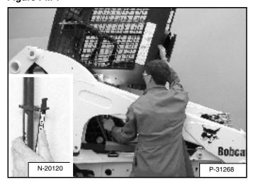
Pull down on the bottom of the operator cab until it stops at the latching mechanism [Figure PM-7].
