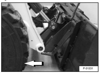
Move the loader backward, away from the bucket or attachment [Figure OI-73].
