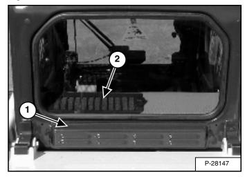
The <u>Fresh Air Filter</u> is located below the rear window of the cab (Item 1) [Figure PM-21].
