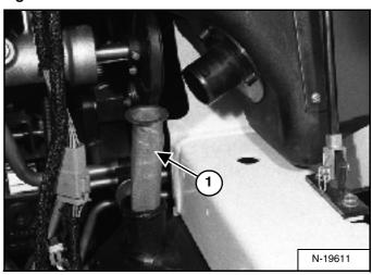
Remove the hydraulic fill screen (Item 1) [Figure PM-47]. Use air pressure to dry the screen.
