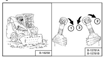
Lower the lift arms all the way (Item 1) [Figure OI-88]. Tilt the bucket forward (Item 2) [Figure OI-88] until the cutting edge of the bucket is on the ground.
