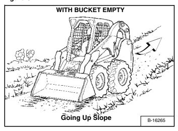
With an empty bucket, go down or up the slope with the heavy end toward the top of the slope [Figure OI-76] and [Figure OI-77].
