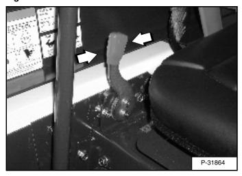
Set the engine speed control at the 1/2 speed position [Figure OI-52].
