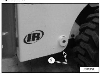
2. Base End Lift Cylinder (Both Sides) [Figure PM-63].
