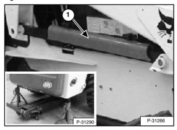
Put jackstands under the rear corners of the loader frame (Inset) [Figure PM-1].
