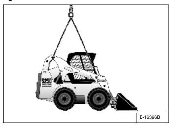
Attach cables or chains to lift eyes [Figure Ol-100].
