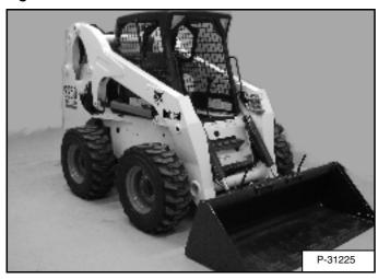
Lower the lift arms fully and put the attachment flat on the ground [Figure OI-96].
