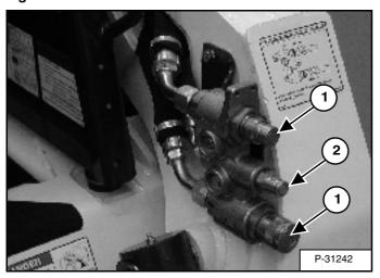
The High-Flow function provides additional flow to the system to operate an attachment which requires more hydraulic flow. (EXAMPLE: Planer.)
