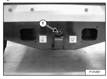
Remove the drain plug (Item 1) [Figure PM-54] from the front of the chaincase housing.
