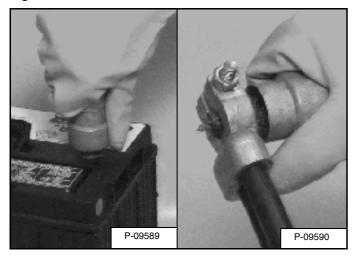
The battery cables must be clean and tight [Figure PM-37]. Check electrolyte level in the battery. Add distilled water as needed. Remove acid or corrosion from battery and cables with sodium bicarbonate (baking soda) and water solution.
