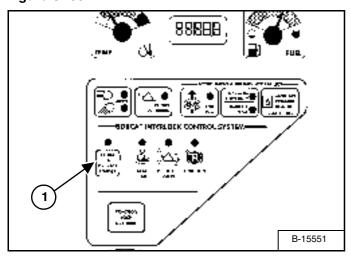
Press the PRESS TO OPERATE LOADER Button (Item 1) [Figure OI-55] to activate the BICS system and to perform hydraulic and loader functions. See also *Cold Temperature Starting* below.
