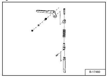
Inspect the mounting frame on the attachment and the Bob-Tach, linkages and wedges for excessive wear or damage [Figure PM-78]. Replace any parts that are damaged, bent, or missing. Keep all fasteners tight.
