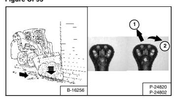
Lower the lift arms (Item 1) [Figure OI-95] and put the cutting edge of the bucket on the ground (Item 2) [Figure OI-95]. Drive forward to the edge of the hole to push the material into the hole.
