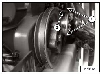
Loosen the mounting and adjustment bolts (Item 1) [Figure PM-61].
