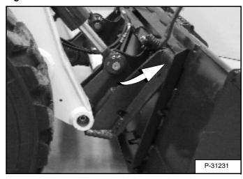
Drive the loader forward until the top edge of the Bob-Tach is completely under the top flange of the bucket **[Figure OI-70]** (or other attachment).
