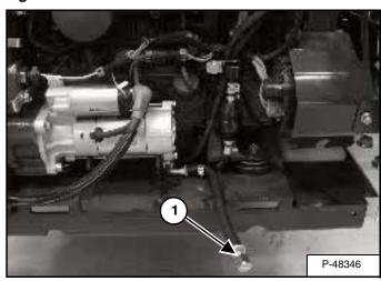
Remove the drain plug (Item 1) [Figure PM-32] and drain the oil into a container and recycle or dispose of used oil in an environmentally safe manner.
