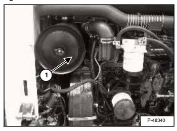
Remove the wing nut and remove the dust cover [Figure PM-24].
