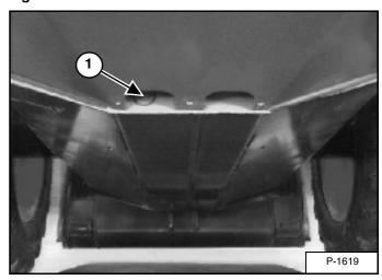
Remove the drain plug (Item 1) [Figure PM-56] and drain the oil into a container.
