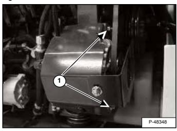
Loosen the alternator mounting and adjustment bolts (Item 1) [Figure PM-58].
