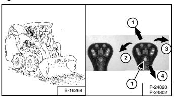
Press and hold the float button (Item 1) [Figure OI-93] while the joystick is in neutral. While lowering the lift arms (Item 2) [Figure OI-93], release the float button.
