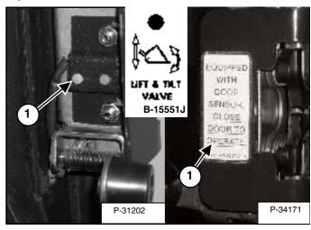
Later model cab doors\* have a sensor (Item 1) [Figure PM-9] installed which edactivates the lift and tilt valves when the door is open.
