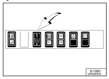
Push and hold the BOB-TACH "WEDGES UP" switch [Figure PM-76] until wedges are fully raised. Push and hold the BOB-TACH "WEDGES DOWN" switch [Figure PM-76] until the wedges are fully down.
