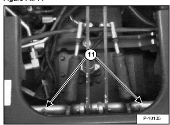
11. 250 Hours: Steering Lever Shaft (2) [Figure PM-71].
