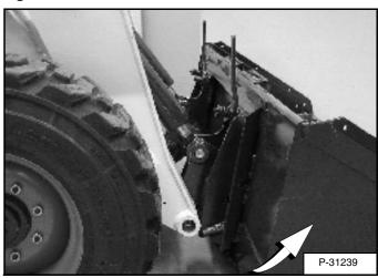
Tilt the Bob-Tach backward until the cutting edge of the bucket (or other attachment) is slightly off the ground [Figure OI-64].
