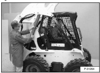
Have a second person install the lift arm support device over the rod of one of the lift cylinders [Figure PM-2].
