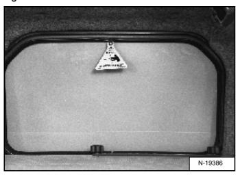
Pull on the tag [Figure PM-10] on the top of the rear window to remove the rubber cord.
