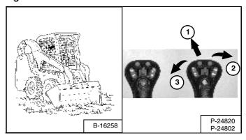
Lower the lift arms all the way (Item 1) [Figure OI-94]. Put the cutting edge of the bucket on the ground (Item 2) [Figure OI-94].
