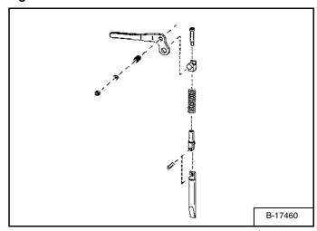
Inspect the mounting frame on the attachment and Bob-Tach, linkages and wedges for excessive wear or damage [Figure PM-75]. Replace any parts that are damaged, bent or missing. Keep all fasteners tight.
