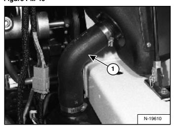
Remove the two hose clamps and remove the hose (Item 1) [Figure PM-46].
