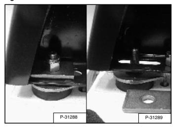
Install the plates and nuts (both sides) [Figure PM-8].
