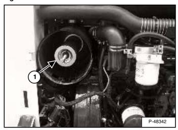
Remove the inner filter element (Item 1) [Figure PM-26].
