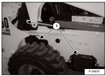
NOTE: All access covers (Item 1) [Figure PM-35] (both sides) must be in place to ensure correct air flow through the oil cooler which will ensure cooling for engine and hydraulic system.
