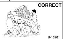
Use the correct procedure to lift of lower operator cab.
