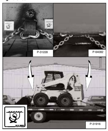
Use the following procedure to fasten the Bobcat loader to the transport vehicle to prevent the loader from moving during sudden stops or when going up or down slopes [Figure OI-98].
