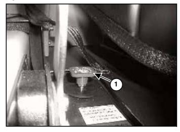
The lift arm by-pass control (Item 1) [Figure OI-9] is used to lower the lift arms if the lift arms cannot be lowered during normal operations.
