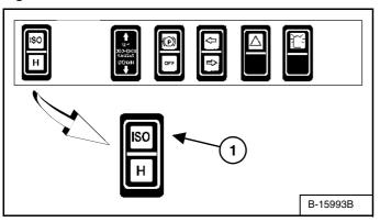
Select the 'ISO' control pattern by pressing the top of the switch (Item 1) [Figure OI-19].
