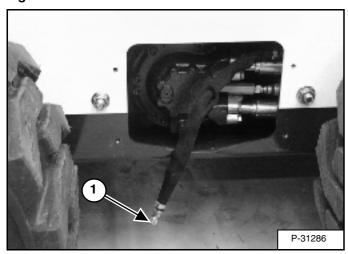
Pull the reservoir drain hose out the left motor cover hole. Remove the plug (Item 1) [Figure PM-49] and drain the fluid into a container.
