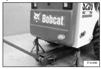
Install jackstands under the rear of the loader frame [Figure PM-4].
