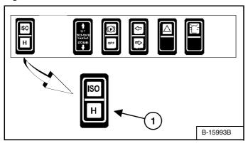
Select the 'H' control pattern by pressing the bottom of the switch (Item 1) [Figure Ol-16].
