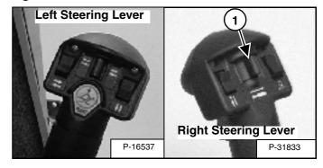
Push switch (Item 1) [Figure OI-36] to the right or left to change fluid flow direction. (EXAMPLE: Side shift on the Planer.)
