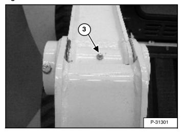
3. Lift Arm Pivot Pin (Both Sides) [Figure PM-64].
