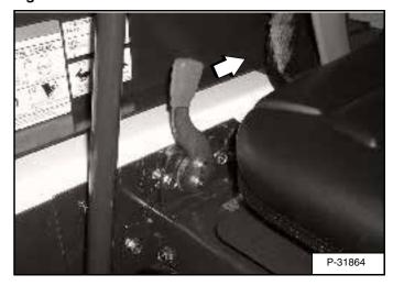
Pull the engine speed control fully backward [Figure OI-58] to decrease the engine speed.
