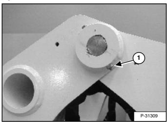
All lift arm and cylinder pivots have a large pin held in position with a retainer bolt and lock nut (Item 1) [Figure PM-72].
