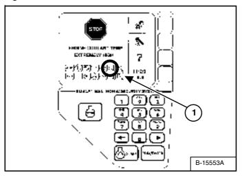
After the engine is running, frequently monitor the right instrument panel [Figure OI-59] (Standard Panel) and [Figure OI-60] (Deluxe Panel) for error conditions.
