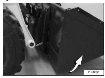
Tilt the Bob-Tach backward until the cutting edge of the bucket (or other attachment) is slightly off the ground [Figure OI-71].
