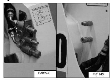
To Connect: Remove dirt or debris from the surface of both the male and female couplers, and from the outside diameter of the male coupler. Visually check the couplers for corroding, cracking, damage or excessive wear. If any of these conditions exist, the coupler(s) [Figure OI-30] must be replaced.
