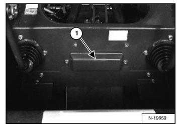
The electrical system is protected from overload by fuses and relays under the fuse panel cover (Item 1) [Figure PM-38]. A decal is inside the cover to show location and amp ratings.
