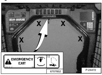
Push the window out with your foot [Figure PM-13] at any corner (X) of the window.
