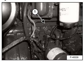
The engine serial number is located on the side of the engine (Item 1) [Figure 2] above the oil filter.
