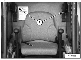
Use compressed air to clean any debris or dirt from the pivot parts (Item 1) **[Figure PM-15]**. Do not lubricate. Inspect all mounting hardware. The correct bolt torque is 35 Nm.
