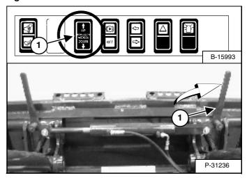
Push and hold the BOB-TACH "WEDGES UP" Switch (Front Accessory Panel) [Figure OI-72] until the wedges are fully raised.
