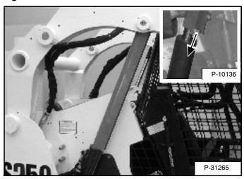
Lower the lift arms slowly until the lift arm support device is held between the lift arms and the lift cylinder [Figure PM-3]. The tabs of the lift arm support device must go under the cylinder (Inset) [Figure PM-3].
