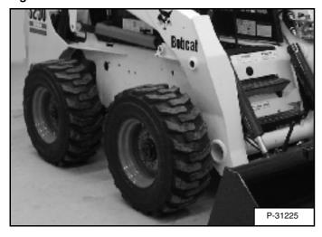
For the service interval to check the wheel nuts (See SERVICE SCHEDULE on Page PM-5). The correct torque is 142-156 Nm torque [Figure PM-52].
