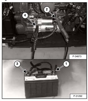
Connect the end of the first cable (Item 1) [Figure PM-40] to the positive (+) terminal of the booster battery. Connect the other end of the same cable (Item 2) [Figure PM-40] to the positive terminal on the loader starter.
