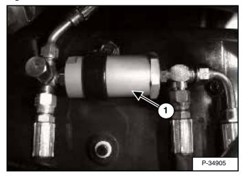
Disconnect the hoses from the hydrostatic motor case drain filter (Item 1) [Figure PM-50], remove the filter and discard.
