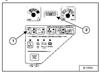
Press and hold the LIGHT Button (Item 1) [Figure PM-23] for two seconds.
