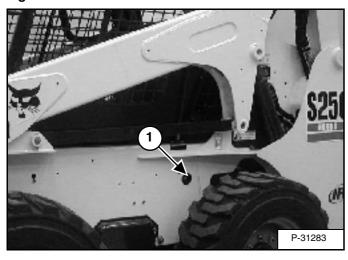
Check the fluid level in the sight gauge (Item 1) [Figure PM-43].
