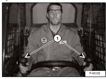
The steering levers (Item 1) [Figure OI-14] are on the left and right side in front of the seat.
