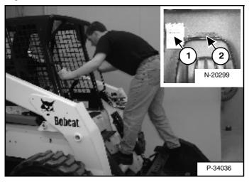
Use the bucket or attachment steps, grab handles and safety treads (on the loader lift arms and frame) to get on and off the loader [Figure OI-42]. Do not jump.
