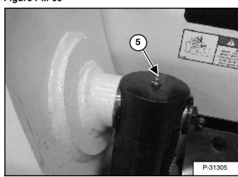
5. Base End Tilt Cylinder (Both Sides) [Figure PM-66].
