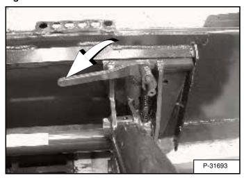
Move the Bob-Tach levers down to engage the wedges [Figure PM-73].
