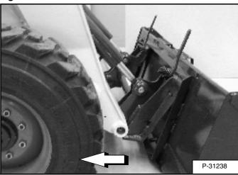
Move the loader backward, away from the bucket or attachment [Figure OI-68].
