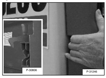
Reach into the slot in the rear door and pull the latch handle [Figure PM-17].
