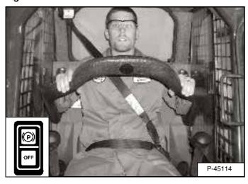
Lower the seat bar and engage the parking brake [Figure OI-47].
