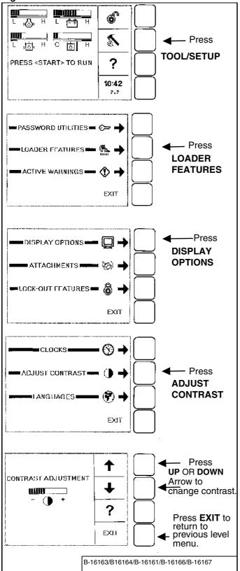
All new machines with Deluxe Instrumentation arrive at Bobcat Dealerships with the panel in locked mode. This means that a password must be used to start the engine **[Figure SA-3]**.
