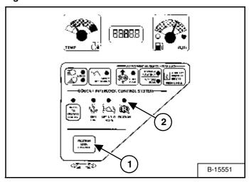
(Functions Only When The Seat Bar Is Raised And The Engine Is Running) There is a TRACTION LOCK OVERRIDE Button (Item 1) [Figure OI-10] on the left instrument panel which will allow you to use the steering levers to move the loader forward and backward when using the backhoe attachment or for loader service.
