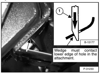
The wedges (Item 1) [Figure PM-74] must extend through the holes in the attachment mounting frame.
