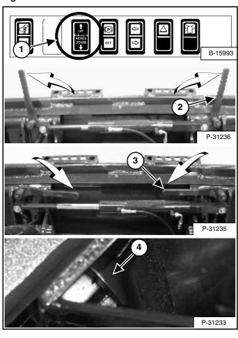
Push and hold BOB-TACH "WEDGES UP" switch (Item 1) [Figure OI-69] (Front Accessory Panel) until levers (Item 2) are in unlocked position (wedges fully raised).
