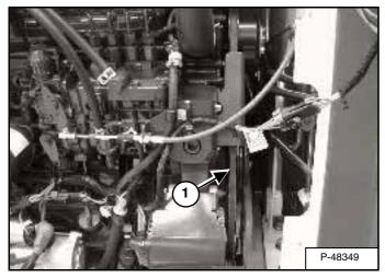
Move the alternator to tighten the belt. The tension is correct when there is 8,0 mm movement at the middle of the belt span (Item 1) [Figure PM-59] with 66 N of force.
