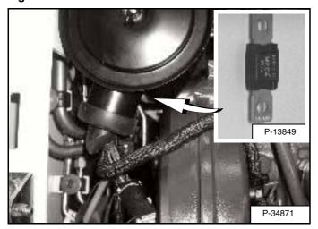
The loader has a 12 volt, negative ground alternator charging system. The electrical system is protected by fuses located in the cab on the steering control panel, and a 100 amp master fuse [Figure PM-36] in the engine compartment on the left side of the engine, under the air cleaner. The fuses will protect the electrical system when there is an electrical overload. The reason for the overload must be found before staring the engine again.
