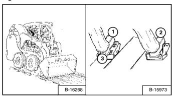
Put the lift arms in *float* position by pushing the pedal all the way forward (Item 1) **[Figure OI-81]** until the pedal is locked in the forward position.
