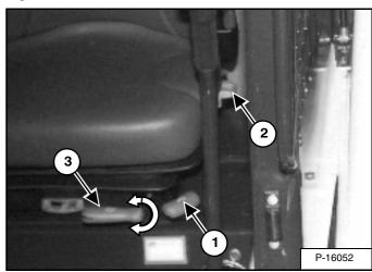
Suspension Seat - (Option & Loaders with 2-Speed) Release the lever (Item 1) [Figure OI-44] to adjust the seat distance from the levers and footrests.
