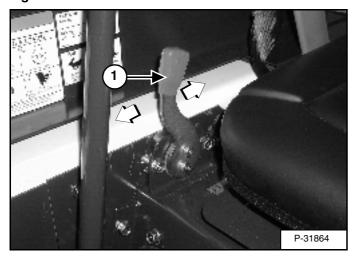
The speed control lever is at the right side of the operator's seat (Item 1) [Figure Ol-11].
