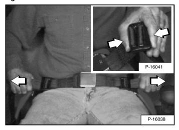
Squeeze both seat belt adjusters to release and lengthen each half of the seat belt [Figure OI-45].
