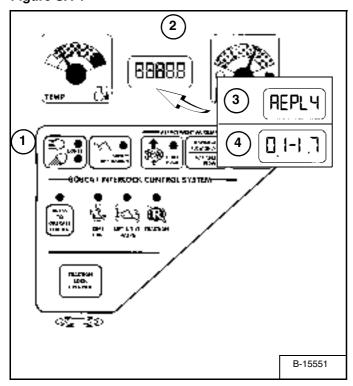
Press and hold the LIGHTS Button (Item 1) [Figure SA-1] for two seconds to view SERVICE CODES in the HOURMETER / CODE DISPLAY (Item 2). If more than one SERVICE CODE is present, the codes will scroll on the HOURMETER / CODE DISPLAY.
