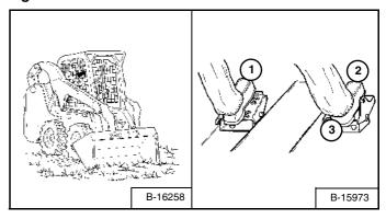
Lower the lift arms all the way (Item 1) [Figure OI-82]. Put the cutting edge of the bucket on the ground (Item 2) [Figure OI-82].
