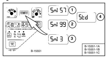
When the Inching Control is engaged, the machine will travel at 57% of Standard travel speed and the percentage (SnI 57) will appear in the display (Item 1) [Figure OI-13].
