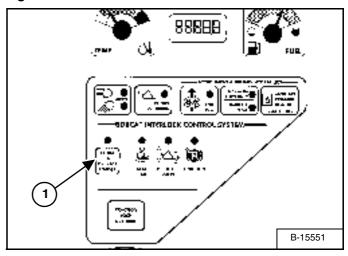
Press the PRESS TO OPERATE LOADER Button (Item 1) [Figure OI-51] to activate the BICS system and to perform hydraulic and loader functions. (See Cold Temperature Starting on Page OI-30.)
