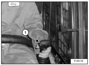
The joystick which controls drive and steering is on the left side in front of the seat (Item 1) [Figure OI-20].
