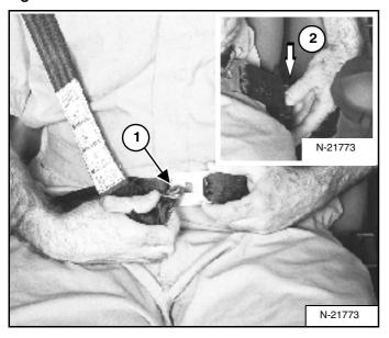
3-Point Restraint - (Option & Loaders with 2-Speed) Connect the shoulder belt to the lap belt (Item 1) [Figure OI-46]. Pull the lap belt across to the left side of the seat (Item 2) [Figure OI-46] and fasten.
