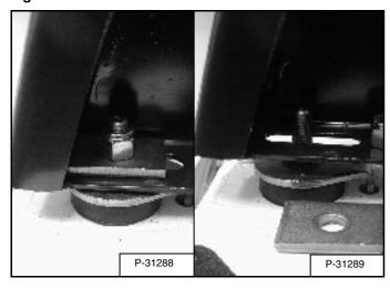
Remove the nuts and plates [Figure PM-5] (both sides) at the front corners of the cab.
