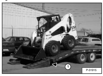
A loader with an empty bucket or no attachment must be loaded backward onto the transport vehicle [Figure OI-97].
