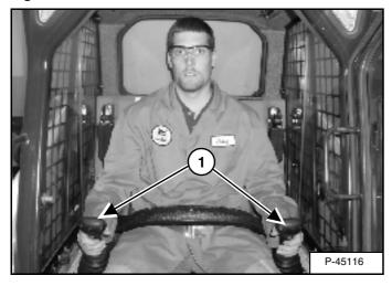
Both joysticks control drive and steering and are located on the right and left side in front of the seat (Item 1) [Figure OI-17].
