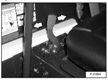
Set the engine speed control to the 1/2 speed position [Figure OI-48].
