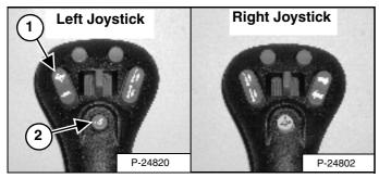
The two speed allows you to reduce cycle times when there is a long travel distance between the dig site and the dump site. You can also use the two speed when traveling from one job site to another at faster speeds.
