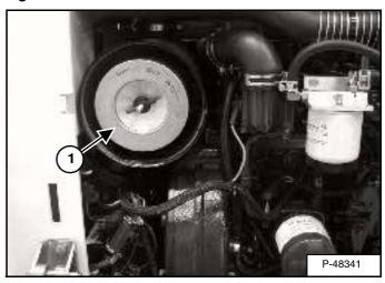
Remove the wing nut and pull the outer filter element (Item 1) [Figure PM-25] out and discard.
