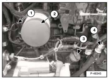
Open the rear door and remove the dipstick (Item 1) [Figure PM-30].
