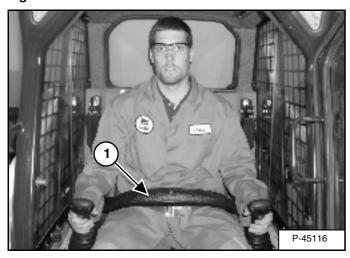
The seat bar restraint system has a pivoting seat bar with arm rests (Item 1) [Figure OI-22].
