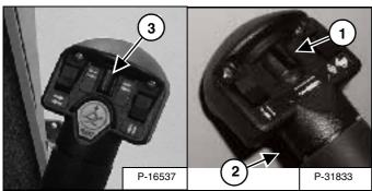
You can use additional switches (Items 1, 2, and 3) [Figure OI-40] on the right and left control handles for functions which control some attachments.
