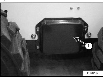
Remove the hydrostatic motor cover (Item 1) [Figure PM-48]. (Left Side)
