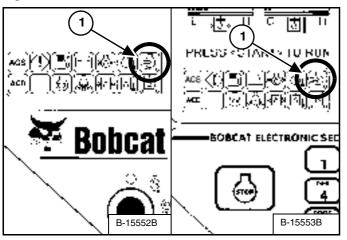
It is important to change the air filter element only when the Air Cleaner Icon in the right panel is ON (1) [Figure 124] and you hear three beeps from the alarm.
