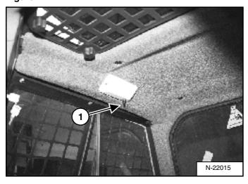
Push the button (1) **[Figure 12]** to turn the light ON. Push the button again to turn OFF.
