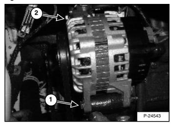
Loosen the alternator mounting bolt (1) and adjustment bolt (2) [Figure 138].
