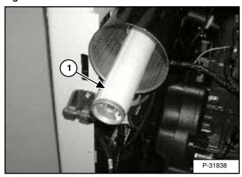
Remove the inner filter element (1) [Figure 128].
