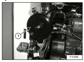
Remove the wing nut and remove the dust cover (1) [Figure 126].
