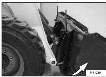
Tilt the Bob-Tach backward until the cutting edge of the bucket (or other attachment) is slightly off the ground [Figure 64].
