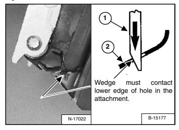
The wedges (1) **[Figure 170]** must extend through the holes in the attachment mounting frame.
