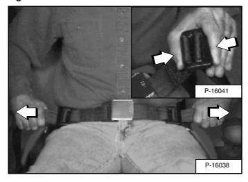
Squeeze both seat belt adjusters to release and lengthen each half of the seat belt [Figure 46].
