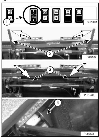
Push and hold BOB-TACH "WEDGES UP" switch (1) [Figure 69] (Front Accessory Panel) until levers (2) are in unlocked position (wedges fully raised).
