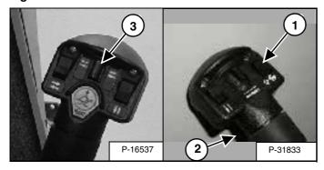
Press the auxiliary hydraulics button for VARIABLE FLOW (See also Auxiliary Hydraulics Button - VARIABLE FLOW on Page 18).
