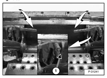
Push down on the Bob-Tach levers until they are fully engaged in the locked position (1) [Figure 65] (wedges fully extended).
