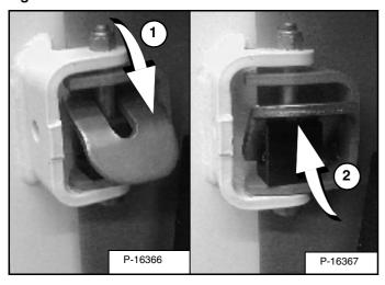
Move the door stop into the engaged position (1) **[Figure 120]** to hold the door open. Move to disengaged position (2) **[Figure 120]** to allow the door to close.
