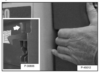
Reach into the slot in the rear door and pull the latch handle [Figure 119].
