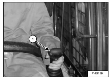
The joystick which controls drive and steering is on the left side in front of the seat (1) [Figure 25].
