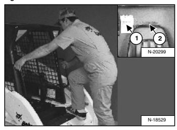
Use the bucket or attachment steps, grab handles and safety treads (on the loader lift arms and frame) to get on and off the loader [Figure 43]. Do not jump.
