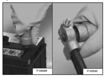
The battery cables must be clean and tight [Figure 140]. Check electrolyte level in the battery. Add distilled water as needed. Remove acid or corrosion from battery and cables with sodium bicarbonate (baking soda) and water solution.
