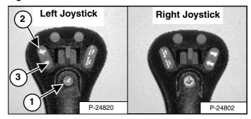
Press the button (1) **[Figure 16]** on the left joystick once to engage the Inching Control.
