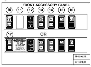
NOTE: Parking Brake (13) [Figure 11] is Standard on all loaders.
