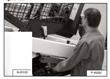
Pull down on the bottom of the operator cab until it stops at the latching mechanism [Figure 109].
