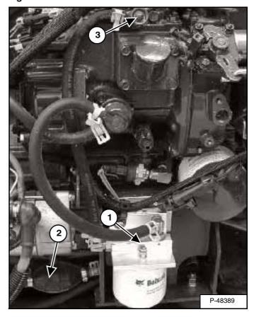
Open the vent (1) [Figure 131] on the fuel filter housing.
