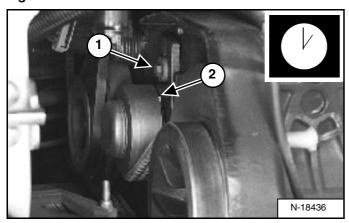
Loosen the bolt (1) [Figure 158] on the spring loaded drive idler.
