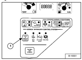
Press the PRESS TO OPERATE LOADER Button (1) [Figure 56] to activate the BICS system and to perform hydraulic and loader functions. (See Cold Temperature Starting on Page 27.)
