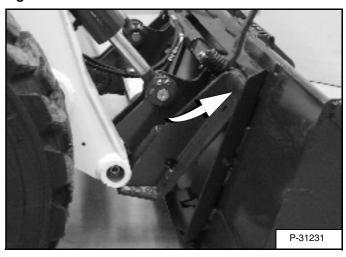
Drive the loader forward until the top edge of the Bob-Tach is completely under the top flange of the bucket **[Figure 70]** (or other attachment).
