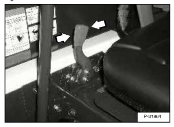
Set the engine speed control to the 1/2 speed position [Figure 49].
