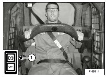
Lower the seat bar and engage the parking brake (1) [Figure 48].
