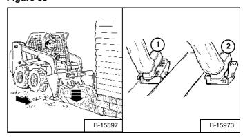
Lower the lift arms (1) [Figure 83] and put the cutting edge of the bucket on the ground (2) [Figure 83]. Drive forward to the edge of the hole to push the material into the hole.
