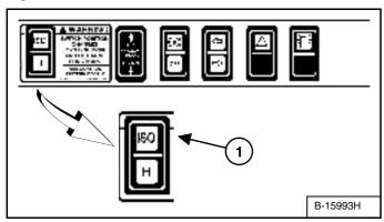
Select the 'ISO' control pattern by pressing the top of the switch (1) [Figure 24].
