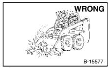
Never leave loader with engine running or with lift arms up. To park, engage parking brake and put attachment flat on the ground.
