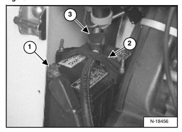
Remove the harness clamp from the positive cable.
