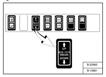
Push and hold the BOB-TACH "WEDGES UP" switch [Figure 172] until wedges are fully raised. Push and hold the BOB-TACH "WEDGES DOWN" switch [Figure 172] until the wedges are fully down.
