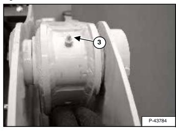
3. Lift Arm Pivot Pin (Both Sides) [Figure 163].
