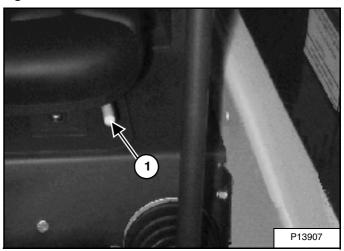
Release the seat lever (1) **[Figure 44]** and adjust the seat position for comfortable operation of the loader controls.
