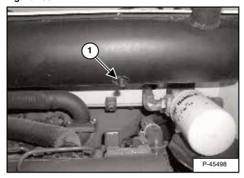
Remove the plug (1) [Figure 160] from the bottom of the muffler.
