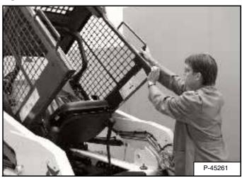
Lift on the grab handles and bottom of the operator cab [Figure 108] slowly until the cab is all the way up and the latching mechanism engages.
