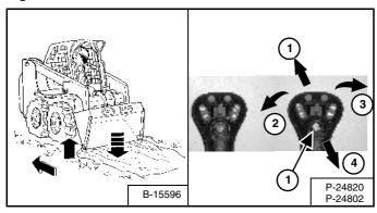
Press and hold the float button (1) [Figure 93] while the joystick is in neutral. While lowering the lift arms (2) [Figure 93], release the float button.
