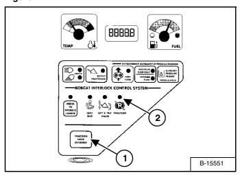
(Functions Only When The Seat Bar Is Raised And The Engine Is Running) There is a TRACTION LOCK OVERRIDE Button (1) [Figure 14] on the left instrument panel which will allow you to use the steering levers to move the loader forward and backward when using the backhoe attachment or for loader service.
