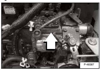
The engine serial number is located on the side of the engine [Figure 2].
