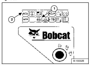
Turn the key switch to RUN [Figure 50]. The indicator lights on the right instrument panel [Figure 50] will come ON briefly and the Instrument Panel/monitoring system will do a self test.
