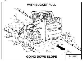
With a full bucket, go up or down the slope with the heavy end toward the top of the slope [Figure 74] and [Figure 75].
