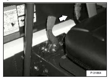
Pull the engine speed control fully backward [Figure 58] to decrease the engine speed.
