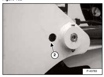
2. Base End Lift Cylinder (Both Sides) [Figure 162].
