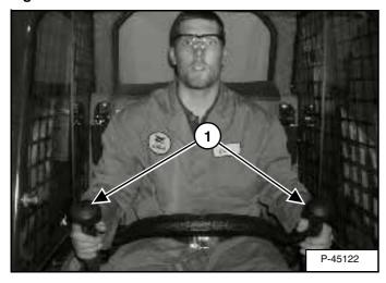
The steering levers (1) **[Figure 19]** are on the left and right side in front of the seat.
