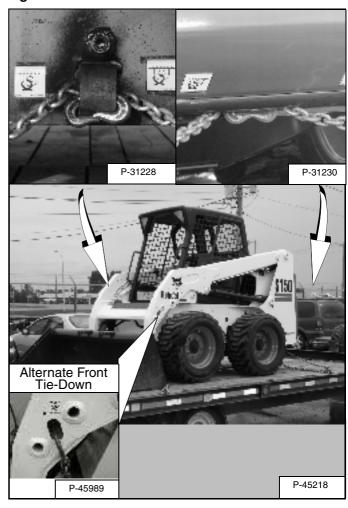
Use the following procedure to fasten the Bobcat Loader to the transport vehicle to prevent the loader from moving during sudden stops or when going up or down slopes [Figure 98].
