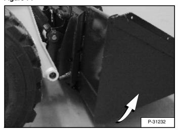
Tilt the Bob-Tach backward until the cutting edge of the bucket (or other attachment) is slightly off the ground [Figure 71].
