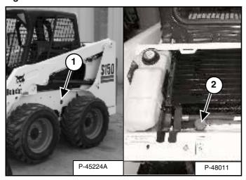
Check the fluid level in the sight gauge (1) [Figure 146].
