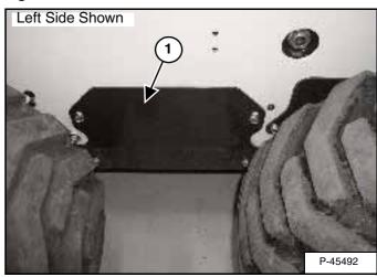
Remove both hydrostatic motor covers (1) [Figure 149].
