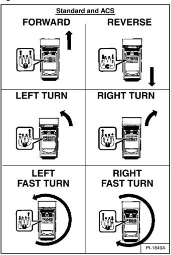
The steering levers control forward and reverse travel and turning the loader [Figure 20].
