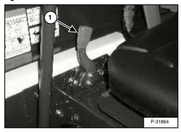
The speed control lever is at the right side of the operator's seat (1) [Figure 15].
