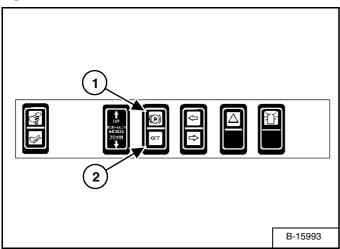
Press the top of the switch (1) [Figure 18] to engage the parking brake. The traction drive system will be locked.
