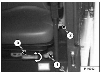
Suspension Seat - (Option) Release the lever (1) [Figure 45] to adjust the seat distance from the levers and footrests.
