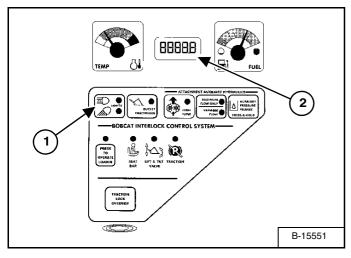
Press and hold the LIGHT Button (1) [Figure 125] for two seconds.
