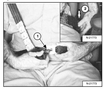
3-Point Restraint - (Option) Connect the shoulder belt to the lap belt (1) [Figure 47]. Pull the lap belt across to the left side of the seat (2) [Figure 47] and fasten.
