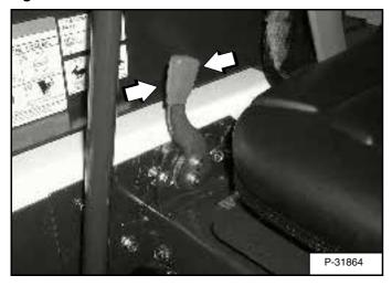
Set the engine speed control at the 1/2 speed position [Figure 53].
