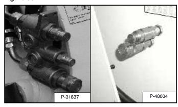
To Connect: Remove dirt or debris from the surface of both the male and female couplers, and from the outside diameter of the male coupler. Visually check the couplers for corroding, cracking, damage or excessive wear. If any of these conditions exist, the coupler(s) [Figure 36] must be replaced.
