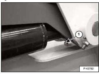
1. Rod End Lift Cylinder (Both Sides) [Figure 161].
