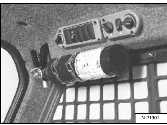
Know where fire extinguishers and first aid kits are located and how to use them. Fire extinguishers are available from your Bobcat dealer. The fire extinguisher can be installed in the location shown [Figure 4].
