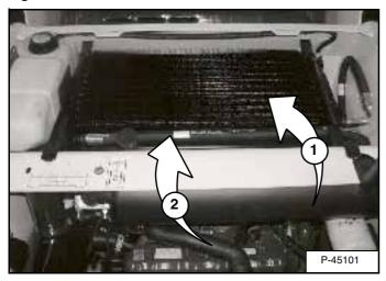
Use low air pressure or water pressure to clean the top of the oil cooler (1) [Figure 135].
