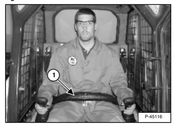
The seat bar restraint system has a pivoting seat bar with arm rests (1) [Figure 27].
