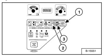
Press and hold the Auxiliary Pressure Release Button (1) [Figure 37] for 5 seconds.
