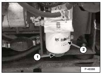
Loosen the drain (1) [Figure 130] at the bottom of the filter element to remove water from the filter.
