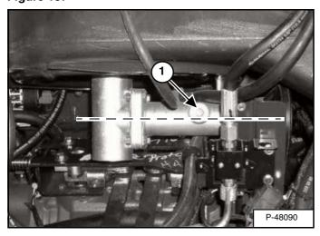
Remove the plug (1) [Figure 157]. Lubricant level must be at the bottom edge of the plug hole.
