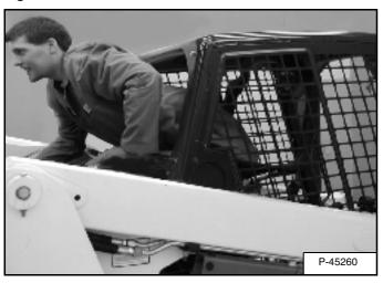
Exit through the rear of the operator cab [Figure 113].
