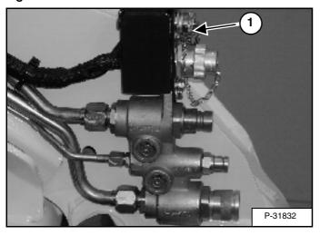
You will need the Dual-Connector (7-pin/14-pin) kit (1) [Figure 41] to operate early model attachments. See your Bobcat loader dealer.
