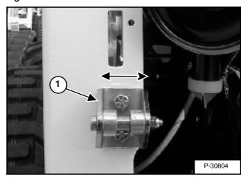
The door latch (1) [Figure 121] can be adjusted side to side for alignment with the door latch mechanism.
