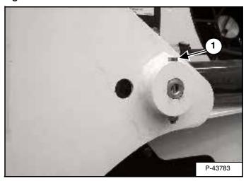
All lift arm and cylinder pivots have a large pin held in position with a retainer bolt and lock nut (1) [Figure 168].
