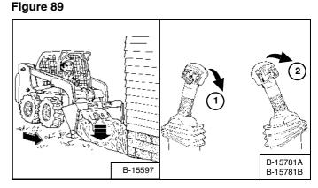
Lower the lift arms (1) [Figure 89] and put the cutting edge of the bucket on the ground (2) [Figure 89]. Drive forward to the edge of the hole to push the material into the hole.
