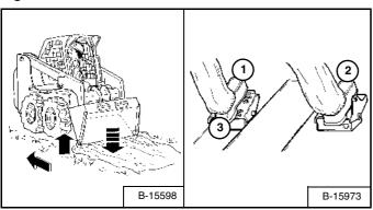
Put the lift arms in *float* position by pushing the pedal all the way forward (1) **[Figure 81]** until the pedal is locked in the forward position.
