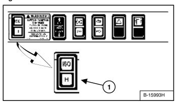
Select the 'H' control pattern by pressing the bottom of the switch (1) [Figure 21].
