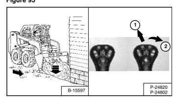
Lower the lift arms (1) [Figure 95] and put the cutting edge of the bucket on the ground (2) [Figure 95]. Drive forward to the edge of the hole to push the material into the hole.
