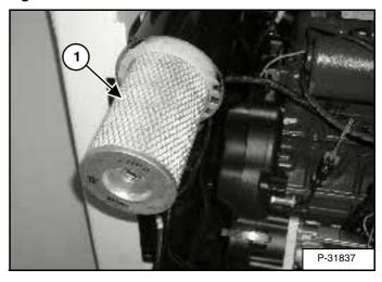
Remove the wing nut and pull the outer filter element (1) [Figure 127] out and discard.
