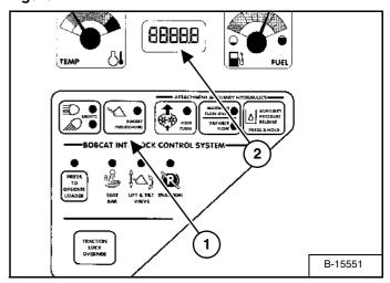
Press BUCKET POSITIONING button (1) **[Figure 42]** to engage the bucket position function. (The light will be on.) Press again to disengage.
