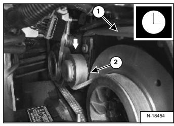
Push the idler pulley against the belt, using a pry bar (1) [Figure 159]. The pointer will be at the 3 o'clock position (2) [Figure 159] when the idler pulley is against the stop (maximum movement).
