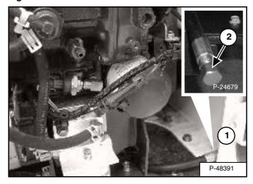
Open the rear door and remove the drain hose from its storage position (1) [Figure 133].
