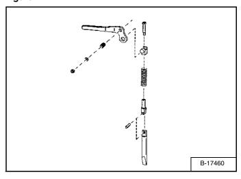
Inspect the mounting frame on the attachment and the Bob-Tach, linkages and wedges for excessive wear or damage [Figure 174]. Replace any parts that are damaged, bent, or missing. Keep all fasteners tight.
