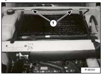
Lift and pull the rear grill and remove it from the loader [Figure 122].
