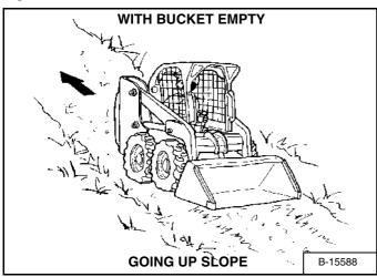
With an empty bucket, go down or up the slope with the heavy end toward the top of the slope [Figure 76] and [Figure 77].
