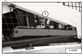
Lower the lift arm support device to the top of the lift cylinder. Hook the free end of the spring (1) [Figure 102] to the lift arm support device so there will be no interference with the support device engagement.
