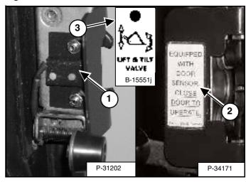
The cab door (option) has a sensor (1) [Figure 111] installed which deactivates the lift and tilt valves when the door is open.
