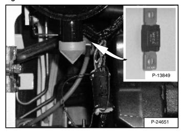
The loader has a 12 volt, negative ground alternator charging system. The electrical system is protected by fuses located in the cab on the steering control panel, and a 100 amp master fuse [Figure 139] in the engine compartment on the left side of the engine, under the air cleaner. The fuses will protect the electrical system when there is an electrical overload. The reason for the overload must be found before staring the engine again.
