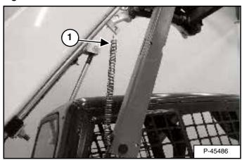
Connect the spring (1) **[Figure 104]** from the lift arm support device to the bracket below the lift arms.
