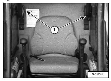
Use compressed air to clean any debris or dirt from the pivot parts (1) [Figure 117]. Do not lubricate. Inspect all mounting hardware. The correct bolt torque is 35 Nm.
