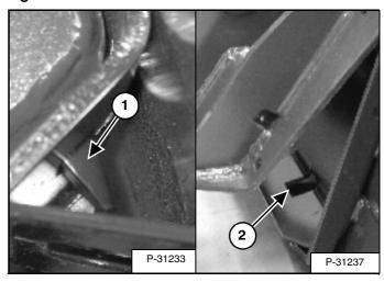
The wedges (1) [Figure 66] must extend through the holes (2) [Figure 66] in the mounting frame of the bucket (or other attachment), securely fastening the bucket to the Bob-Tach.
