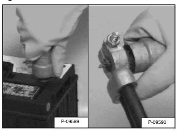
Always clean the battery terminals and cable ends when installing a new or used battery [Figure 145].
