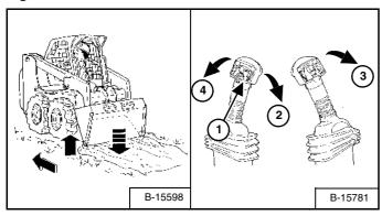
Press and hold the float button (1) [Figure 87] while the lever is in neutral. While lowering the lift arms (2) [Figure 87], release the float button.
