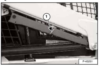
Raise the lift arms a small amount. The spring will lift the support device off the lift cylinder rod. Lower the lift arms. Stop the engine.
