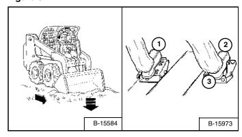
Lower the lift arms all the way (1) [Figure 82]. Put the cutting edge of the bucket on the ground (2) [Figure 82].
