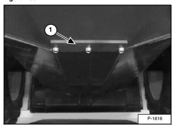
Remove the check plug (1) **[Figure 155]** from the front of the chaincase housing.
