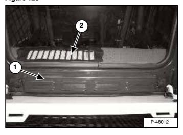
The <u>Fresh Air Filter</u> is located below the rear window of the cab (1) [Figure 123].
