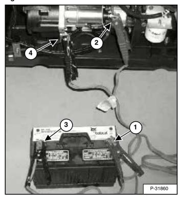
Connect the end of the first cable (1) [Figure 143] to the positive (+) terminal of the booster battery. Connect the other end of the same cable (2) [Figure 143] to the positive terminal on the loader starter.
