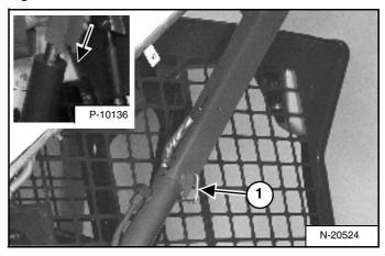
Raise the lift arms until the lift arm support device drops onto the lift cylinder rod (Inset) [Figure 103].
