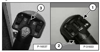
VARIABLE FLOW allows for slow-to-fast movement of auxiliary functions. If you move the auxiliary switch (1) [Figure 38] half-way, the auxiliary functions move at approximately one-half speed.
