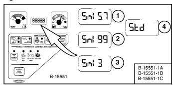
When the Inching Control is engaged, the machine will travel at 57% of Standard travel speed and the percentage [Snl 57] will appear in the display (1) [Figure 17].
