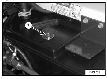
Raise the cab. Remove the plug from the top of the reservoir (1) [Figure 148] then pump the fluid out of the reservoir and into a container.
