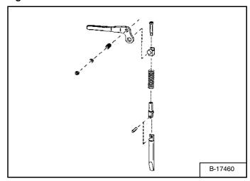
Inspect the mounting frame on the attachment and Bob-Tach, linkages and wedges for excessive wear or damage [Figure 171]. Replace any parts that are damaged, bent or missing. Keep all fasteners tight.
