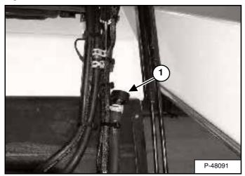
Remove and discard the hydraulic breather (1) **[Figure 151]**. Install new breather. (See SERVICE SCHEDULE on Page 53) for correct interval. Lower the cab. (See Lowering The Operator Cab on Page 57.)
