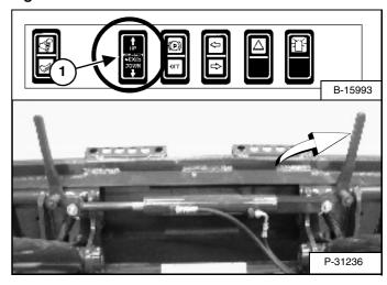
Push and hold the BOB-TACH "WEDGES UP" Switch (Front Accessory Panel) (1) [Figure 72] until the wedges are fully raised.
