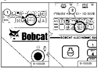
If the Fluid Pressure Icon (1) [Figure 57] (Standard Panel) or (2) [Figure 57] (Deluxe Panel) comes ON when operating the loader (cold), more warm up time is needed.
