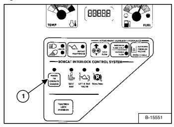
Press the PRESS TO OPERATE LOADER Button (1) [Figure 52] to activate the BICS<sup>™</sup> system and to perform hydraulic and loader functions. (See Cold Temperature Starting on Page 27.)
