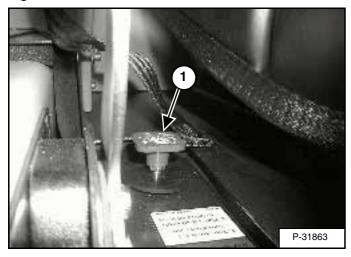
The lift arm by-pass control (1) [Figure 13] is used to lower the lift arms if the lift arms cannot be lowered during normal operations.
