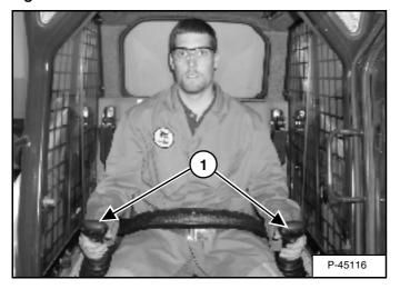
Both joysticks control drive and steering and are located on the right and left side in front of the seat (1) [Figure 22].
