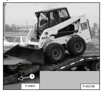
A loader with an empty bucket or no attachment must be loaded backward onto the transport vehicle [Figure 97].
