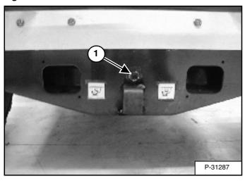
Remove the drain plug (1) [Figure 154] from the front of the chaincase housing.
