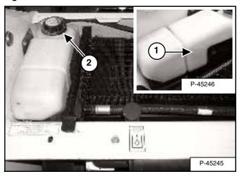
Check the coolant level on the side of the recovery tank (1) [Figure 136]. The level must be between the MIN and MAX marks.
