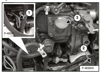
Open the rear door and remove the dipstick (1) [Figure 132].
