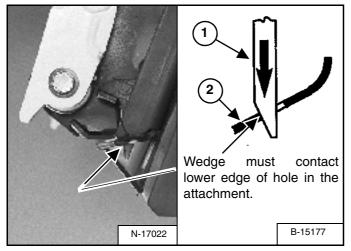
The wedges must extend through the holes in the attachment mounting frame (1) [Figure 173].
