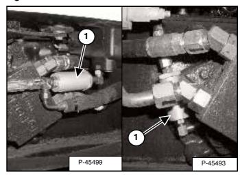
Remove the case drain filters (1) **[Figure 150]** near the hydrostatic motors. Disassemble the filter housings, thoroughly clean and install new filters. Reassemble and install the case drain filters. Install motor covers.
