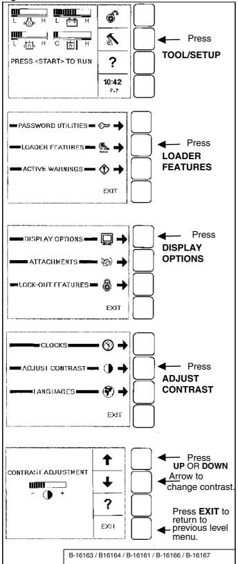
All new machines with Deluxe Instrumentation arrive at Bobcat Dealerships with the panel in locked mode. This means that a password must be used to start the engine [Figure 177].
