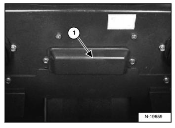
The electrical system is protected from overload by fuses and relays under the fuse panel cover (1) [Figure 141]. A decal is inside the cover to show location and amp ratings.
