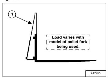
If a pallet fork attachment is used, the load center moves forward and reduces the Rated Operating Capacity.
