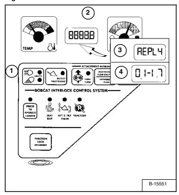
Press and hold the LIGHTS Button (1) [Figure 175] for two seconds to view SERVICE CODES in the HOURMETER / CODE DISPLAY (2). If more than one SERVICE CODE is present, the codes will scroll on the HOURMETER / CODE DISPLAY.
