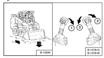
Lower the lift arms all the way (1) [Figure 88]. Tilt the bucket forward (2) [Figure 88] until the cutting edge of the bucket is on the ground.
