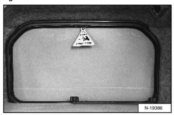
Pull on the tag [Figure 112] on the top of the rear window to remove the rubber cord.
