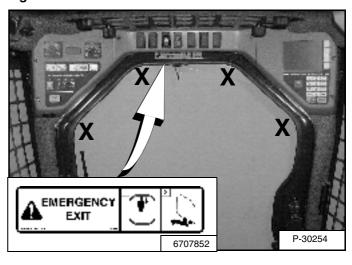
Push the window out with your foot [Figure 115] at any corner (X) of the window.
