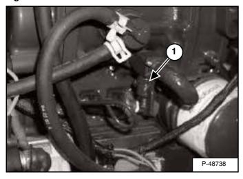
Connect a hose to the engine block drain (1) [Figure 137]. Open the drain valve and drain the coolant into a container.
