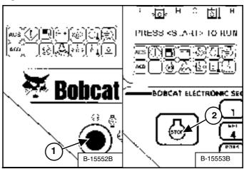
Turn the key switch to the STOP position (1) **[Figure 59]** (Standard Panel) or press the STOP Button (2) **[Figure 59]** (Deluxe Panel).
