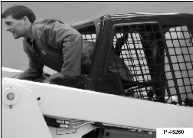
Exit through the rear of the operator cab [Figure 113].
