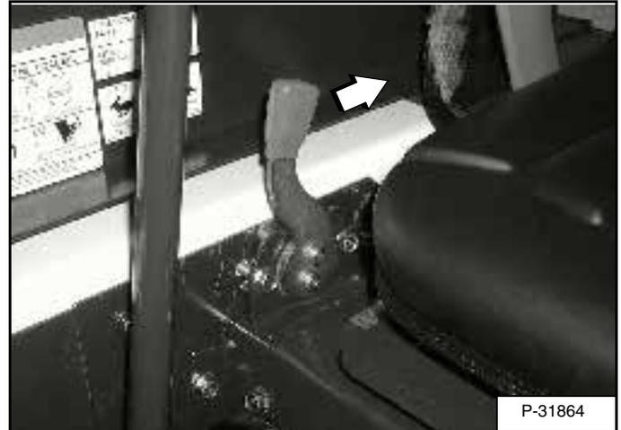
Pull the engine speed control fully backward [Figure 58] to decrease the engine speed.
