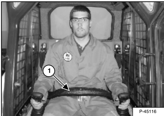
The seat bar restraint system has a pivoting seat bar with arm rests (1) [Figure 27].
