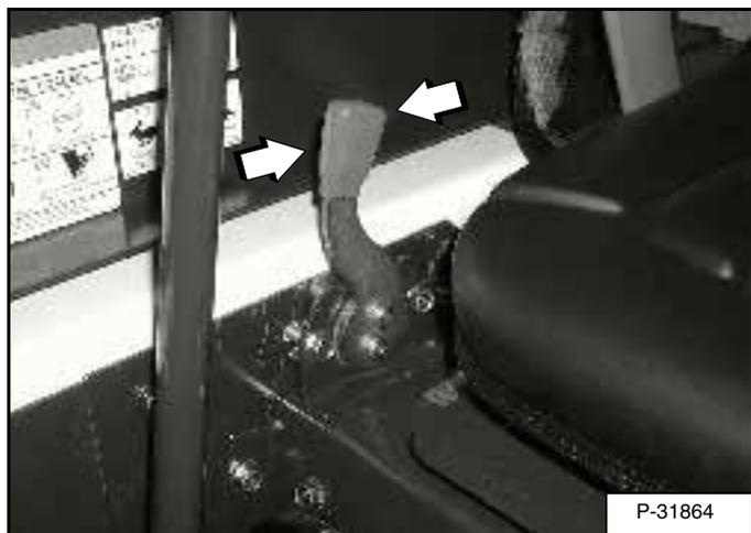
Set the engine speed control to the 1/2 speed position [Figure 49].
