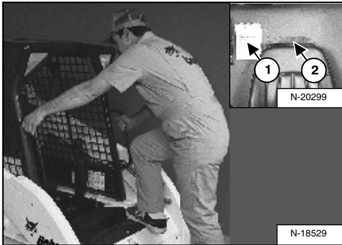
Use the bucket or attachment steps, grab handles and safety treads (on the loader lift arms and frame) to get on and off the loader [Figure 43]. Do not jump.
