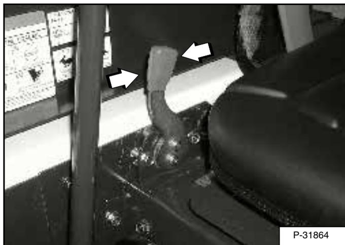
Set the engine speed control at the 1/2 speed position [Figure 53].
