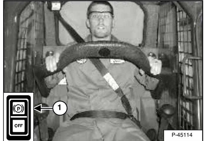
Lower the seat bar and engage the parking brake (1) [Figure 48].
