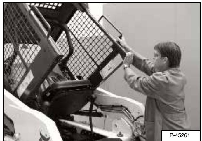
Lift on the grab handles and bottom of the operator cab [Figure 108] slowly until the cab is all the way up and the latching mechanism engages.
