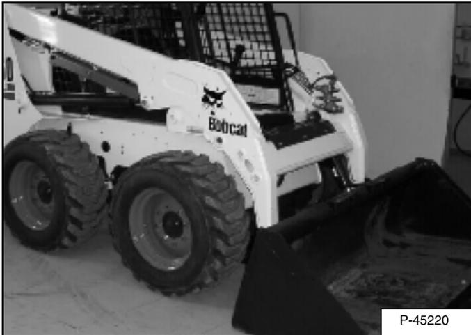
For the service interval to check the wheel nuts (See SERVICE SCHEDULE on Page 53). The correct torque is 142-156 Nm torque [Figure 152].
