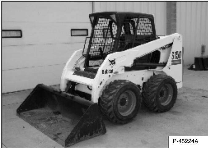
Lower the lift arms fully and put the attachment flat on the ground [Figure 96].
