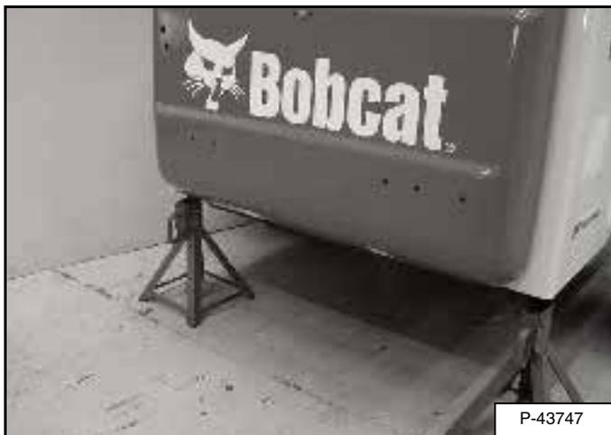
Install jackstands under the rear of the loader frame [Figure 106].
