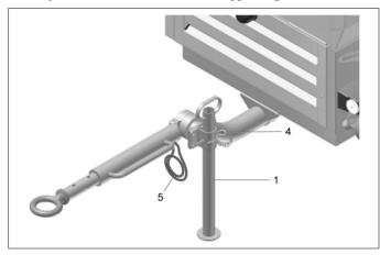
Adjustable towbar with jockey wheel and brakes:
