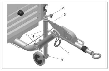
When parking a generator, secure support leg (1) or jockey wheel (2) to support the generator in a level position. Be sure that the jockey wheel (2) is blocked by the blocking pin (6).
