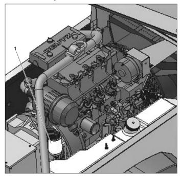
Replacing the filter element:
