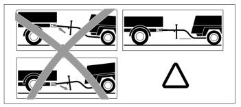
For both non-adjustable - and adjustable towbar, the towbar should be as level as possible and the generator and towing eye end in a level position.
