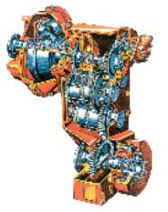
An electronically-controlled transmission provides the operator with a choice of fully automatic operation or manual powershift control. Six forward ratios and three reverses gears enable full use of the engine power in all ground conditions. Precise clutch engagement and smooth gearshift modulation result in extended driveline component life and reduced fatigue for the operator.
