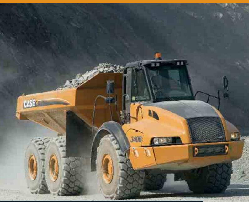
335B 330B 340B 327B 235 kW/315 hp 24 650 kg 260 kW/349 hp 28 160 kg 306 kW/410 hp 31 500 kg **Engine Horsepower** Payload Heaped capacity 14.5 m<sup>3</sup> 17.6 m<sup>3</sup> 20.0 m<sup>3</sup> 46 890 kg Total laden weight 50 730 kg 60 000 kg
