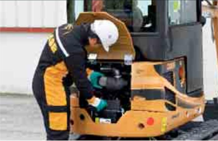
The new 11.3 kW Mitsubishi engine provides plenty of power for the series 2 machines. Centralised access, with all service points easily reached from beneath the engine canopy, reduces maintenance time and cuts service costs. The battery can be accessed from beneath the bonnet when necessary, further reducing downtime. All liquid checks can be carried out from ground level for maximum operator safety and rapid start-up each day.
