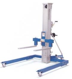
**Straddle Base:** Available in 1.5, 3 and 4.6 m (5, 10 and 15 ft) heights. The straddle base design is versatile and adjustable. It's easy to use and straddles loads from 56 cm to 1.27 m (22 to 50 in) wide. It's perfect for wide loads and narrow doorways. Easily handles pallets up to 1.2 m (48 in) wide. The straddle base models are built with the same durable construction used with the standard base models. Flat forks permit ground level loading.
