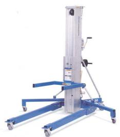
**Standard Base:** Available in 1.5, 3, 4.6, 6.1 and 7.6 m (5, 10, 15, 20 and 25 ft) heights. The field-proven design ensures durability and dependability. The welded steel base provides extra support. Stabilisers are standard on 6.1 and 7.6 m (20 and 25 ft) models. There are no loose parts.
