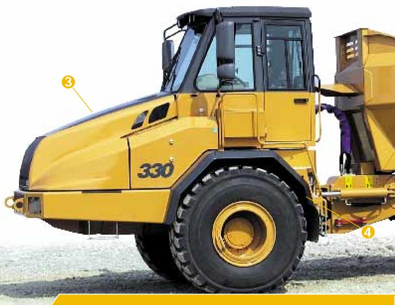
The widest **chassis** in the industry improves both traction and stability, in addition to allowing the use of inboard tipping cylinders for non ejector-bodied versions. Not only does this location protect the cylinders from damage, the improved lift geometry allows for a much gentler initial tipping action, thus reducing long term component wear.
