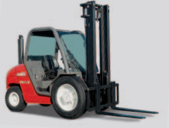
MSI 30 G with fixed reservoir (standard version with gas bottle).
